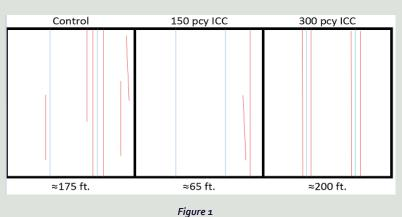
U.S. 80 Bridge deck layout with cracks (red) and support column locationss (blue)
