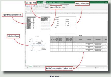
Figure 1 Wave force calculator interface
