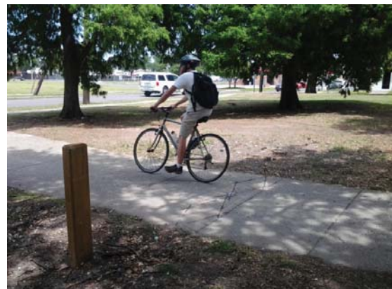
EcoMulti Infrared sensor and Loop Detector on the Jefferson Davis Parkway Trail, New Orleans Photo Credit: Tara Tolford (2014)
