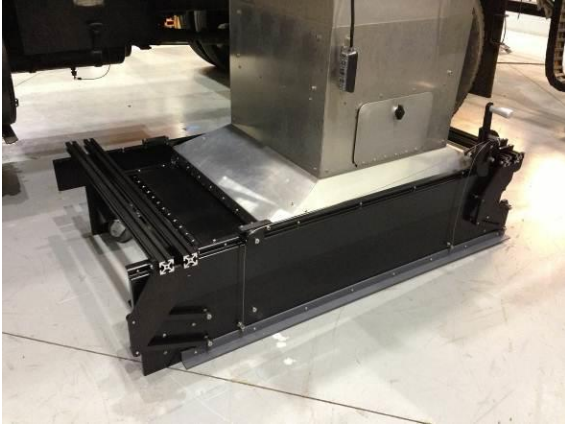
Figure 4: New shroud camera shroud including lift mechanism to stow while traveling
