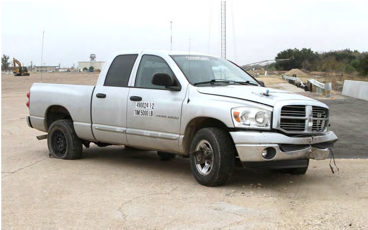
Figure 5.5. Vehicle after Test No. 490024-1-2.
