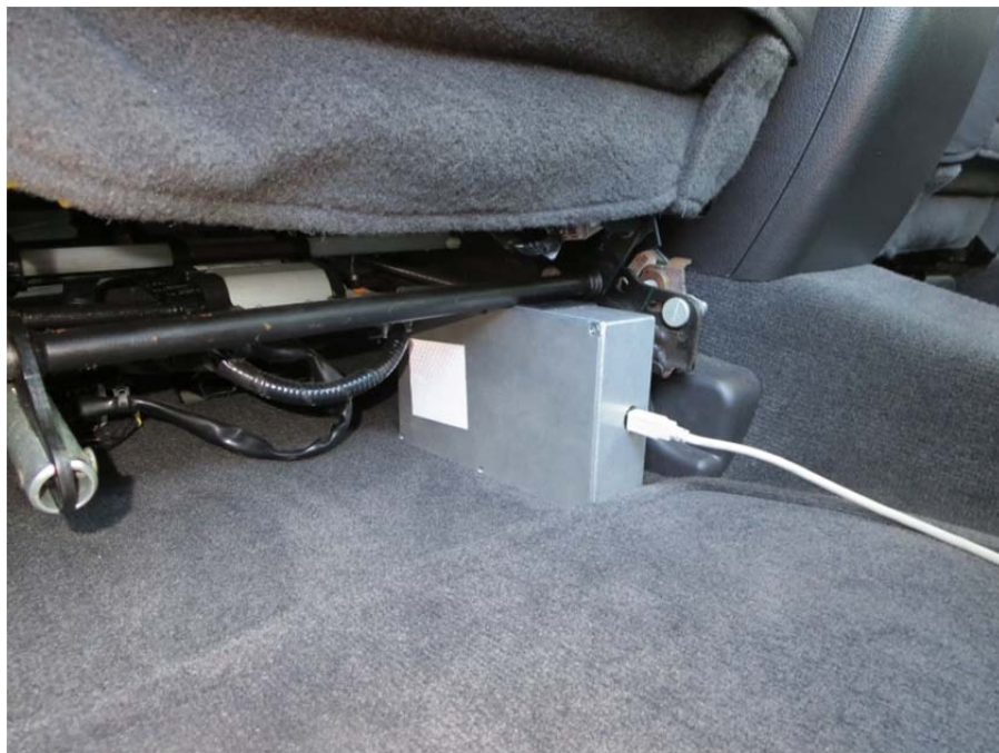
Figure 6. Accelerometer Monitoring Vibration of Drivers Seat.
