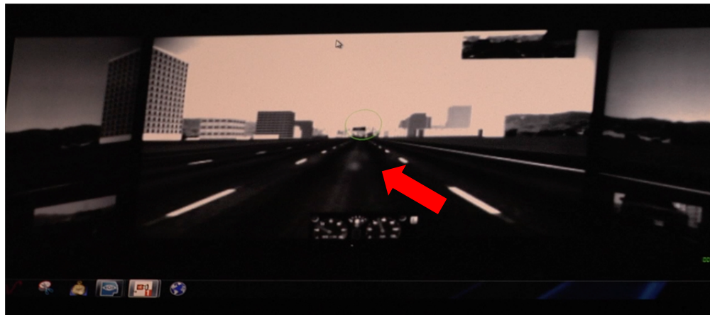
(b) Screen Capture of Eye Tracking Video (Green circle on the capture indicates where a driver looks)
