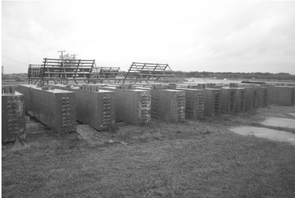
Figure 3-4. LSC Specimens Exposed to the Environment at the Riverside Campus.
