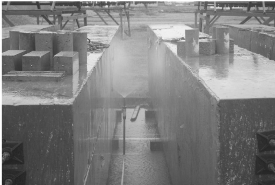
Figure 3-5. Sprinkler System between Two LSC Specimens.
