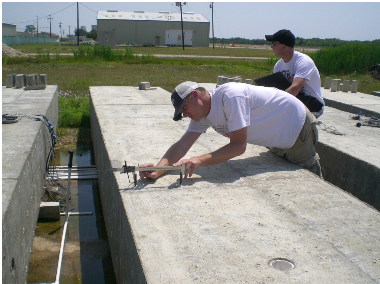
Figure 3-6. DEMEC Surface Strain Measurements.
