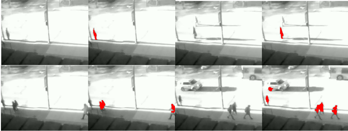
Figure 2: Sample results from blob detection and filtering. Detected pedestrians are marked in red.
