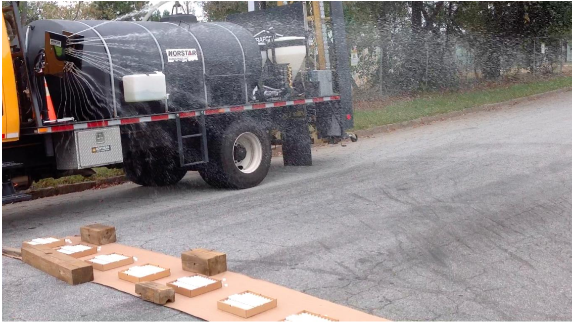
Picture 9. Evaluation of spray pattern uniformity using tracking dye and 20-mL glass vials.
