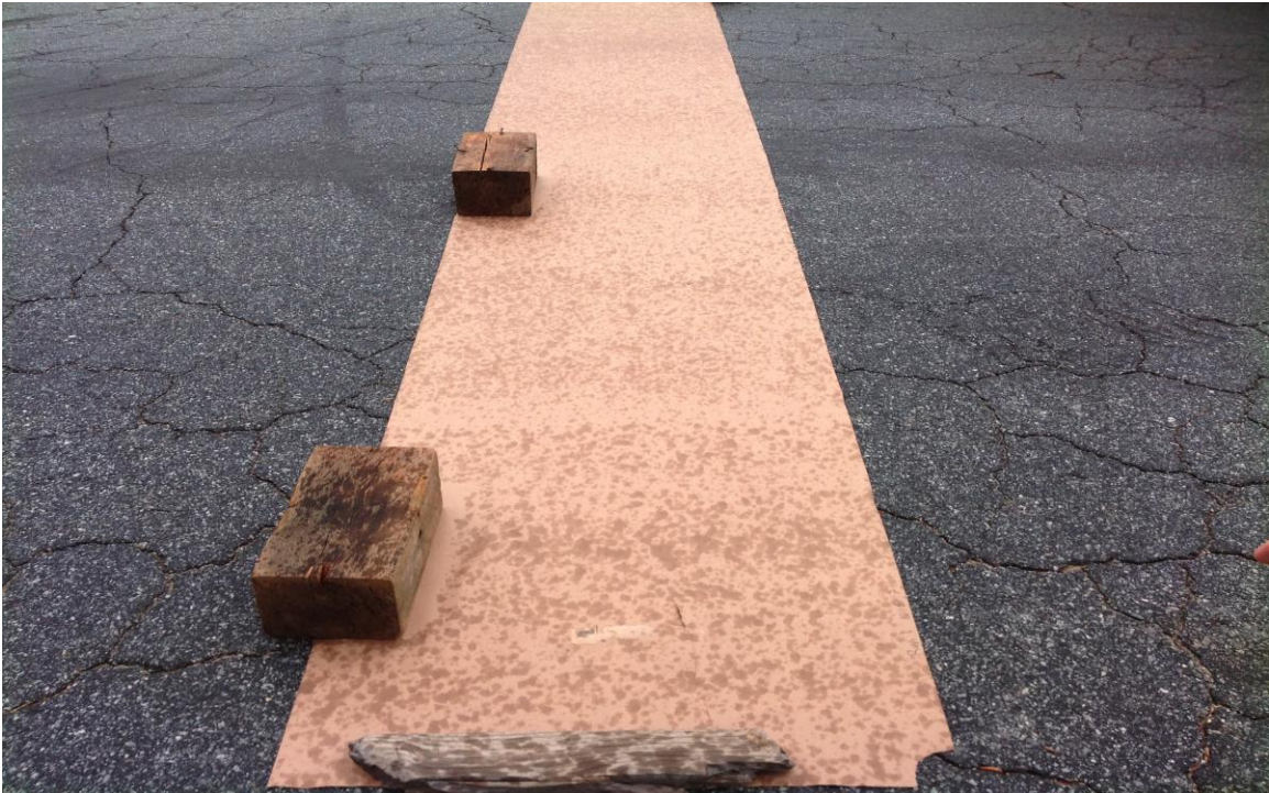
Picture 8. Spray droplets at various distances from the truck in calibration evaluations.
