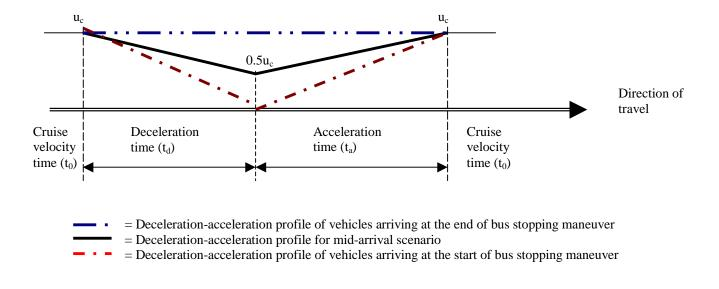
Figure 3 Schematic illustration of time-velocity relationship for estimation of mobile emissions
