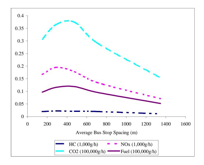
Figure 5 Graphical illustration of relationship between bus stop spacing and mobile emissions from Example 2.
