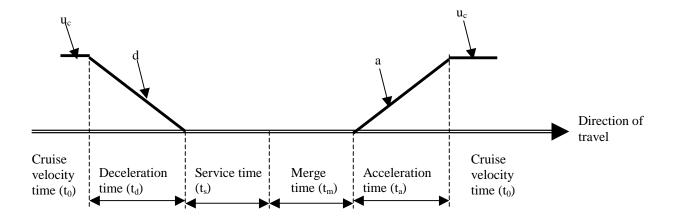
Figure 2 Schematic illustration of bus velocity profile at bus stops
