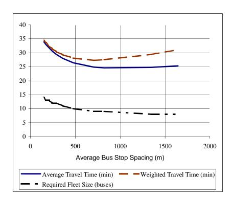
Figure 4 Relationship between bus stop spacing, travel time and fleet size requirement developed from Table 2.
