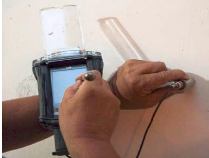
Figure 4: Impact-Echo Testing Equipment [31].
