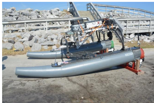
Figure 63: Left Image: From left to right, the PI, his two Ph.D. students, and two range technicians from GUSC. Right Image: The USV based bridge inspection system assembled for deployment at the Hwy 300 bridge test site.
