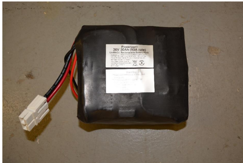
Figure 12: The LiNiMnCo 36 V, 30 Ah batteries.
