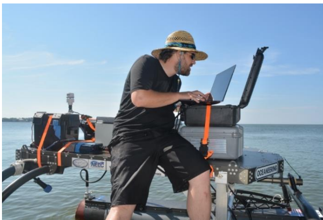
Figure 58: One of the FAU Ph.D. students aboard the USV16 verifying the sonar orientation and imaging settings.
