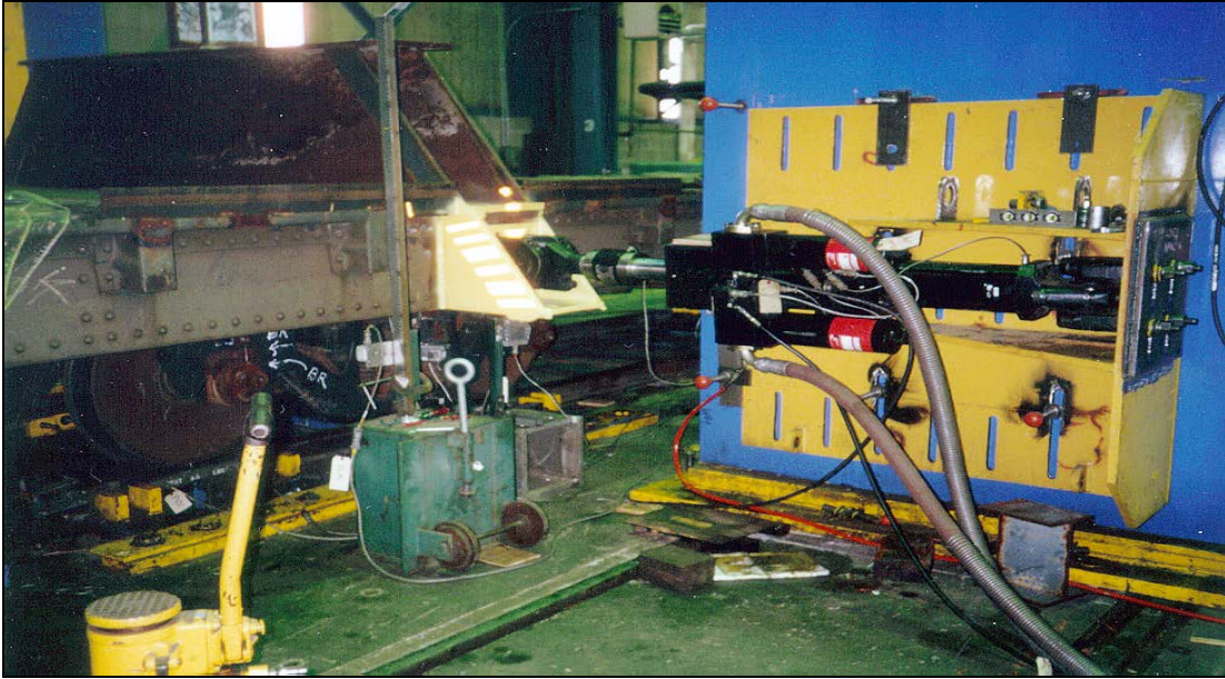
Figure 38. Mini-Shaker Unit Attached to Flat Car
