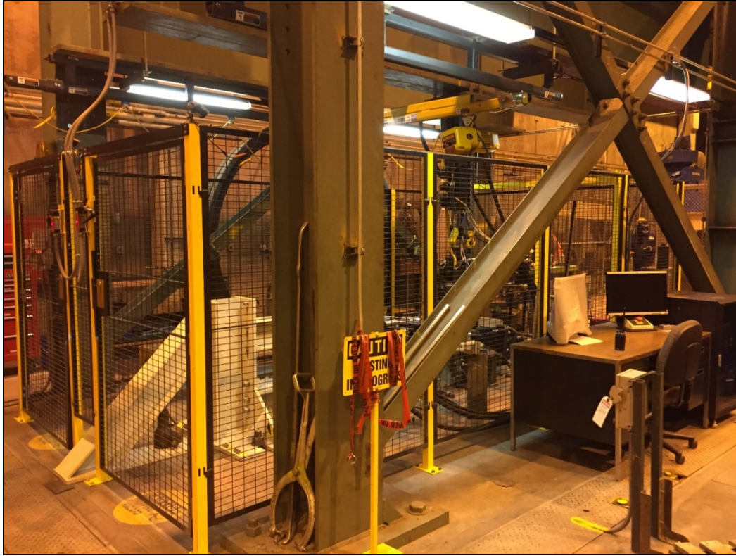
Figure 43. New Tie Wear Machine in the CTL
