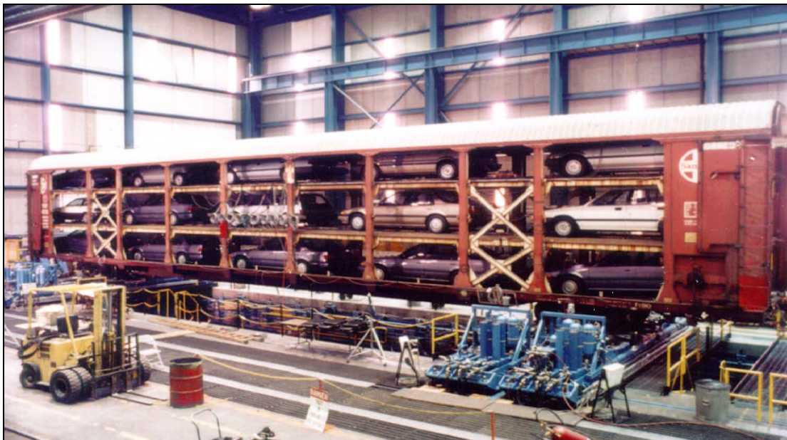
Figure 36. Vibration Test Unit, With Autorack Car in Test Mode
