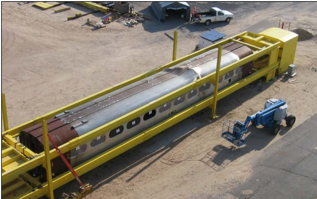
Figure 47. Squeeze Test Fixture
