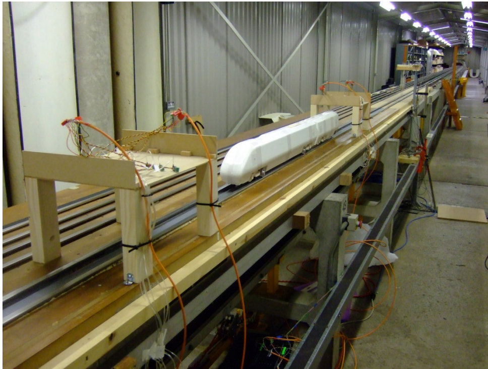
Figure 32. TRAIN rig reduced scale model testing facility in Derby, England, set up to measure pressure on a short overhead canopy
