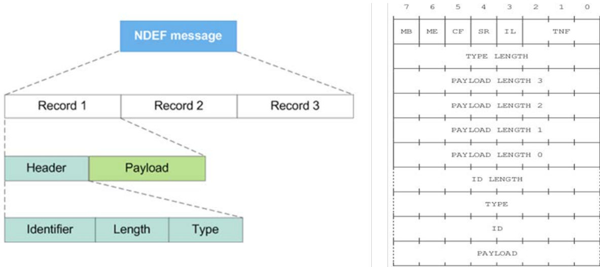
Figure 5. NDEF Message and Record Structure
