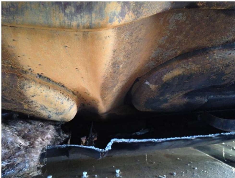
Figure 44. Localized tank buckling between coils at tank center, near base of tank. Jacket cut away locally to expose inner tank.
