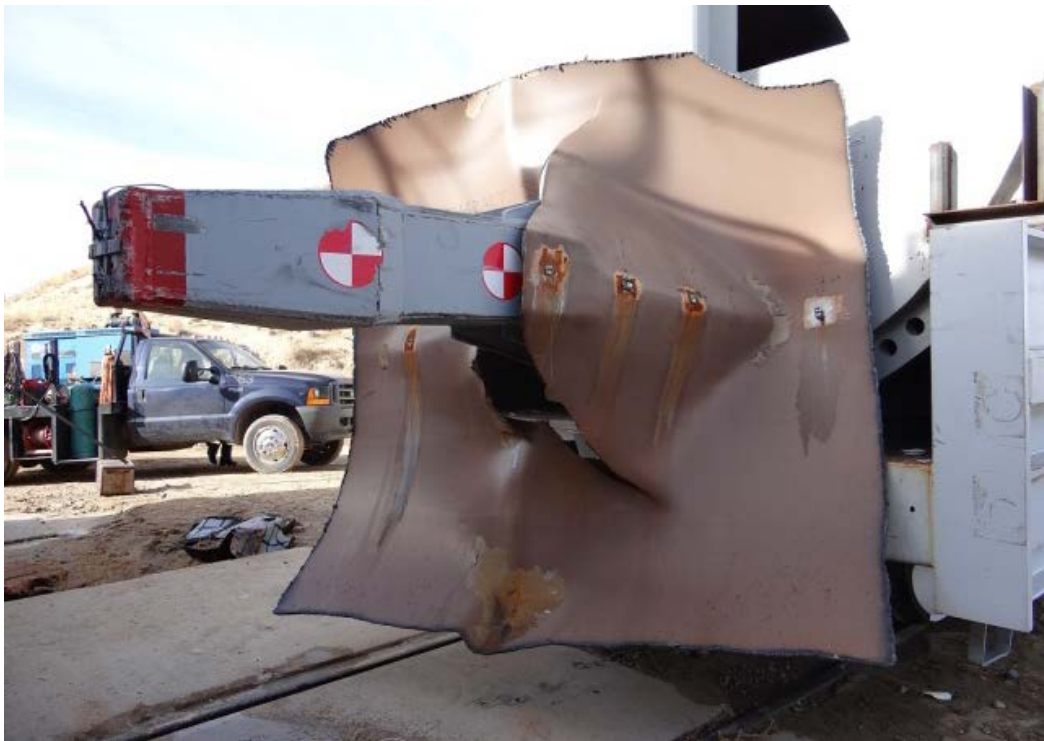
(b) Punctured tank shell
