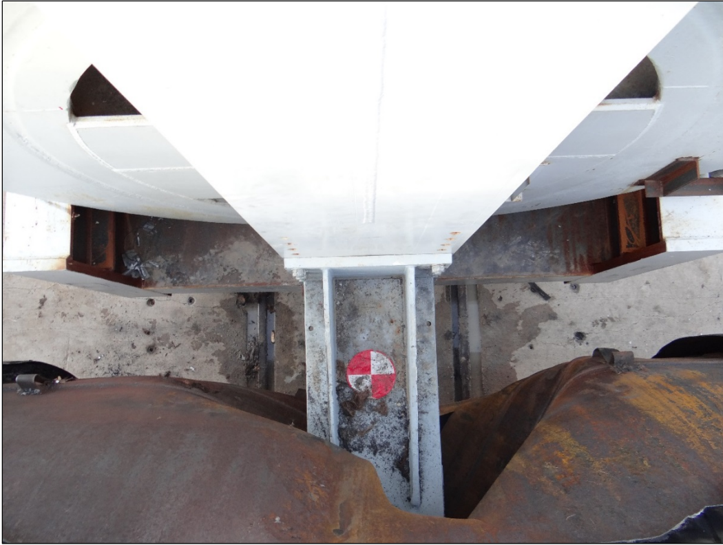
Figure A-7. Punctured Shell after the Test
