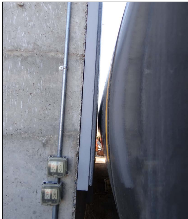
Figure A-4. Distance between Impact Wall and Tank Car (Pre-Test)
