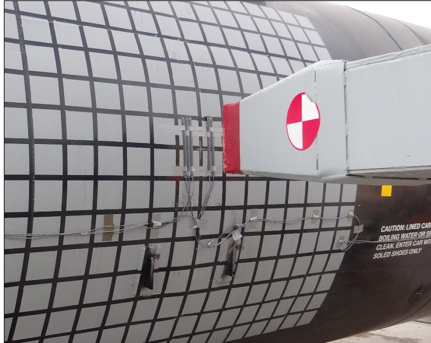
Figure A-3. Ram Indenter Alignment and Trigger System
