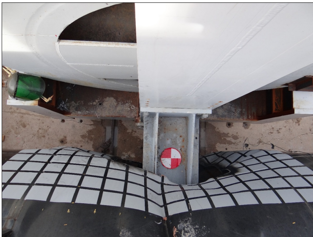
Figure A-6. Punctured Jacket after the Test
