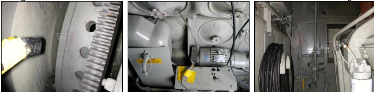
(a) RPM sensor; (b) manifold absolute pressure (MAP) sensor; (c) intake air temperature (IAT) sensor
