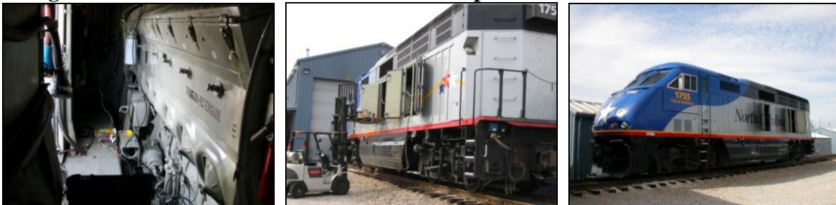
(a) routing sampling hoses and cables; (b) routing sampling hoses through a side door, secured with ties (rear-view); (c) side-view of F59PHI locomotive
