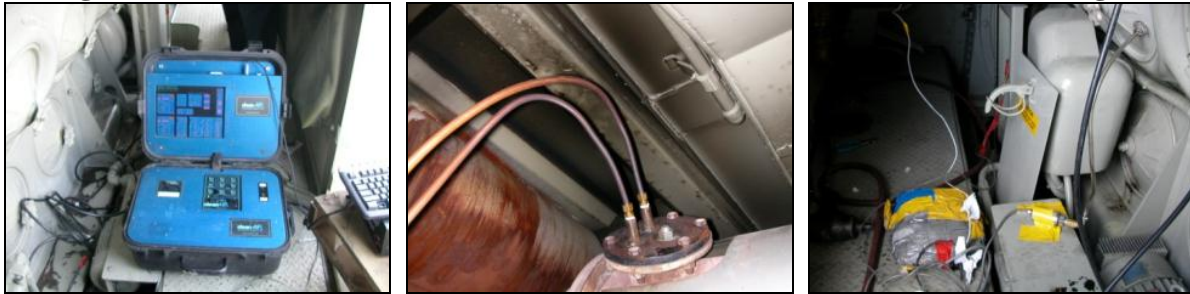
(a) PEMS main unit (front-view); (b) exhaust sampling port and metal tubes; (c) sensor array box
