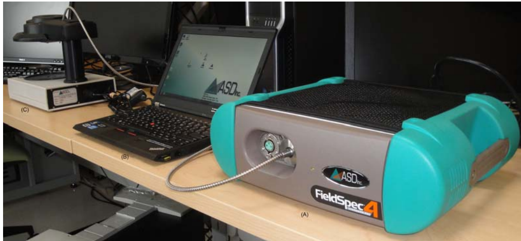
Figure 1. ASD FS4 Setup: (A) – FS4, (B) – Computer Control, and (C) – ASD Turntable.
