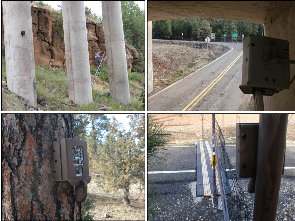
Figure 12. Examples of Camera Orientations at Munds Canyon Bridge (Upper Left); Schnebly Hill Road TI (Upper Right); Jump-out Near MP 320 (Lower Left); Electrified Cattle Guard at Schnebly Hill Road TI (Lower Right)
