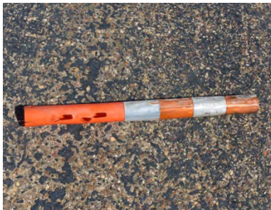
Figure A-6. Sample 3B Failure at 28 Impacts.
