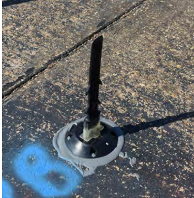
Figure A-14. Sample 7B Failure at 18 Impacts.
