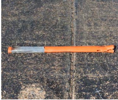
Figure A-10. Sample 5B Failure at 21 Impacts.
