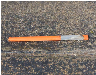
Figure A-16. Sample 8B Failure at 28 Impacts.
