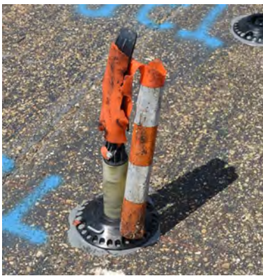
Figure A-5. Sample 3T Failure at 71 Impacts.
