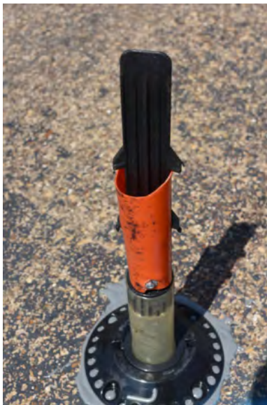
Figure A-8. Sample 4B Failure at 42 Impacts.
