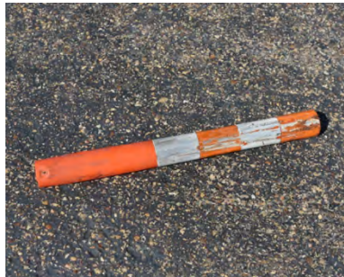
Figure A-2. Sample 1B Failure at 27 Impacts.
