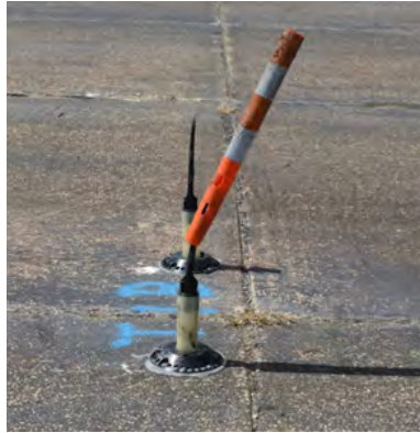
Figure A-1. Sample 1T Failure at 53 Impacts.
