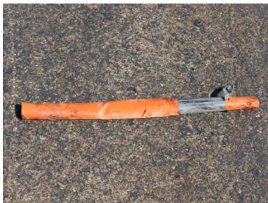
Figure A-12. Sample 6B Failure at 29 Impacts.
