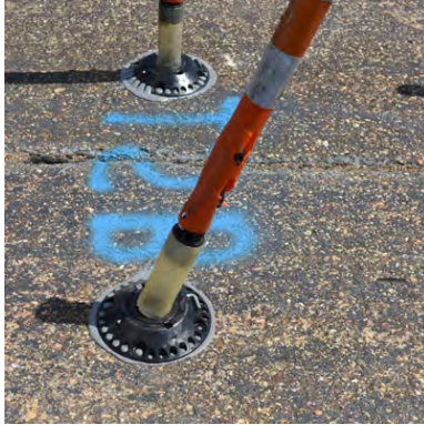
Figure A-4. Sample 2B Failure at 44 Impacts.
