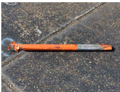
Figure A-13. Sample 7T Failure at 29 Impacts.
