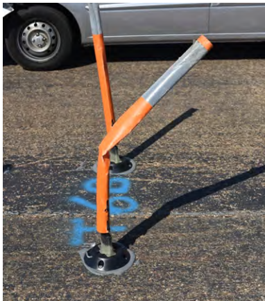
Figure A-11. Sample 6T Failure at 25 Impacts.
