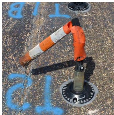
Figure A-3. Sample 2T Failure at 66 Impacts.
