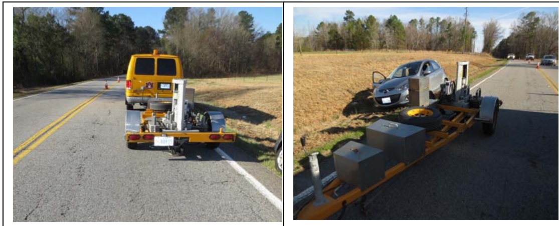
Figure 4—FWD Deflection Testing in Right Wheel Path
