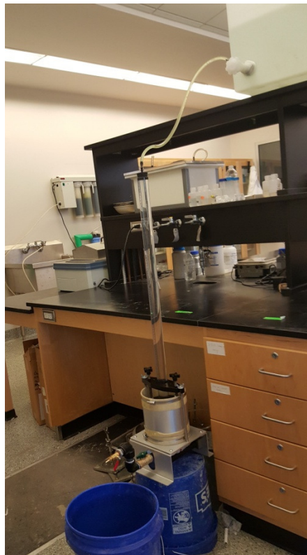
Figure 2-4. Experimental setup for dynamic adsorption test
