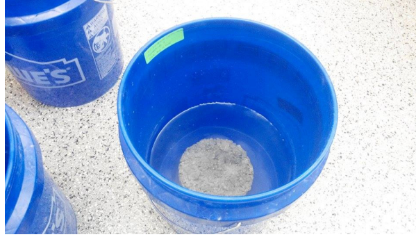
Figure 2-3. Batch adsorption test
