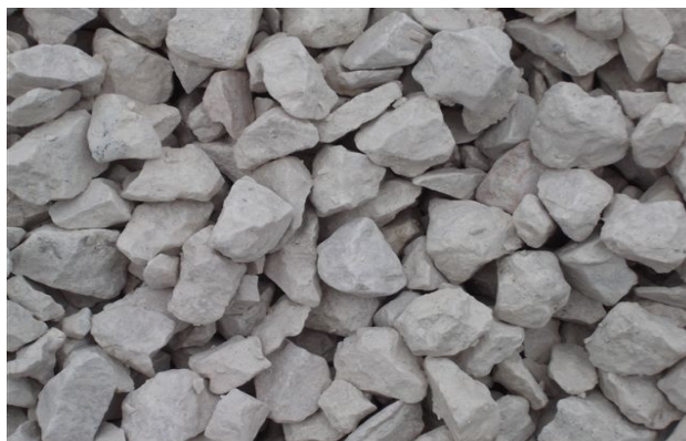
Figure 2-1. Crushed lime stones used in PCP and MPCP sample fabrication
