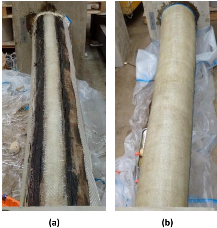
Figure 4-8. FRP-retrofitted timber pile specimens: (a) SP1; (b) SP2.
