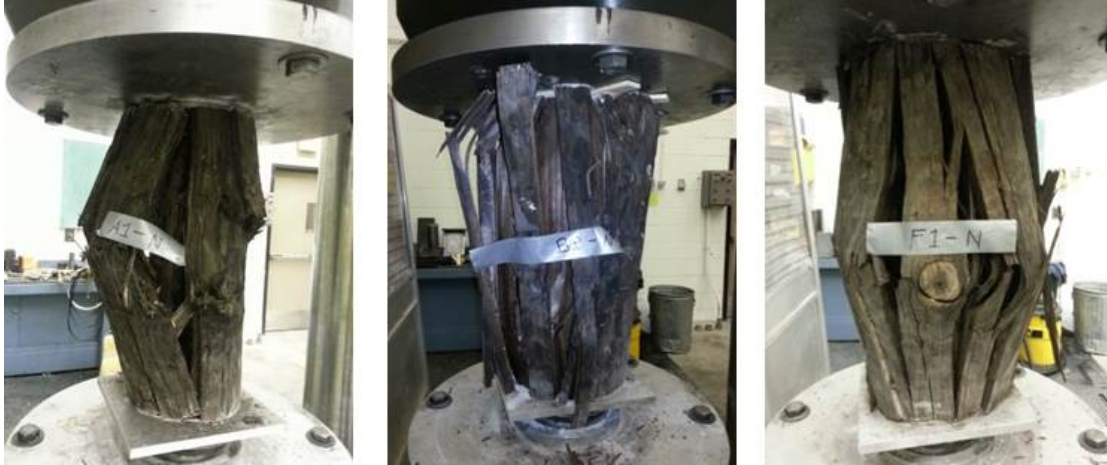
Figure 5-5. Failure of unretrofitted timber specimens.
