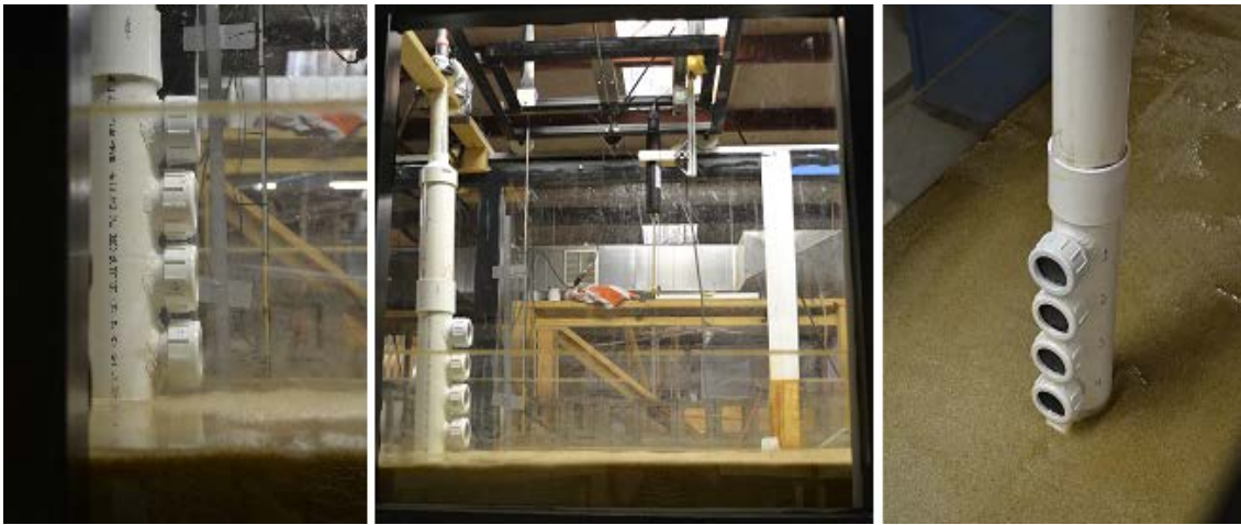
Figure 3.4: Prototype VTP array installed in the flume. VTPs 1-4 are shown above the sand bed. The instrument is anchored to the flume wall.
