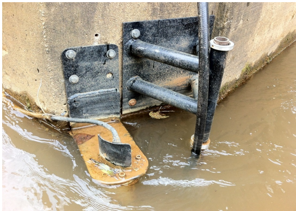
Figure 6.5: TDR (on the right) and VTP (on the left) at Field Site 1.
