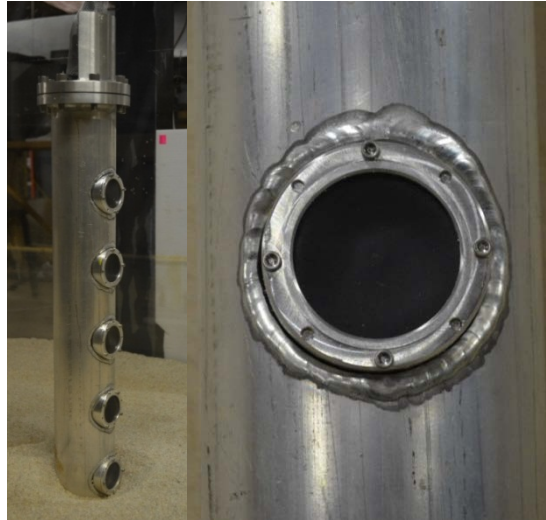
Figure 5.10: VTP setup as installed in CHL flume for channel effects study.
