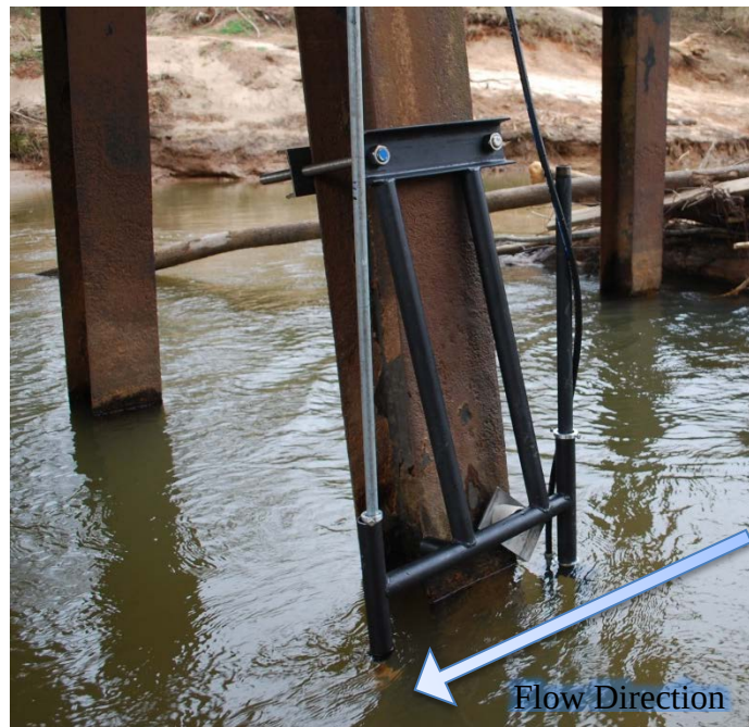
Figure 6.8: Installed TDR (on the right) and sonar (on the left) at Field Site 2.
