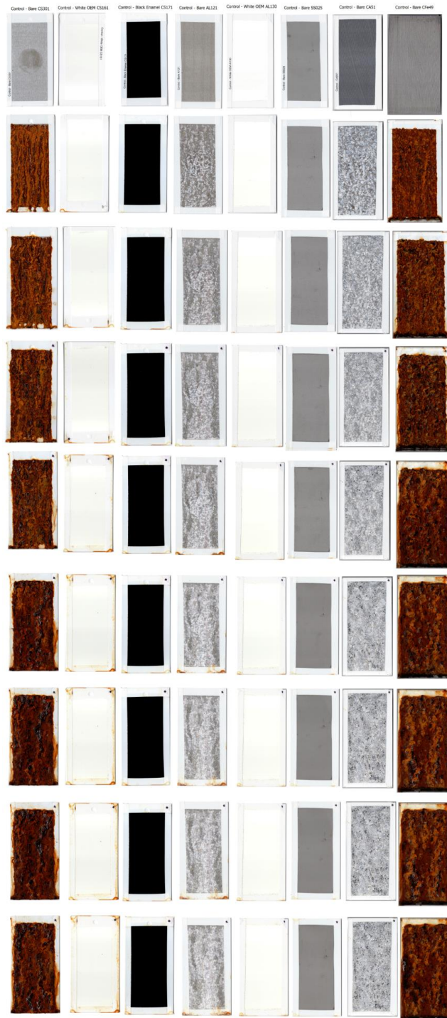
Figure F 1. Control unscrubbed metal panels exposed to the salt spray chamber
