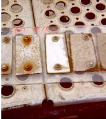
Figure L 3: Metal coupons used to measure corrosion on winter maintenance vehicles. Corrosion rate was measured as weight lost over time due to exposure of the coupons to two different salt solutions (Xi and Xie 2002).
