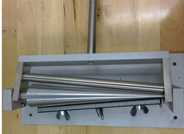
Figure B 4. Conical mandrel test apparatus.
