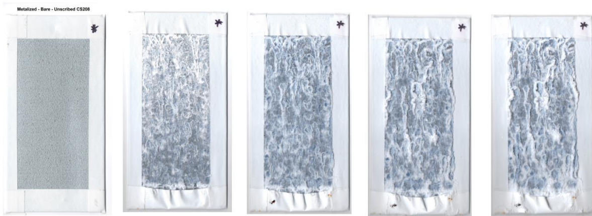
Figure F 5. Metalized unscribed metal panels exposed to the salt spray chamber.
