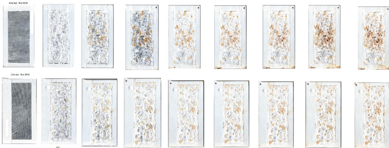
Figure 3.1-11: Example of unscribed coated panels (galvanized) after salt spray exposure. From left to right, scans of the panels were taken each week for eight weeks.
