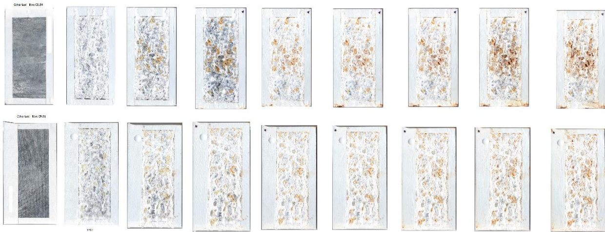
Figure F 2. Galvanized unscribed metal panels exposed to the salt spray chamber.
