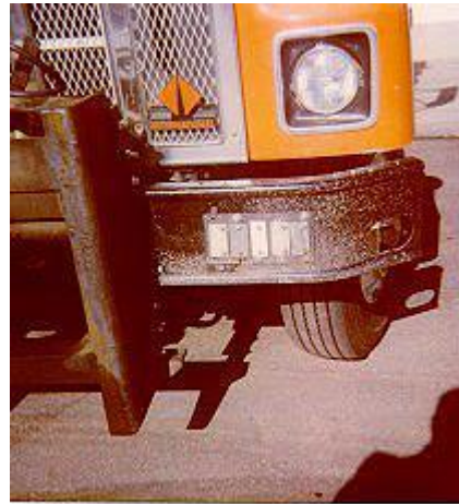
Figure L 3: Metal coupons used to measure corrosion on winter maintenance vehicles. Corrosion rate was measured as weight lost over time due to exposure of the coupons to two different salt solutions (Xi and Xie 2002).
