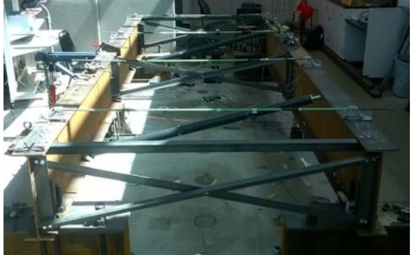
Figure D.43 1 Cross frame at midspan + 2 diagonal pipes+ 3 transverse ties (1-CF + 2-DP + 3-TT).
