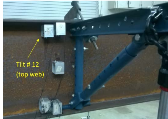
Figure 5.5 Tilt sensors at loaded girder at midspan.
