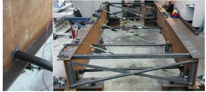
Figure D.19 Horizontal steel pipes at scaled model.
