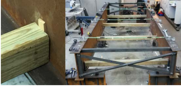
Figure D.18 Timber blocks at scaled model.
