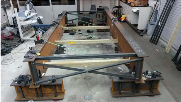
Figure D.46 3 unadjusted diagonal ties + 3 timber blocks (3-UDT + 3-TB).
