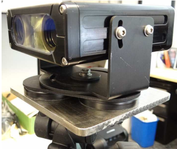
Figure 2: ELSAG ALPR Cameras Mounted to Tripods
