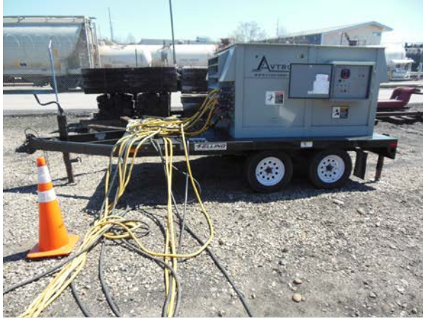
(a) Avtron Model K580 Load Box with Connected Cables
