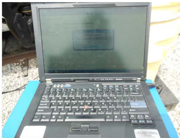
(b) Laptop Logging Engine Control Unit Data
