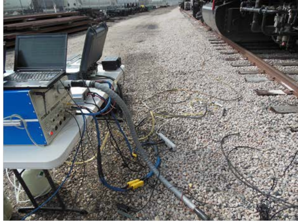
(b) Exhaust Sampling Lines and Accessories Connected to Portable Emission Measurement Systems
