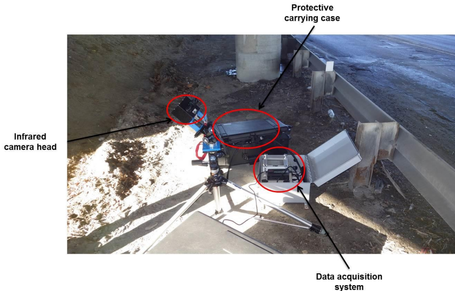
Figure 47. Photograph of the test setup for the West Blvd Bridge.
