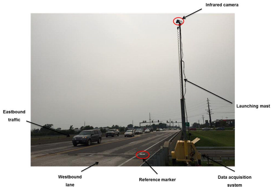
Figure 34. – Photograph showing the position of the IR-UTD portable mast during data collection on the Grindstone Bridge.
