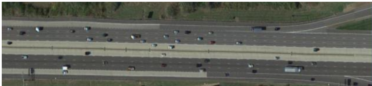
FIGURE 4.2.3 Example of Add and Drop Lanes
