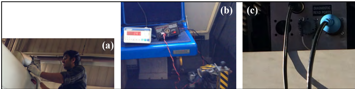
Figure 8. NO x Analyzer (a) Probe Setup on the Tail Pipe, (b) Instrument Setup Inside, and (c) 9-Pin Plug Connector
