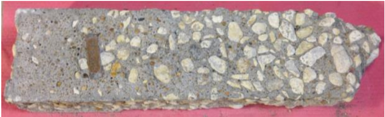
Figure G.2: Surface Scaling of Florence Aggregate Sample
