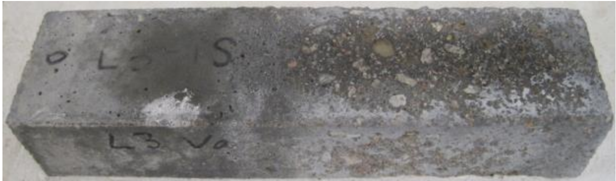
Figure F.6: L3 Half-Immersed Concrete Prism
