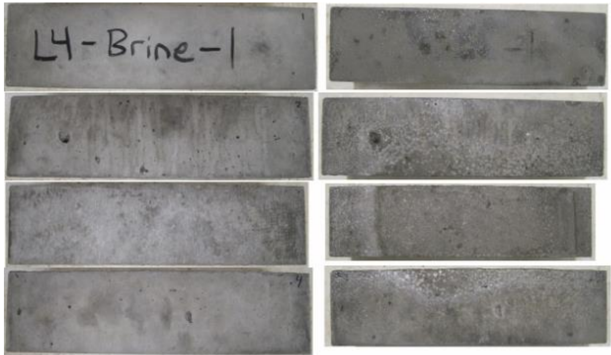
Figure C.21: First L4 Prism in Rock Salt Brine
