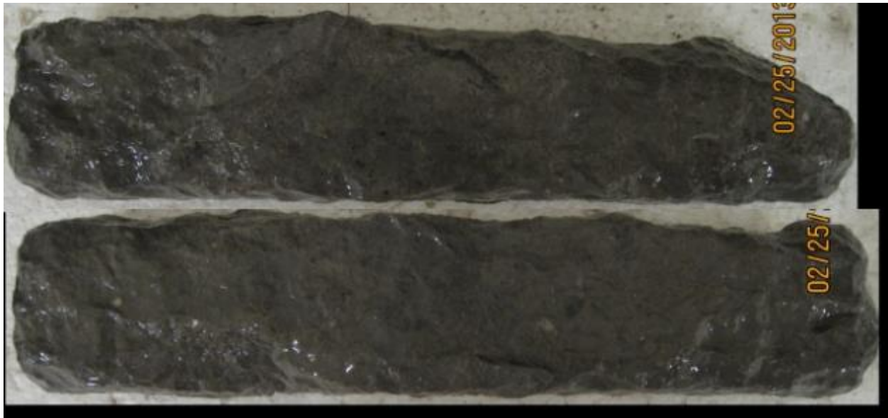
Figure D.1: Unidentifiable Prism After Salt-Frost Exposure
