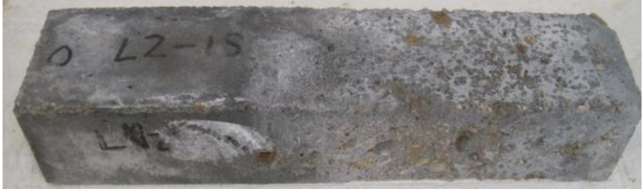
Figure F.5: L2 Half-Immersed Concrete Prism
