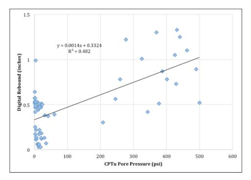
Figure 4-21: Digital Rebound versus CPTu pore pressure from six test sites with rebound > 0.5 inches
