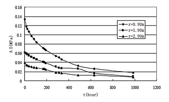
Figure 2-26: Change in pore pressure versus time for the three sensor locations (Bingjian, 2011)
