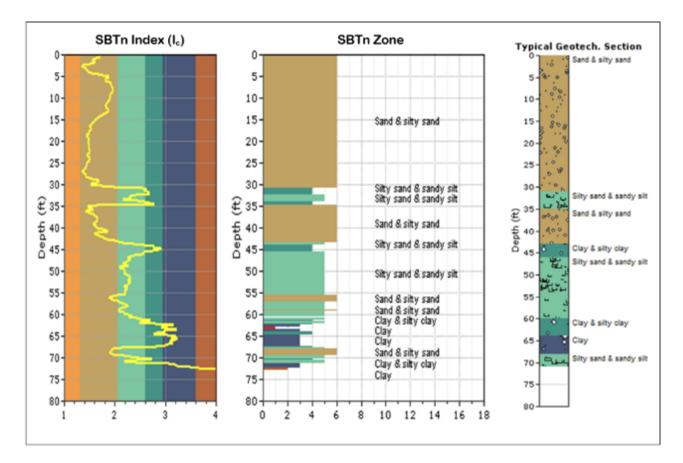
Figure 4-11: Normalized soil behavior type index and typical geotechnical section for SR 417 International Parkway at B1/pile 14 (GSE = 72.3 ft)
