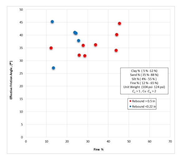
Figure F-3: Fine Content (%) Vs. Effective Friction Angle- Cohesionless soils (SM)
