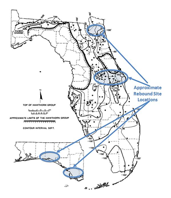
Figure 2-27 Top elevation contours of the Hawthorn Group with approximate high pile rebound site locations [after Scott (1990)]
