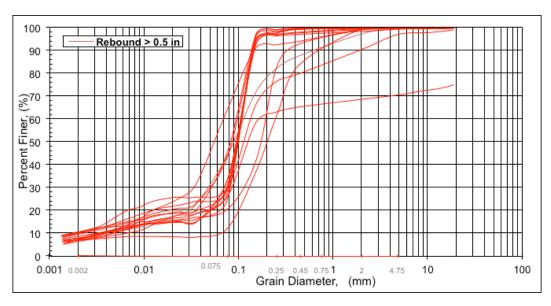
Figure 6.2: Grain size distribution curves for nonHPR cohesionless soils
