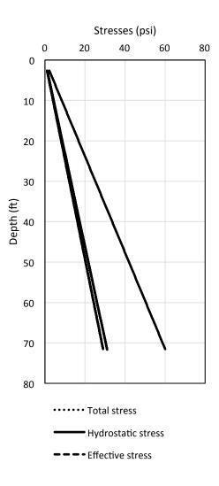
Figure A-6 Total stress, hydrostatic pore water pressure, and effective stress versus depth for I-4 Widening Daytona at EB3 / pile 5
