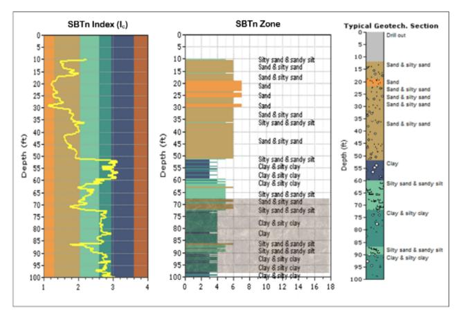
Figure 4-10: Normalized soil behavior type index and typical geotechnical section for I-4/US 192 at Pier 8/pile 4 with HPR zone shaded (GSE = 90.2 ft)
