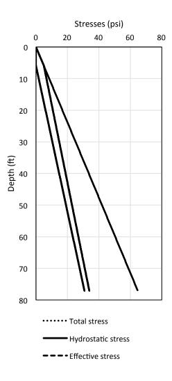
Figure A-3 Total stress, hydrostatic pore water pressure, and effective stress versus depth for SR 50 / SR 436 at west bound / pile 5
