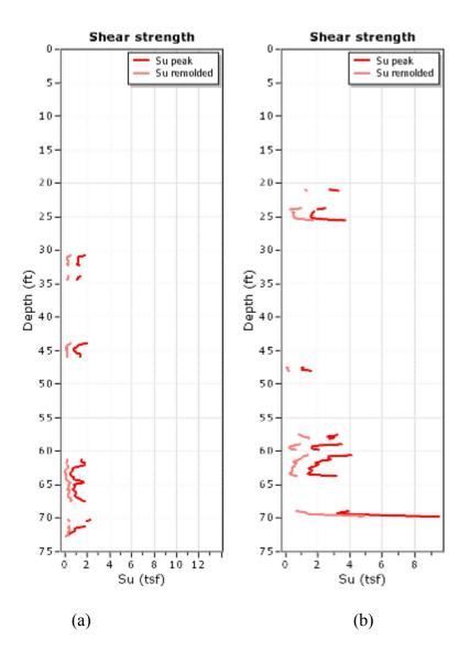
Figure 4-25: Undrained shear strength for SR 417 International Parkway at (a) B1/pile 14 and (b) B2/pile 5
