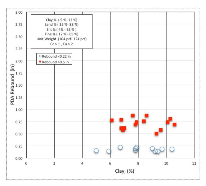
Figure 6.7: Clay Content (%) vs. PDA HPR (in) - cohesionless soils (SM) from all sites
