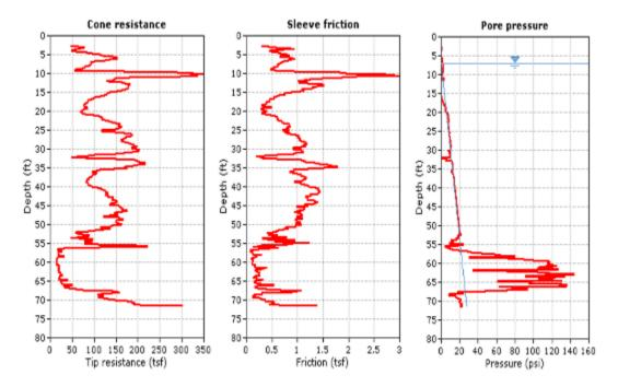
Figure 3-27: CPTu q<sub>c</sub>, f<sub>s</sub>, and u<sub>2</sub> versus depth near EB3/pile 5 at I-4 Widening Daytona
