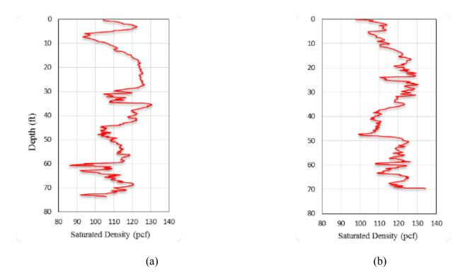
Figure 4-2: Saturated density versus depth for SR 417 International Parkway at (a) B1/pile 14 (b) B2/pile 5
