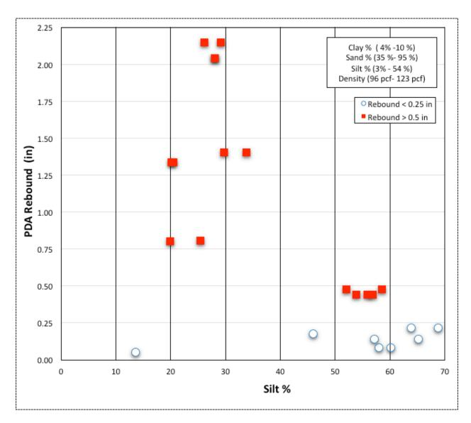
Figure 6.6: Silt content (%) vs. PDA HPR (in) - cohesive soils (CH, CL) from all sites
