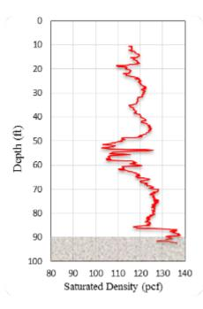
Figure 4-5: Saturated density versus depth for Anderson Street at pier 6/piles 5 and 6 with HPR zones shaded
