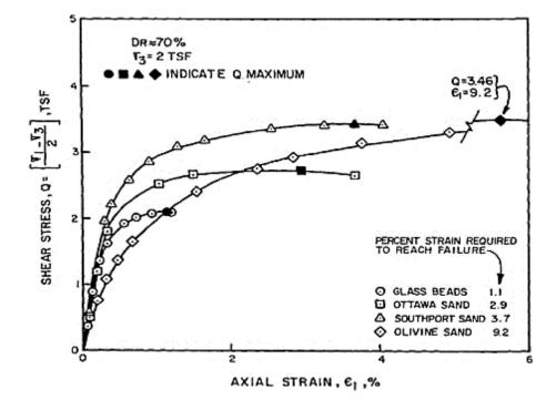
Figure 2-15: Effect of particle shape on stress-strain curves from constant cell pressure tests (Holubec, & D'Appolonia, 1972)
