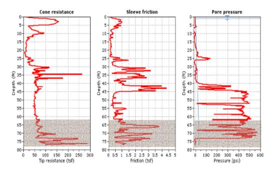
Figure 3-31: CPTu  $q_c$ ,  $f_s$ , and  $u_2$  versus depth from CPT-1 near EB5/pile 2 at SR 83/ Ramsey Branch Bridge
