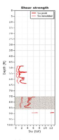
Figure 4-28: Undrained shear strength for Anderson Street at pier 6 with HPR zone shaded
