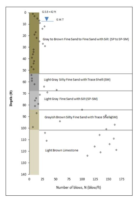
Figure 3-26: General soil profile with USCS classification and the actual N<sub>SPT</sub> from SPT boring SPT DC-1 near EB3/pile 5 at I-4 Widening Daytona
