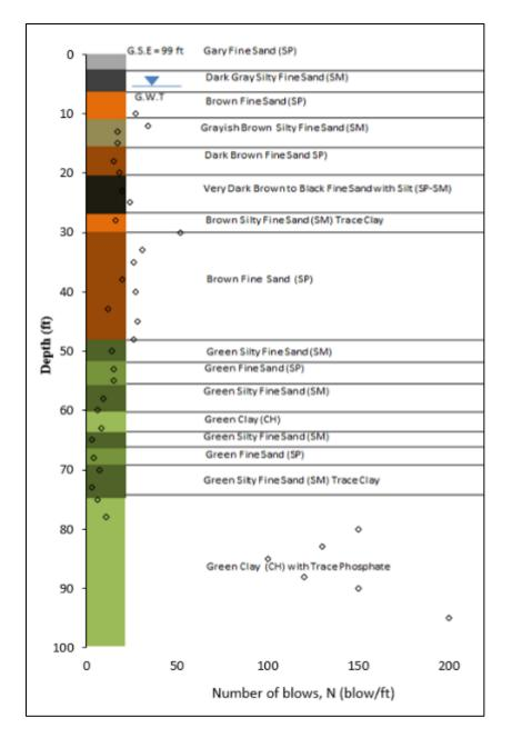
Figure 3-14: General soil profile with USCS classification and the actual N<sub>SPT</sub> from SPT boring TH-4B near pile 5 at the westbound side of SR50/SR436
