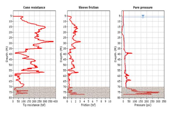
Figure 3-15: CPTu  $q_c$ ,  $f_s$ , and  $u_2$  versus depth from CPT-1 near pile 5 at the westbound side of SR 50 / SR436
