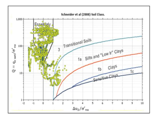
Figure 7.8: NonHPR data overlaid on Schneider et al.'s (2008) SBT chart
