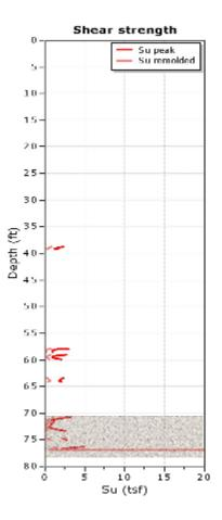
Figure 4-26: Undrained shear strength for SR 50/SR 436 at westbound/pile 5 with HPR zone shaded
