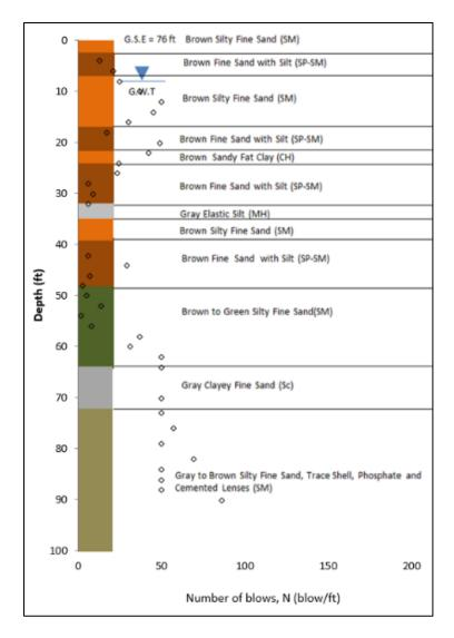
Figure 3-9: General soil profile with USCS classification and N<sub>SPT</sub> from SPT borings SPT-B1 and SPT-B2 for SR 417 International Parkway I-4 Interchange
