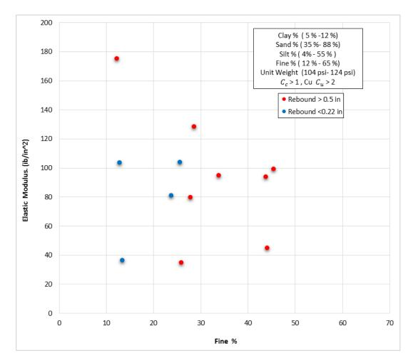
Figure F-2: Fine Content (%) Vs. Elastic Modulus (psi)- Cohesionless soils (SM)
