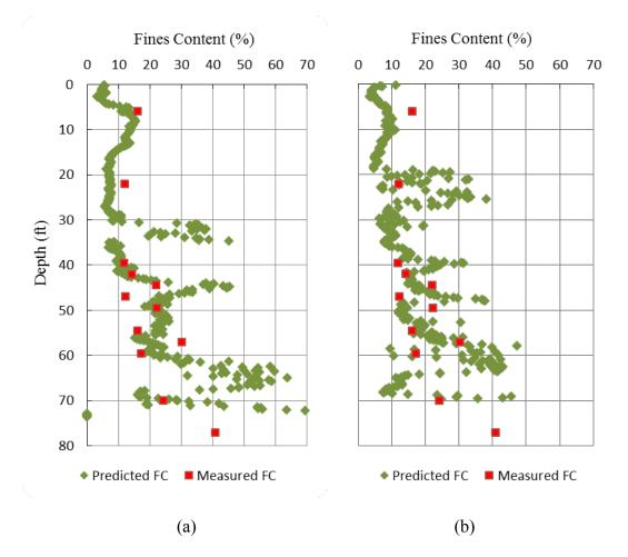
Figure 4-35: Predicted and measured fines content versus depth for SR 417 International Parkway at (a) B1/pile 14 (b) B2/pile 5
