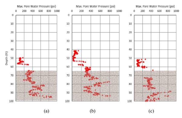
Figure 4-32: Gui and Jeng 's (2009) maximum compression-induced pore water pressure due to driving 24-inch prestressed concrete piles with HPR zones shaded for I-4/US 192 at (a) pier 6/pile 16, (b) pier 7/pile 10, and (c) pier 8/pile 4
