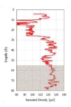
Figure 4-7: Saturated density versus depth for SR 83/Ramsey Branch Bridge at EB5/pile 2 with HPR zones shaded
