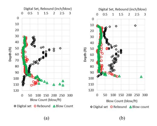
Figure 3-21: Digital set, pile rebound, and N<sub>PD</sub> versus depth for (a) pier 6/pile 6 and (b) pier 6/pile 5 at the Anderson Street overpass
