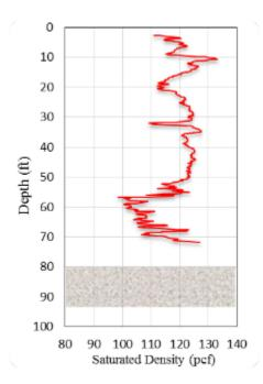
Figure 4-6: Saturated density versus depth for I-4 Widening Daytona at EB3/pile 5 with HPR zones shaded
