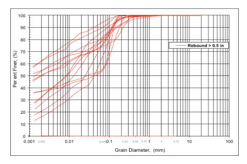
Figure 6.3: Grain size distribution curves for high pile HPR cohesive soils
