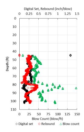
Figure 3-25: Digital set, pile rebound, and N<sub>PD</sub> versus depth for EB3/pile 5 at I-4 Widening Daytona
