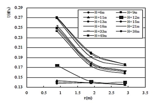
Figure 2-25: Excess pore pressure versus radial distance at discrete driving depths curve (From Bingjian, 2011)
