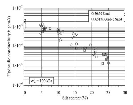
Figure 2-42: Hydraulic conductivity for various silt contents (Bandini & Sathiskumar, 2009)
