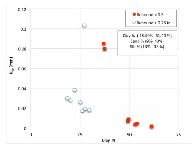
Figure 6.18: Clay content (%) vs. D<sub>60</sub> content – cohesive soils (CH, CL) from all sites
