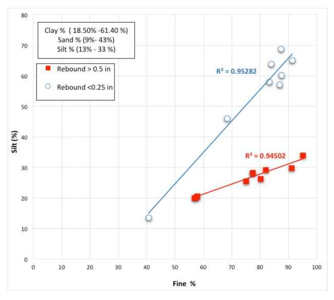
Figure 6.20: Silt content (%) vs. fines content (%) – cohesive soils (CH, CL) from all sites
