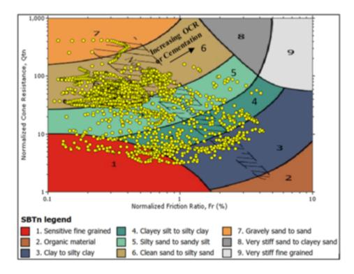
Figure 7.2: NonHPR data overlaid on Robertson's (1990) normalized cone resistance versus normalized friction ratio SBT chart with the normally consolidated zone shown.
