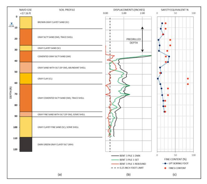
Figure 3-34: (a) FDOT and TH-6 soil profile, (b) PDA diagram, (c)  $N_{safe}$  and FC for Heritage Parkway test pile B3P1
