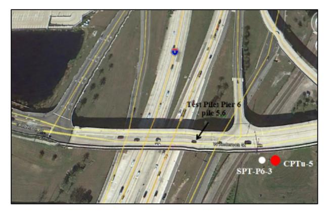
Figure 3-20: Test piles, SPT boring, and CPTu sounding locations for the Anderson Street overpass
