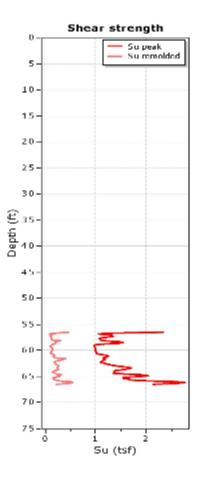
Figure 4-29: Undrained shear strength for I-4 Widening Daytona at EB3/pile 5
