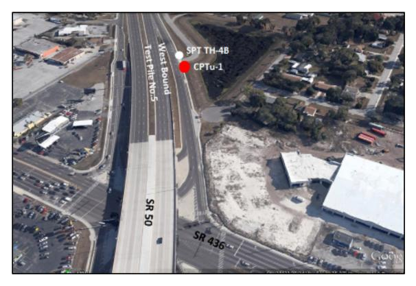
Figure 3-12: Test piles, SPT boring, and CPTu sounding locations for SR50/SR436
