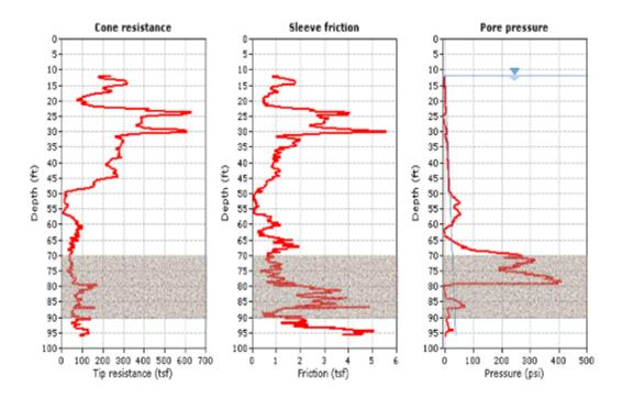
Figure 3-4: CPTu qc, fs, and u2 versus depth from CPTu-4 near pier 6/pile 16 at I-4/US 192
