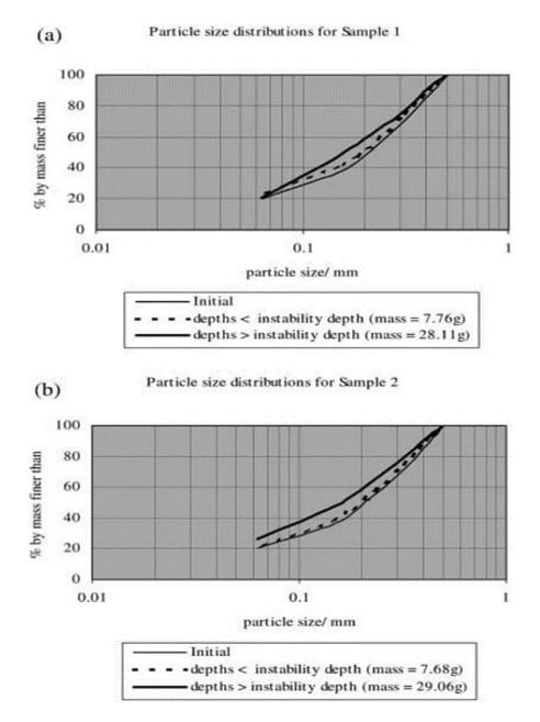
Figure 2-19: Particle size distributions for samples 1 and 2 at depths less than and greater than the instability depth (McDowell & Bolton, 2000)
