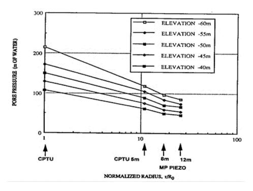
Figure 2-22 Relationship between measured pore pressures from CPT<sub>u</sub> and MP piezometers with normalized radial distance from pile (Robertson et al., 1990)
