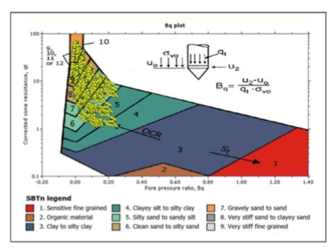
Figure 7.4: NonHPR data overlaid on Robertson's (1990) cone resistance versus pore pressure ratio SBT chart
