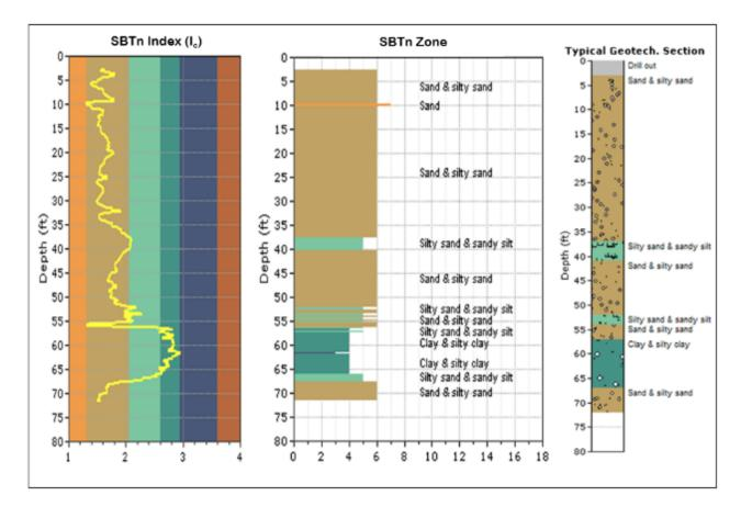
Figure 4-16: Normalized soil behavior type index and typical geotechnical section for I-4 Widening Daytona at EB3/pile 5 (GSE = 42.0 ft)
