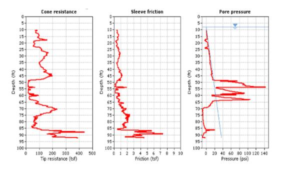
Figure 3-23: CPTu  $q_c$ ,  $f_s$ , and  $u_2$  versus depth from CPT-5 near pier 6 at the Anderson Street overpass
