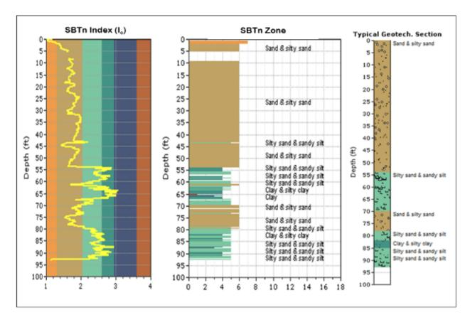
Figure 4-14: Normalized soil behavior type index and typical geotechnical section for I-/SR408 at pier 2/pile 5 (GSE = 106 ft)
