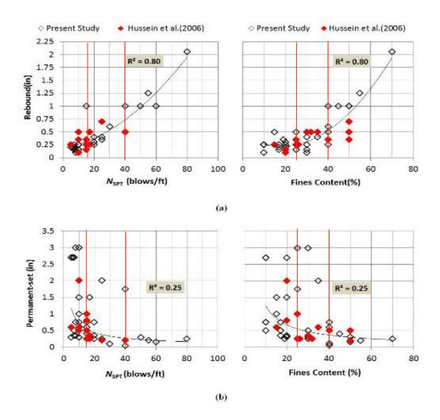
Figure 2-44 (a) Correlation between rebound, NSPT, and fines content, and (b) correlation between permanent-set, N<sub>SPT</sub> and fines content (Jarushi et al., 2013).
