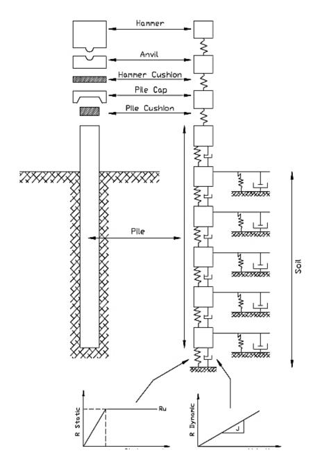
Figure 2-4: Pile-soil model for wave equation analysis (after Smith, 1960)
