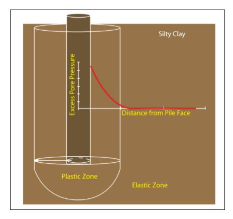
Figure 4-31: Plastic and elastic zones around single driven pile (Wren, 2007)
