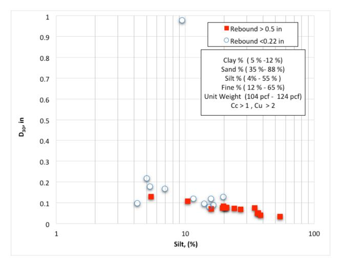
Figure 6.16: Silt content (%) vs. D<sub>30</sub> content – cohesionless soils (SM) from all sites
