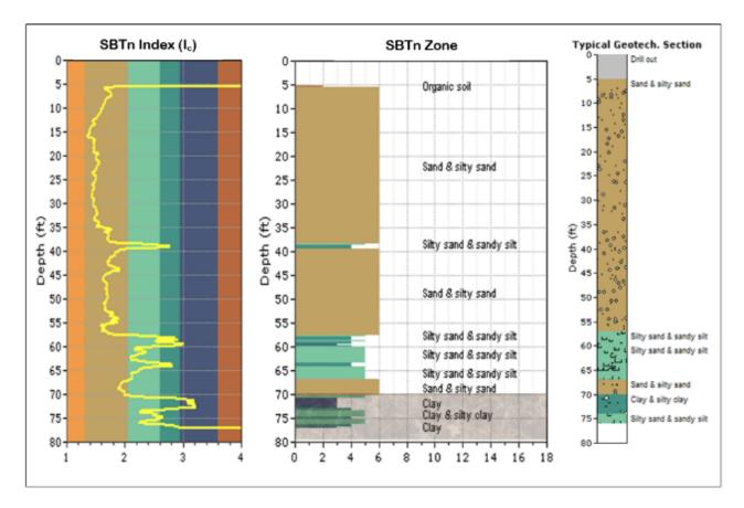
Figure 4-13: Normalized soil behavior type index and typical geotechnical section for SR 50/SR436 at west bound/pile 5 with HPR zone shaded (GSE = 99.0 ft)
