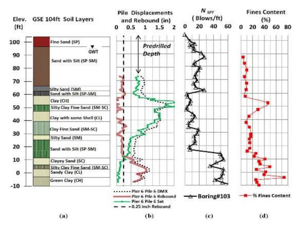
Figure 2-43: (a) Generalized soil profile, (b) PDA diagram, (c) N<sub>SPT</sub>, and (d) percent fines content for site 1 Anderson Street Overpass (Jarushi et al., 2013).
