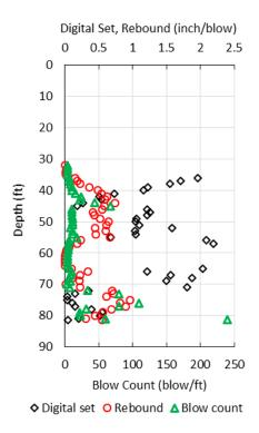
Figure 3-13: Digital set, pile rebound, and  $N_{PD}$  versus depth for pile 5 for the westbound side of SR 50 / SR 436
