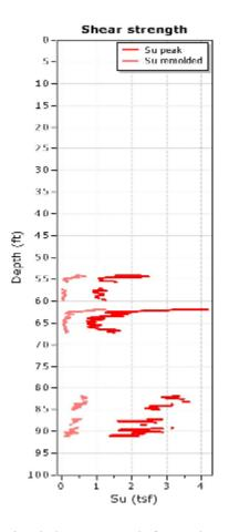
Figure 4-27: Undrained shear strength for I-4/SR 408 at pier 2/pile 5
