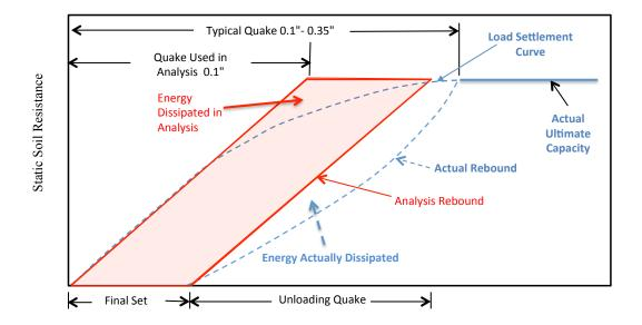
Figure 2-2: Resistance vs. penetration with quake for one hammer blow (modified after Smith, 1960)
