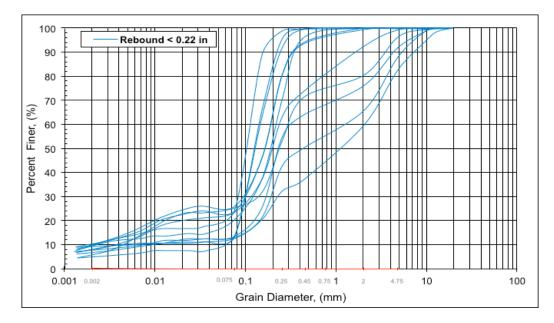
Figure 6.1: Grain size distribution curves for high pile HPR cohesionless soil
