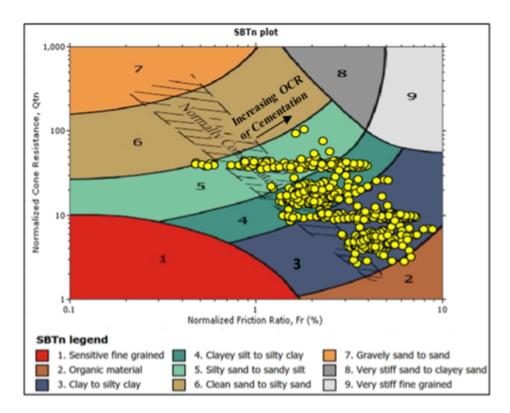
Figure 7.1: HPR data overlaid on Robertson's (1990) normalized cone resistance versus normalized friction ratio SBT chart with the normally consolidated zone shown
