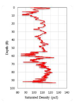
Figure 4-4: Saturated density versus depth for I-4/SR408 at pier 2/pile 5
