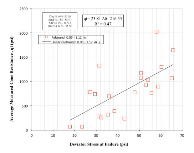
Figure 6.31 Averaged CPTu cone tip resistance near thin-walled tube sample versus cyclic triaxial deviator stress at failure from corresponding sample
