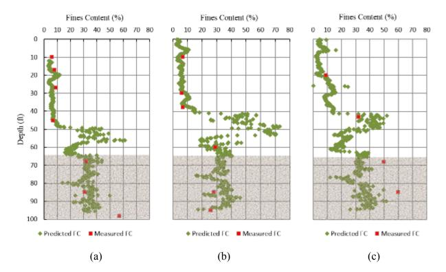
Figure 4-34: Predicted and measured fines content versus depth for I-4/US 192 at (a) Pier 6/pile 16 (b) Pier 7/pile 10 (c) Pier 8/pile 4 with HPR zones shaded
