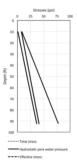
Figure A-5 Total stress, hydrostatic pore water pressure, and effective stress versus depth for Anderson Street at pier 6 / pile 5, 6
