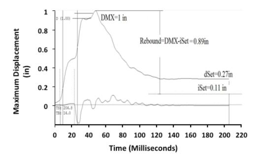
Figure 2-8: Typical PDA pile top displacement versus time diagram from one hammer blow for an FDOT HPR site (Cosentino et al., 2010)
