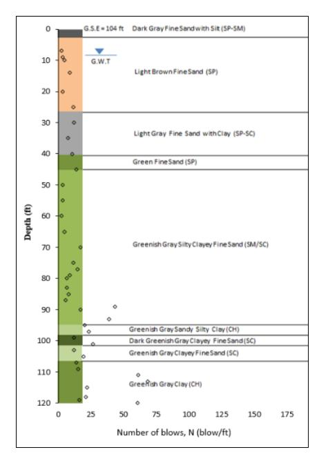
Figure 3-22: General soil profile with USCS classification and the actual N<sub>SPT</sub> from SPT boring SPT P6-3 near pier 6 at the Anderson Street overpass
