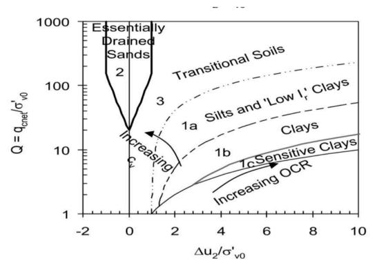
Figure 2-34: Normalized SBT chart developed by Schneider et al. (2008)
