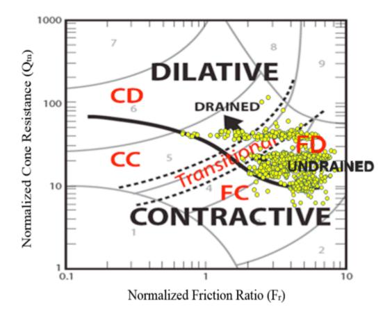
Figure 7.5: HPR data overlaid on Robertson's (2012) updated normalized cone resistance versus friction ratio SBT chart
