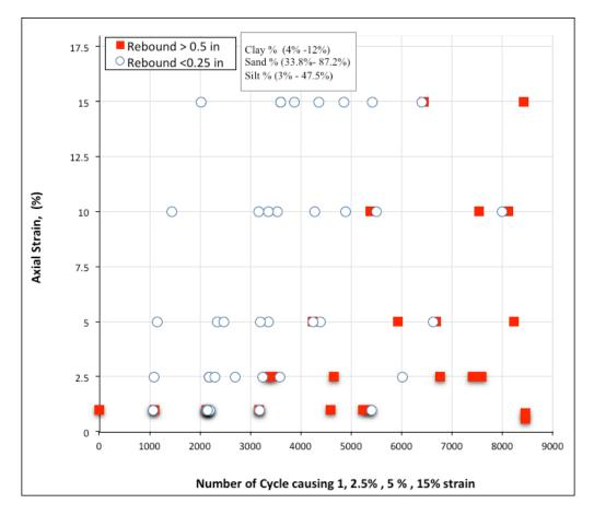
Figure 6.27: Number of cycles required to achieve 1%, 2.5%, 5%, 10%, and 15% strain for cohesionless soils susceptible to HPR and nonHPR
