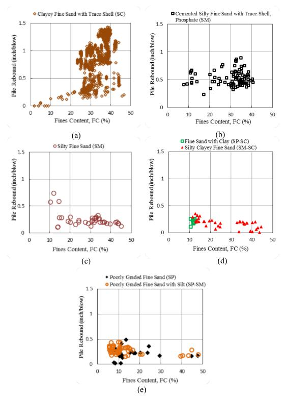
Figure 4-41: Pile rebound versus CPTu FC for different soil types
