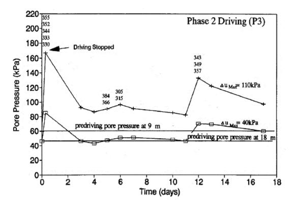
Figure 2-23: Pore water pressure changes due to pile driving (Eigenbrod & Issigonis, 1996)
