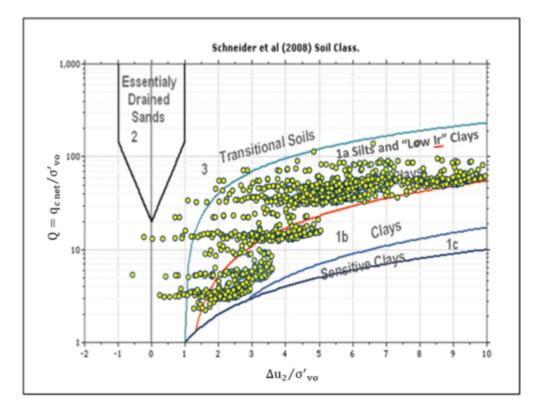
Figure 7.7: HPR data overlaid on Schneider et al.'s (2008) SBT chart
