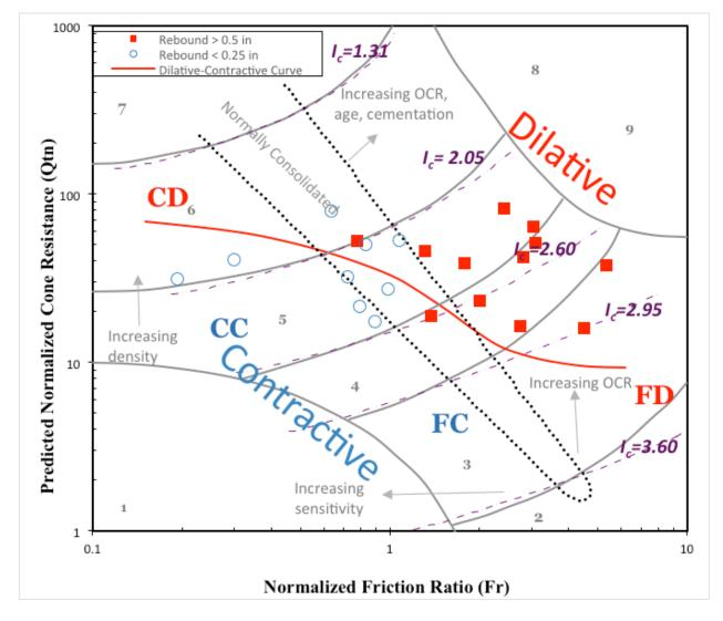
Figure 6.32: Estimated soil behavior based on regression equation from HPR and nonHPR laboratory samples on Robertson's (2012) updated normalized cone resistance versus friction ratio SBT chart
