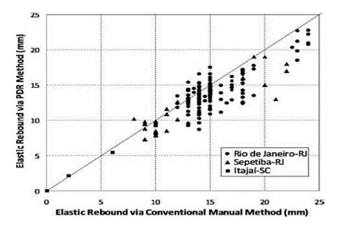
Figure 2-10: Comparison between elastic rebound results obtained with conventional manual method and the pdr system (Oliveira et al., 2013).
