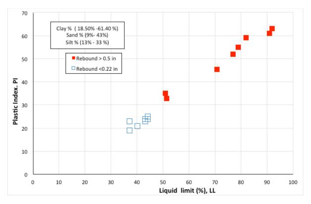
Figure 6.22: Liquid limit (LL) versus Plastic Index, (PI) for cohesive (CL, CH) soils
