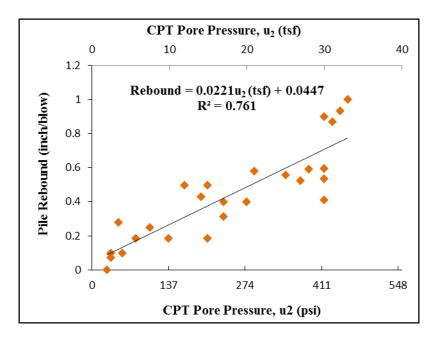
Figure 4-19: Pile rebound for 24 24-inch precast concrete piles versus CPTu u2 (Jarushi et al.,
