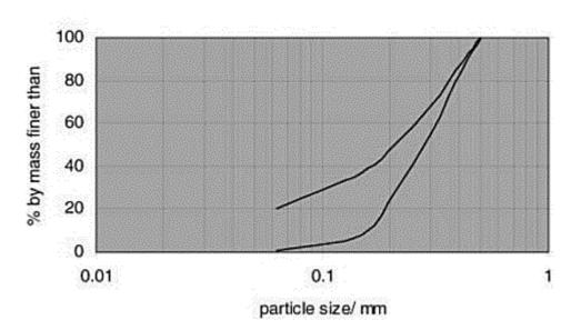
Initial particle size distributions for the two gradings of soil
