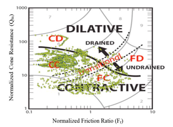
Figure 7.6: NonHPR data overlaid on Robertson's (2012) updated normalized cone resistance versus friction ratio SBT chart
