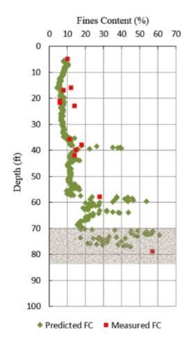
Figure 4-36 for Predicted and measured fines content versus depth for SR 50/SR 436 at westbound/pile 5 with HPR
