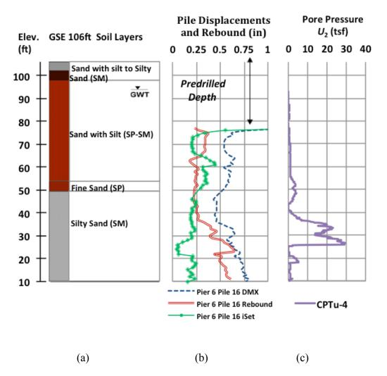
Figure 2-46: (a) Generalized soil profile, (b) PDA diagram and (c) CPTu pore-water pressure (u<sub>2</sub>) for Site 3 I-4/US.192 (Cosentino et al., 2013).
