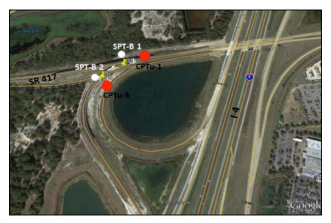
Figure 3-7: Test piles, SPT boring, and CPTu sounding locations for SR 417 International Parkway I-4 Interchange
