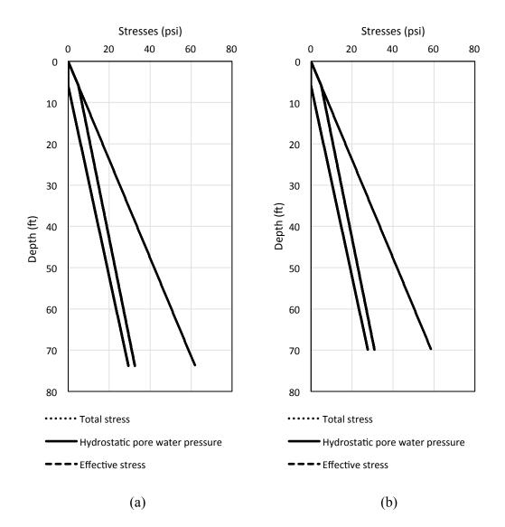
Figure A-2 Total stress, hydrostatic pore water pressure, and effective stress versus depth for SR 417 International Parkway at (a) B1 / pile 14 and (b) B2 / pile 5
