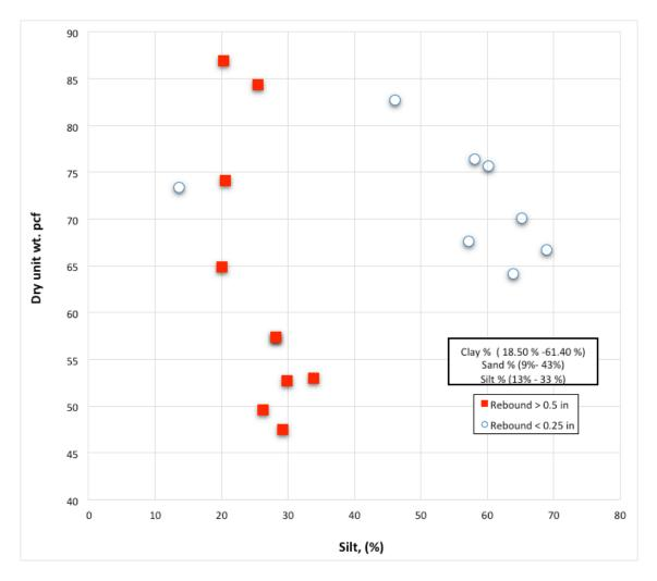
Figure 6.26: Dry unit weight vs. silt content - cohesive soils (CH, CL) from all sites
