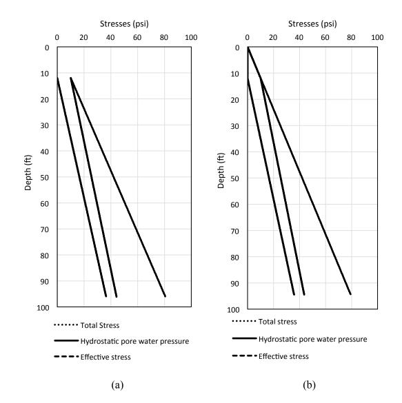
Figure A-1 Total stress, hydrostatic pore water pressure, and effective stress versus depth for I-4 / US 192 at (a) pier 6 / pile 16 and (b) pier 7 / pile 10
