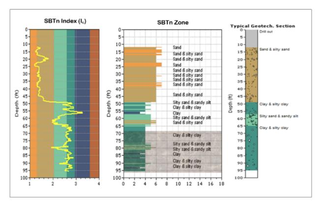
Figure 4-8: Normalized soil behavior type index and typical geotechnical section for I-4/US 192 at Pier 6/pile 16 with HPR zone shaded (GSE = 109.6 ft)
