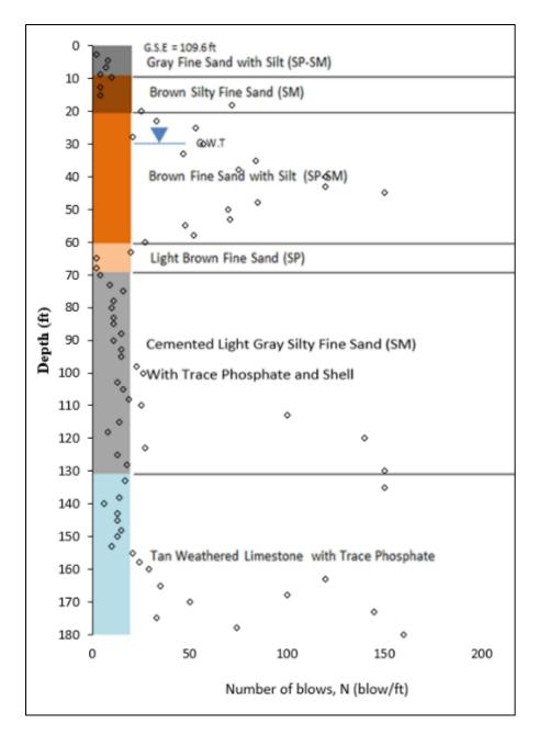
Figure 3-3: General soil profile with USCS classification and the actual number of blows (N) from SPT borings B-39, B-40, and B-41 for I-4/US 192 Interchange
