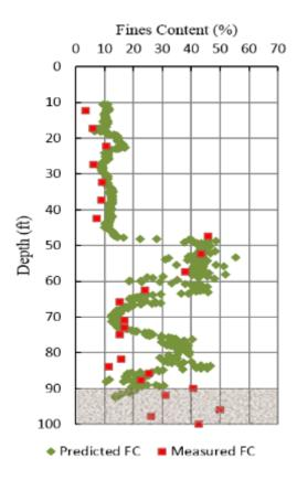
Figure 4-38 for Predicted and measured fines content versus depth for the Anderson Street overpass at pier 6/pile 5, 6 with HPR zone shaded
