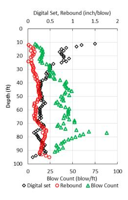
Figure 3-17: Digital set, pile rebound, and  $N_{PD}$  versus depth for pier 2/pile 5 at Ramp B of I-4 / SR 408
