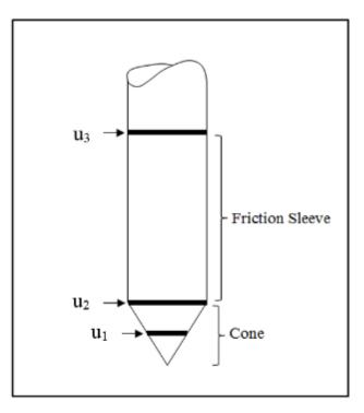
Figure 2-29: CPTu Pore pressure transducer positions: at the cone point  $(u_1)$ , behind the cone tip  $(u_2)$ , and on the shaft between the cone and sleeve  $(u_3)$
