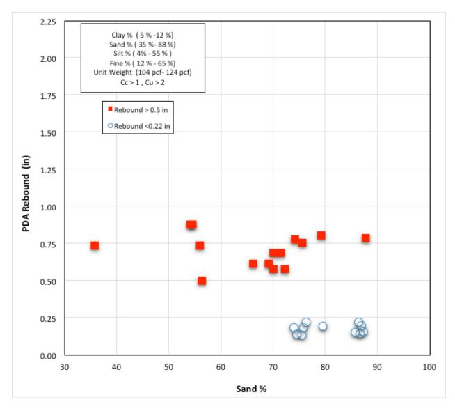
Figure 6.9: Sand Content (%) vs. PDA HPR (in) - cohesionless soils (SM) from all sites
