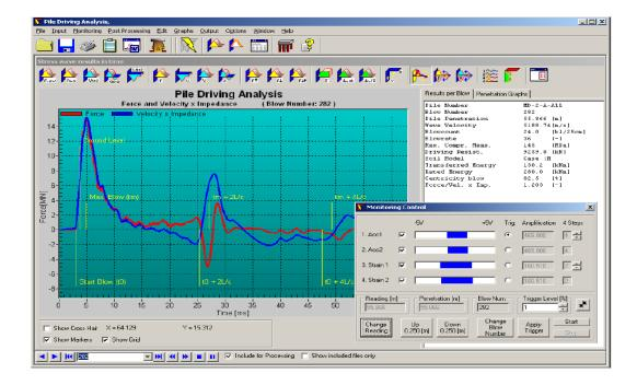
Figure 2-6: PDA output measured force and velocity versus time from a hammer blow (Courtesy of Pile Dynamic, Inc.)
