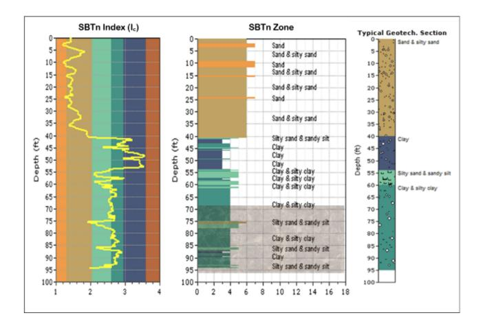
Figure 4-9: Normalized soil behavior type index and typical geotechnical section for I-4/US 192 at Pier 7/pile 10 with HPR zone shaded (GSE = 108.6 ft)
