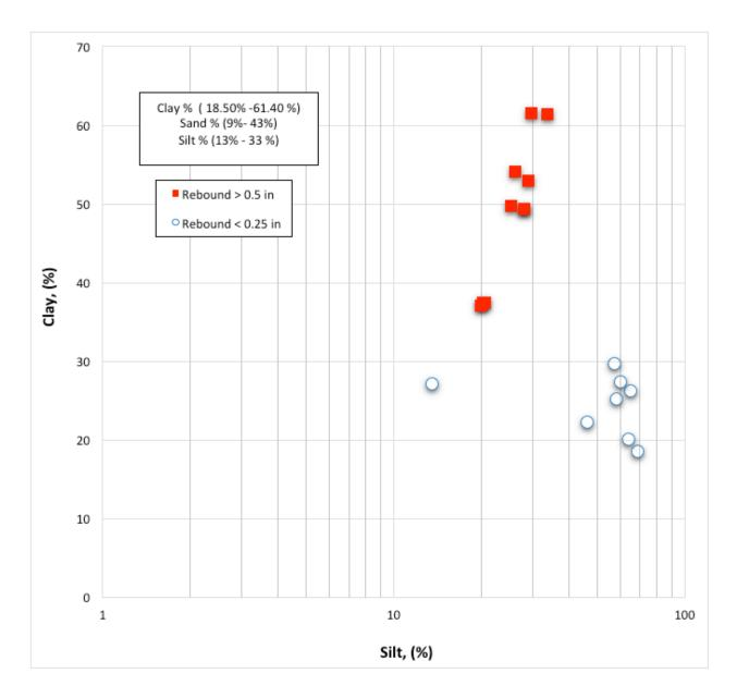
Figure 6.14: Silt content (%) vs. clay content – cohesive soils (CH, CL) from all sites
