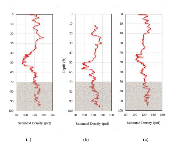
Figure 4-1: Saturated density versus depth for I-4/US 192 at (a) Pier 6/pile 16, (b) Pier 7/pile 10, and (c) Pier 8/pile 4 respectively with HPR zones shaded
