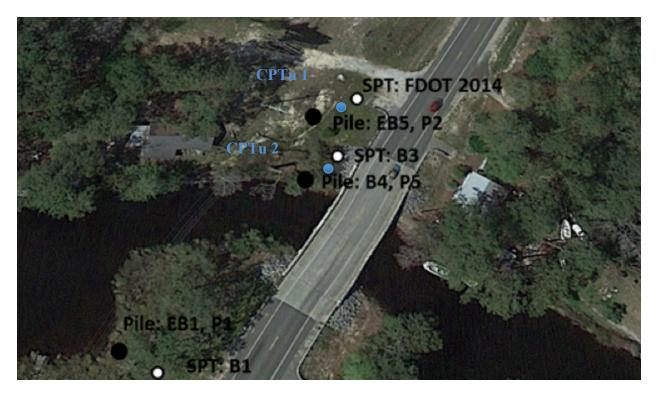
Figure 3-28: Test pile, SPT boring, and CPTu soundings locations for SR 83/Ramsey Branch Bridge
