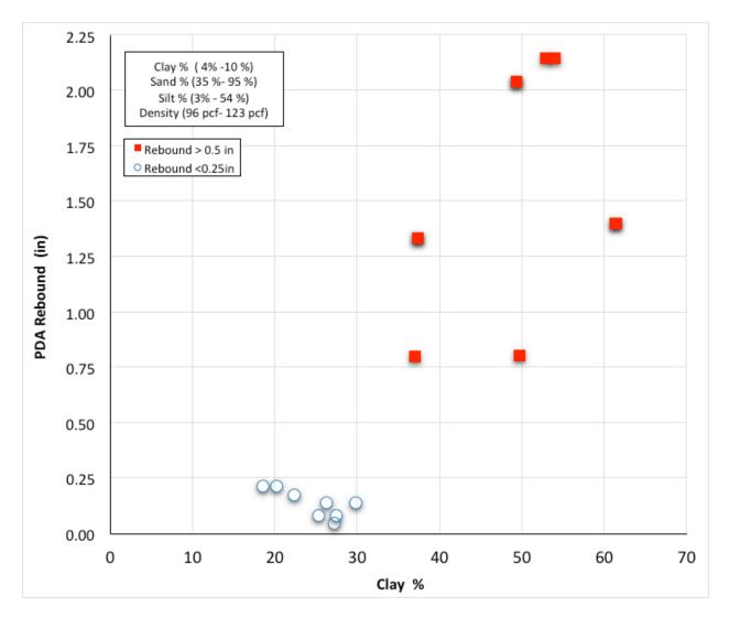
Figure 6.8: Clay content (%) vs. PDA HPR (in) - cohesive soils (CH, CL) from all sites
