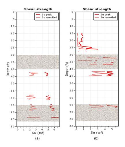
Figure 4-30: Undrained shear strength for SR 83/Ramsey Branch Bridge at EB 5/pile 2 with HPR zones shaded (a) CPT1, (b) CPT2
