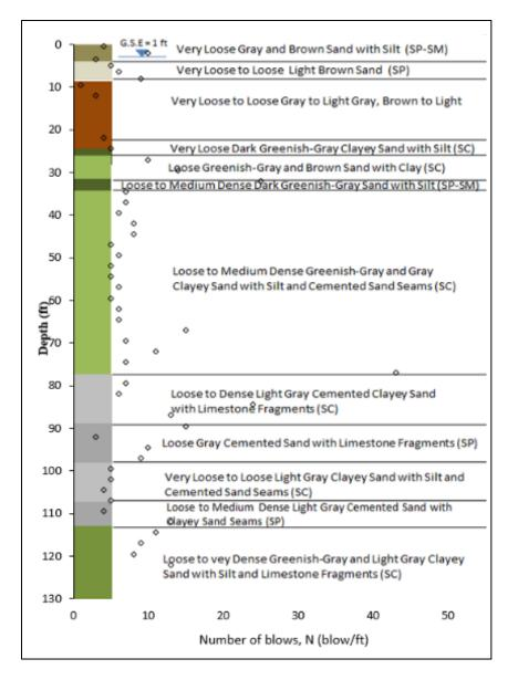
Figure 3-30: General soil profile with USCS classification and the actual N<sub>SPT</sub> from SPT boring B-3 near EB5/pile 2 at SR 83/ Ramsey Branch Bridge
