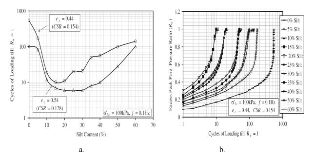
Figure 2-20: Results of cyclic triaxial tests: (a) Silt contents versus cycles required to generate 100% excess pore water pressure; (b) Loading cycles versus excess pore pressure ratio (Dash & Sitharam, 2009)
