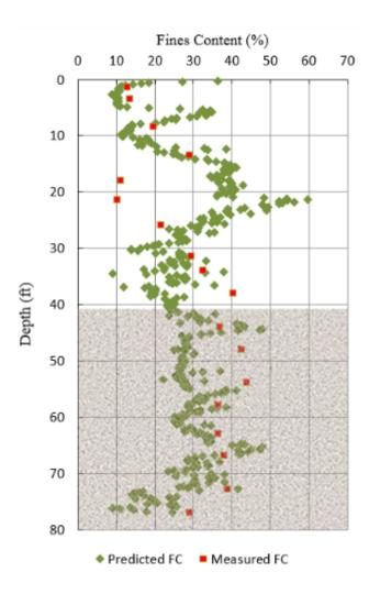
Figure 4-40: Predicted and measured fines content versus depth for SR 83 over Ramsey Branch Bridge at EB 5/pile 2 with HPR zone shaded
