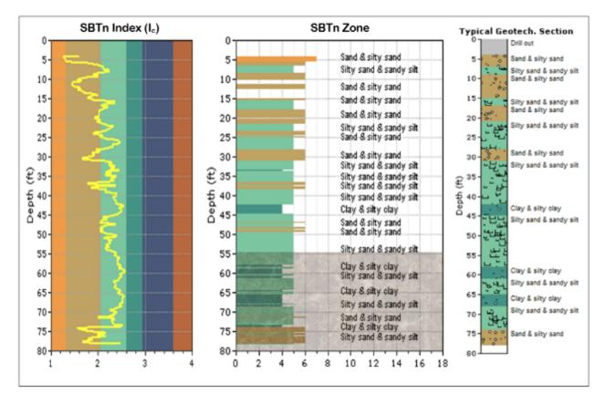
Figure 4-17: Normalized soil behavior type index and typical geotechnical section for SR 83 over Ramsey Branch Bridge at EB 5/pile 2 with HPR zone shaded (GSE = 1.0 ft)
