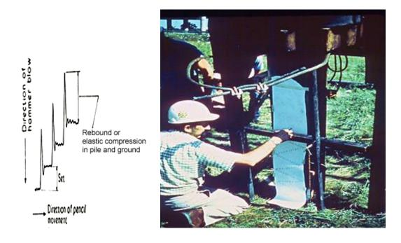
Figure 2-3: Pile displacement and rebound recorded by the manual method (from Hattori 1974, Courtesy of GRL Library)
