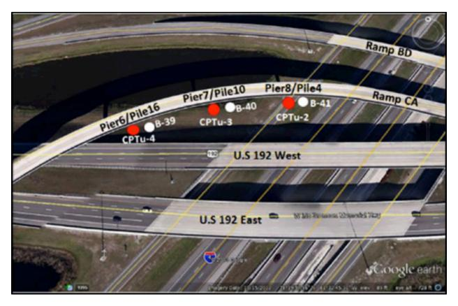
Figure 3-1: Test piles, SPT boring, and CPTu sounding locations for I-4/US-192 interchange
