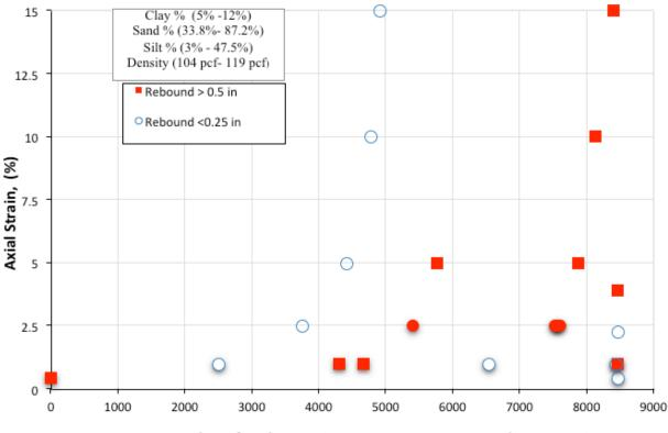
Number of Cycles Causing 0.42, 1, 2.5%, 5%, and 15% Strain
