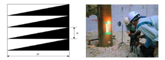
Figure 2-9: Marking paper and line scan camera setup during pile driving (Oliveira et al., 2013)
