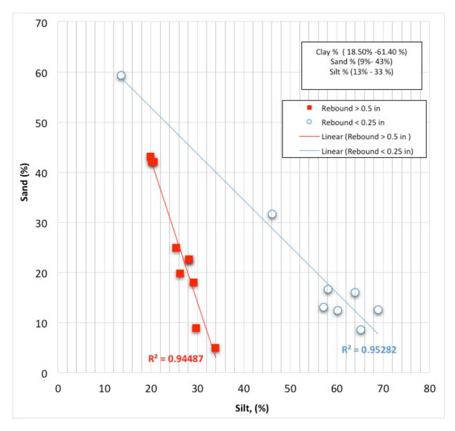
Figure 6.12: Silt Content (%) vs. Sand Content (%) – Cohesive soils (CH, CL) from all sites.
