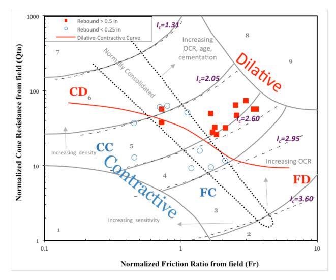
Figure 6.33: Estimated soil behavior based on CPT results matched to HPR and nonHPR laboratory sample elevations on Robertson's (**2012**) updated normalized cone resistance versus friction ratio SBT chart
