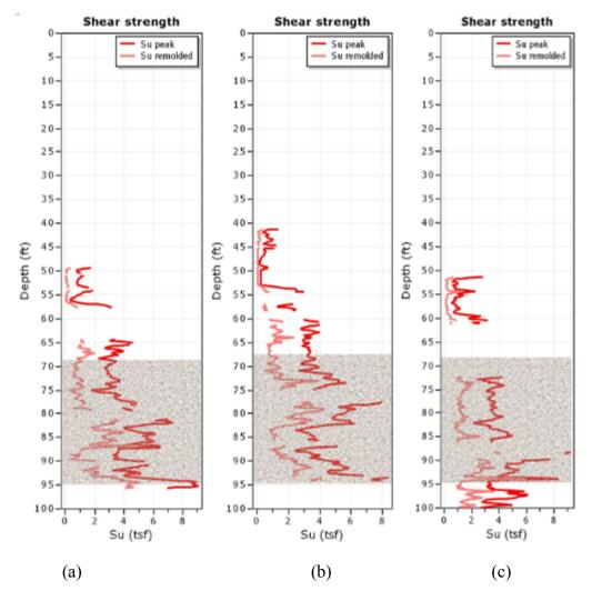
Figure 4-24: Undrained shear strength for I-4/US 192 at (a) pier 6/pile 16, (b) pier 7/pile 10, and (c) pier 8/pile 4 with HPR zones shaded
