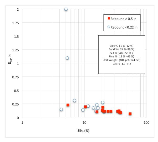
Figure 6.17: Silt content (%) vs. D<sub>60</sub> content – cohesionless soils (SM) from all sites
