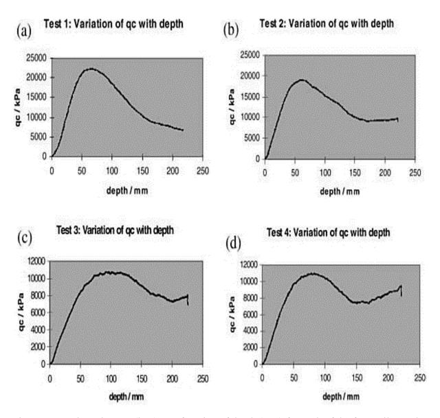
Figure 2-18: Tip resistance (kPa) as a function of depth (mm) for each of the four soil samples (McDowell & Bolton, 2000)
