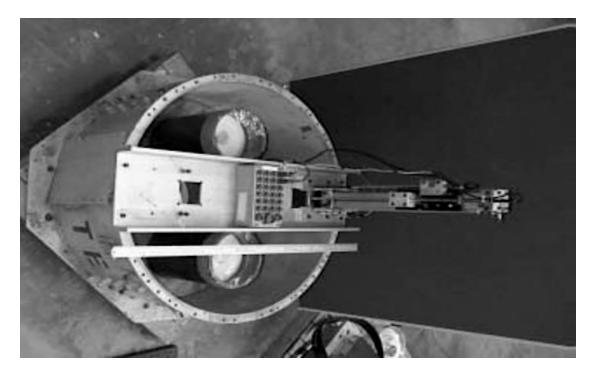
Figure 2-17: Cambridge centrifuge containing the 850 mm diameter steel tub with four190 mm diameter samples (McDowell & Bolton, 2000)
