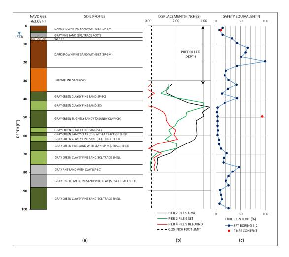
Figure 3-37: (a) Soil Profile, (b) PDA diagram, (c)  $N_{safe}$  and FC for I-10 Chaffee Road Interchange test pile B3 EB 1
