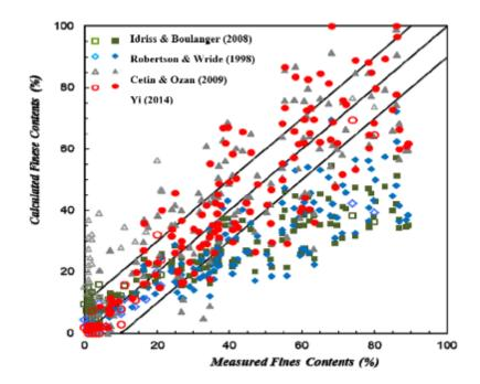
Figure 2-38: Measured versus estimated FC (%) for 95% confidence level (Yi, 2014)
