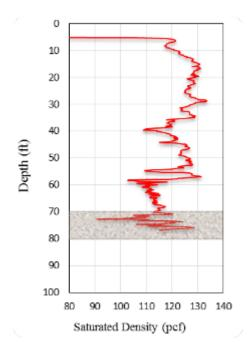
Figure 4-3: Saturated density versus depth for SR 50/SR436 at westbound/pile 5 with HPR zones shaded
