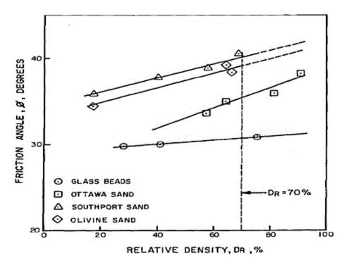
Figure 2-14: Effect of particle shape on angle of internal friction (Holubec & D'Appolonia 1972)
