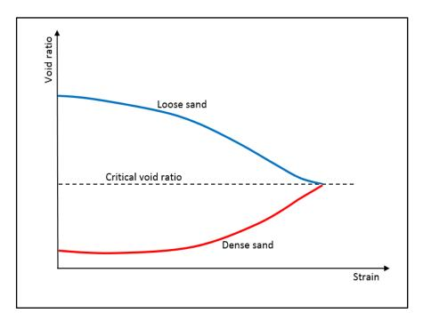
Figure 2-36: Schematic of void ratio versus strain used to determine the state parameter
