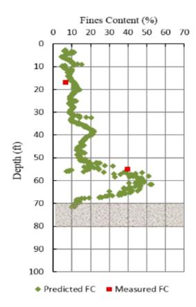
Figure 4-39 for Predicted and measured fines content versus depth for I-4 Widening Daytona at EB 3/pile 5 with HPR zone shaded
