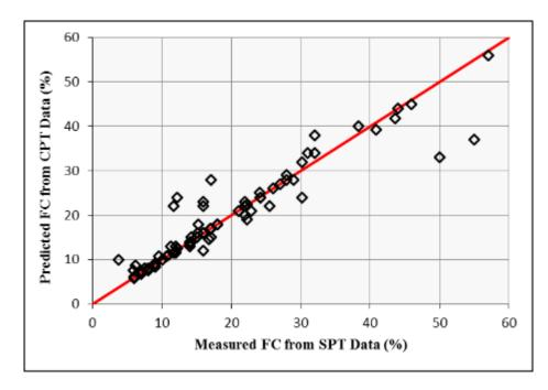
Figure 4-33: Verification of fines content estimation procedure based on 80 data points from all sites
