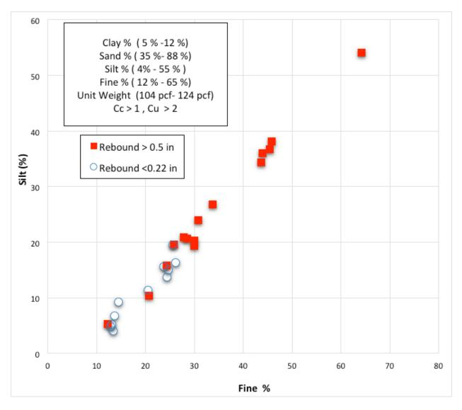
Figure 6.19: Silt content (%) vs. fines content (%) – cohesionless soils (SM) from all sites
