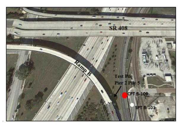
Figure 3-16: Test pile, SPT boring, and CPTu sounding locations for I-4/SR 408 (Ramp B)
