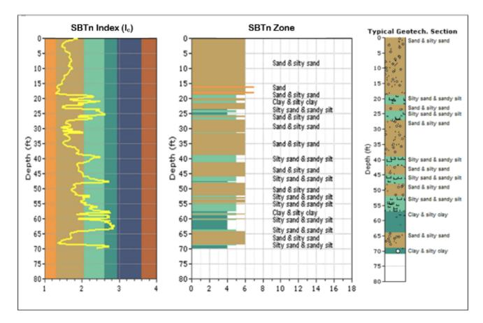
Figure 4-12: Normalized soil behavior type index and typical geotechnical section for SR 417 International Parkway at B2/pile 5 (GSE = 72.3 ft)
