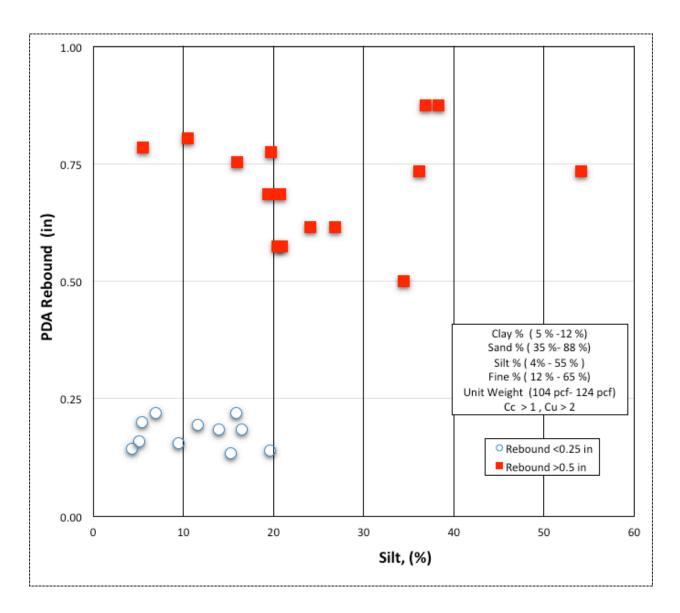
Figure 6.5: Silt content (%) vs. PDA HPR (in) – cohesionless soils (SM) from all sites
