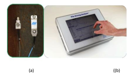
Figure 2-5: (a) PDA Strain Gage and Accelerometers attached to a pile and (b) PDA equipment with CAPWAP<sup>®</sup> (Courtesy of Pile Dynamics, Inc.)
