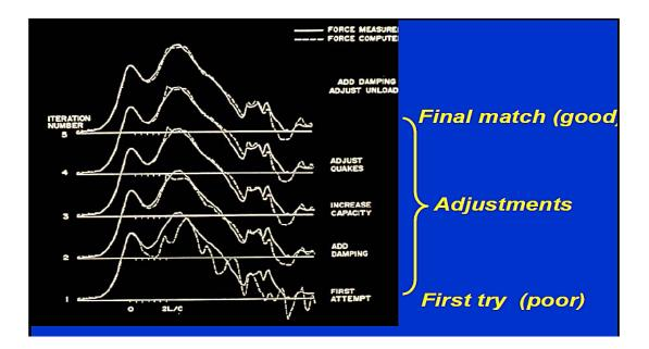
Figure 2-7: CAPWAP<sup>®</sup> iterative process (Courtesy of GRL & Associates)
