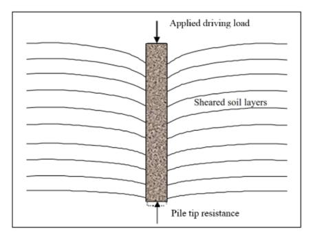
Figure 4-22: Soil layers deformations around a driven pile
