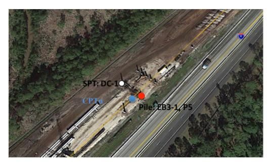
Figure 3-24: Test piles, SPT boring, and CPTu sounding locations for I-4 Widening Daytona
