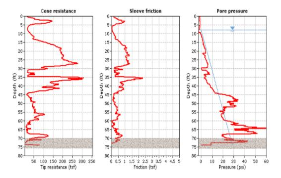
Figure 3-10: CPTu q<sub>c</sub>, f<sub>s</sub>, and u<sub>2</sub> versus depth from CPT-1 near B1/pile 14 at SR 417 International Parkway I-4 Interchange
