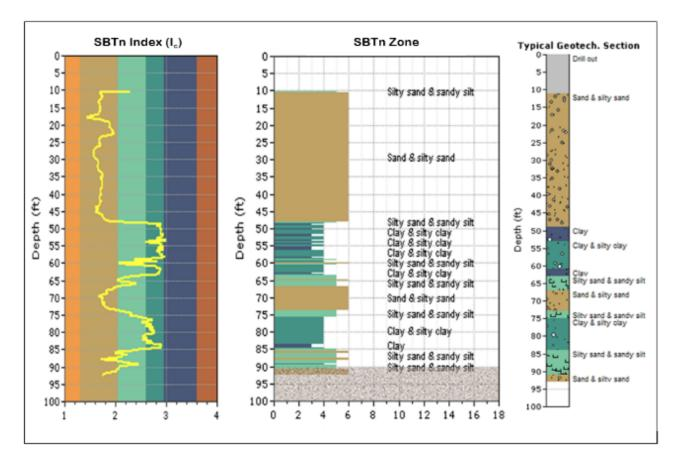
Figure 4-15: Normalized soil behavior type index and typical geotechnical section for Anderson Street overpass at pier 6/pile 5, 6 with HPR zone shaded (GSE = 104 ft)
