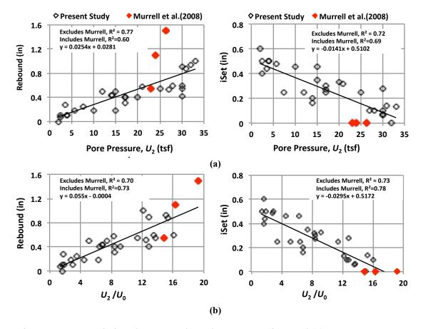
Figure 2-47: Correlations between rebound, permanent-iSet and (a) CPTu pore water pressure, and (b) ratio of CPTu pore pressure  $(u_2)$  and hydrostatic pressure  $(u_0)$  (Cosentino et al., 2013).
