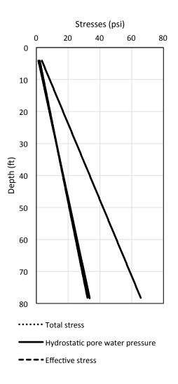
Figure A-7 Total stress, hydrostatic pore water pressure, and effective stress versus depth for SR 83/Ramsey Branch Bridge at EB 5 / pile 2
