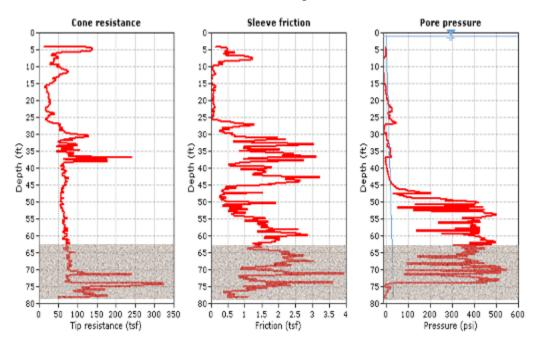
Figure 3-32: CPTu  $q_c$ ,  $f_s$ , and  $u_2$  versus depth from CPT-2 near EB5/pile 2 at SR 83/Ramsey Branch Bridge
