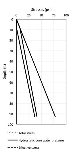
Figure A-4 Total stress, hydrostatic pore water pressure, and effective stress versus depth for I-4 / SR 408 at pier 2 / pile 5
