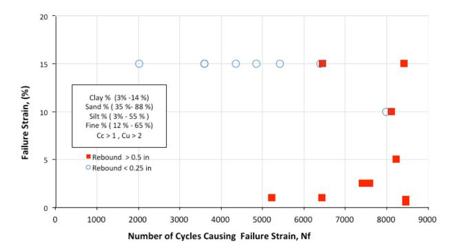
Figure 6.29: Cyclic triaxial failure strain versus number of cycles from cyclic triaxial tests performed on cohesionless HPR and nonHPR soils
