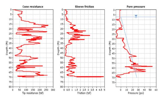
Figure 3-11: CPTu q<sub>c</sub>, f<sub>s</sub>, and u<sub>2</sub> versus depth from CPT-3 near B2/pile 5 at SR 417 International Parkway
