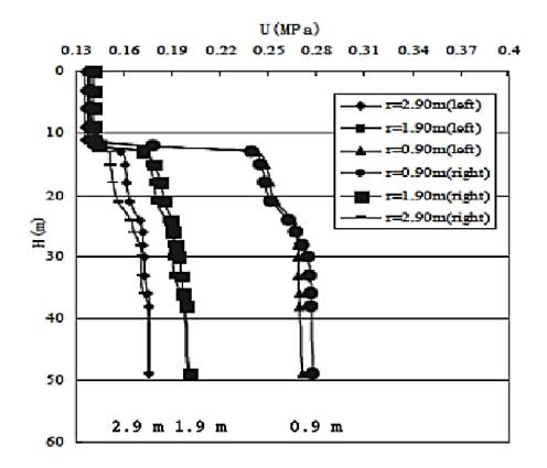
Figure 2-24: Excess pore pressure versus driving depth for the three sensor locations (Bingjian, 2011)
