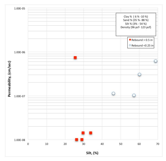
Figure 6.24: Permeability vs. Silt content - Cohesive soils (CH, CL) from all sites
