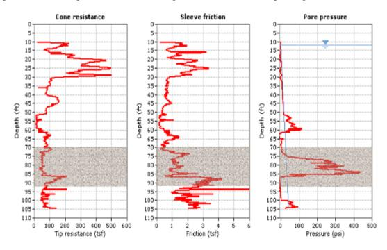
Figure 3-6: CPTu  $q_c$ ,  $f_s$ , and  $u_2$  versus depth from CPTu-2 near pier 8/pile 4 at I-4/US 192
