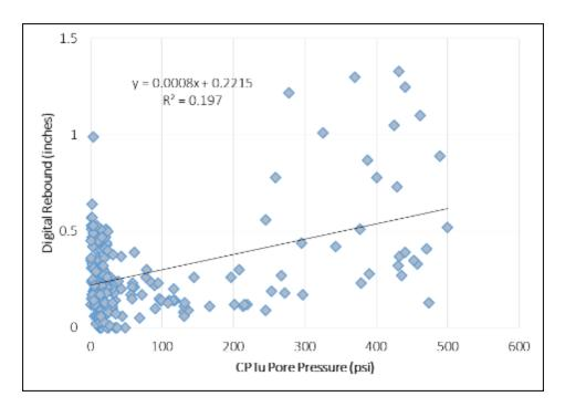
Figure 4-20: Digital Rebound versus CPTu pore pressure from six test sites
