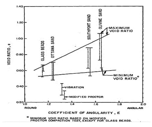
Figure 2-13: Effect of particle shape on minimum and maximum void Ratios (Holubec & D'Appolonia, 1972)
