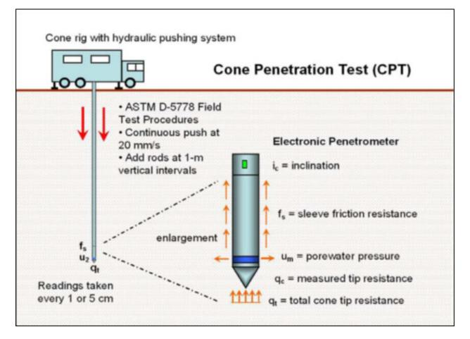
Figure 2-30: Overview of the cone penetration test per ASTM D5778-95
