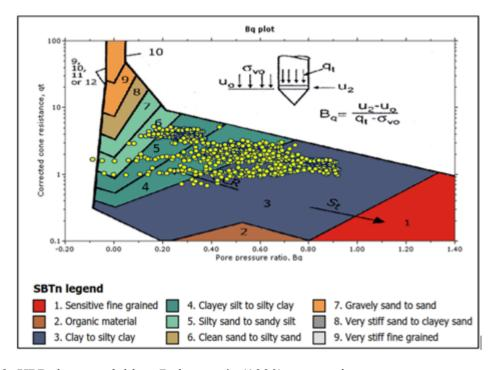
Figure 7.3: HPR data overlaid on Robertson's (1990) cone resistance versus pore pressure ratio SBT chart
