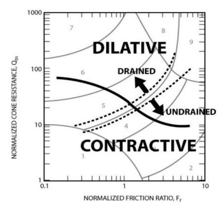
Figure 2-37: Updated normalized cone resistance versus friction ratio SBT chart with soil behavior (Robertson, 2012)
