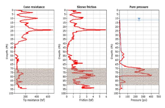
Figure 3-5: CPTu  $q_c$ ,  $f_s$ , and  $u_2$  versus depth from CPTu-3 near pier 7/pile 10 at I-4/US 192
