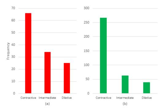
Figure 5.9: Soil predicted reaction to SPT equivalent (N1)60 after Wisnom (2015) for (a) Rebound > 0.50 inches and (b) Rebound < 0.50 inches
