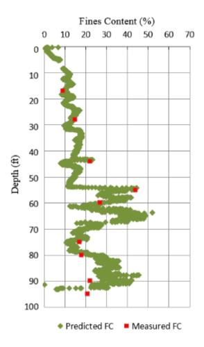
Figure 4-37 for Predicted and measured fines content versus depth for I-4/SR 408 at pier 2/pile 5
