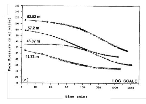
Figure 2-21: CPTu pore pressures dissipation tests at the Alex Fraser Bridge (Robertson et al., 1990)
