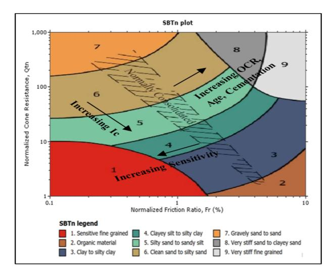
Figure 2-31: Normalized soil behavior type chart (SBTn) based on CPT normalized cone resistance (Q<sub>tn</sub>) and normalized friction ratio (F<sub>r</sub>) (Robertson, 1990)
