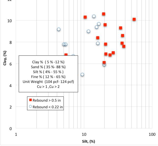
Figure 6.13: Silt content (%) vs. clay content – cohesionless soils (SM) from all sites
