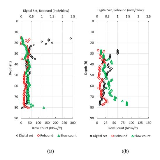
Figure 3-8: Digital set, pile rebound, and N<sub>PD</sub> versus depth for depth for ((a) B1/pile 14 and ((b) B2/pile 5 at SR 417 International Parkway I-4 Interchange
