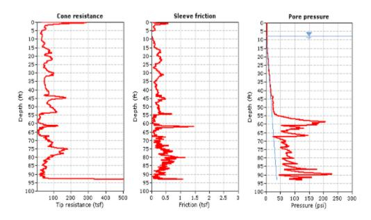
Figure 3-19: CPTu  $q_c$ ,  $f_s$ , and  $u_2$  versus depth from CPT B-109 near pier 2/pile 5 at ramp B of I-4/SR 408
