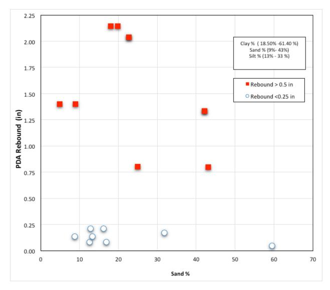
Figure 6.10: Sand content (%) vs. PDA HPR (in) – cohesive soils (CH, CL) from all sites
