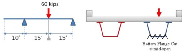
Figure 4-6 Schematic description of the cyclic loading test.
