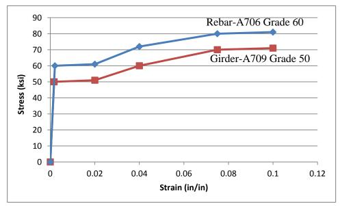
Figure 5-4 Stress-strain behavior of steel girder and rebars.
