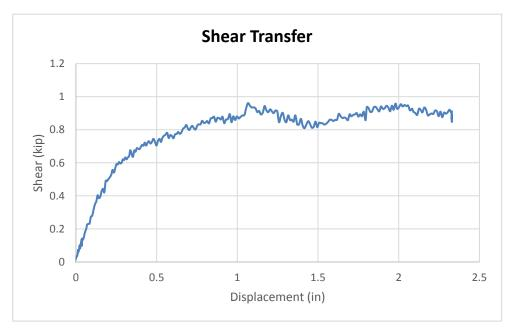
Figure 4-39 Shear transferred through a cross-frame in Test B.
