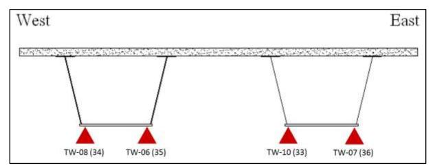
Figure 7-12 Gauge and channel ID of displacement sensors at Location 2.
