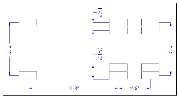
Figure 7-19 Test Truck-2 axle spacing.
