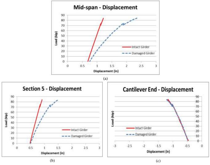
Figure 4-59 Test D: Load vs. displacement curves at (a) mid-span, (b) Section 5 and (c) cantilever end.
