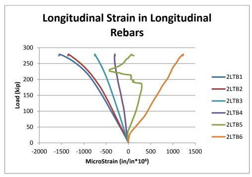
Figure 4-43 Longitudinal strain in rebars at mid-span.
