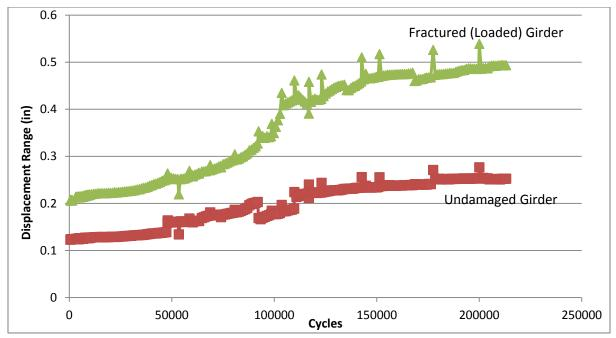
Figure 4-13 Displacement range (max - min) vs. number of loading cycles.
