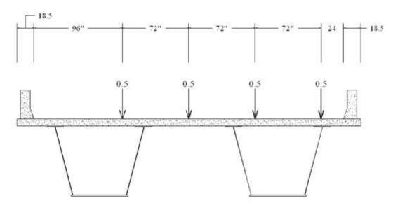
Figure 8-4 Worst case scenario of loading for two trucks with unit weight.
