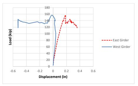
Figure 4-23 Displacement of the both girders near the south support.
