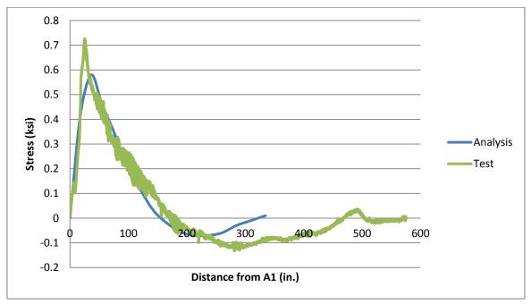
Figure 7-40 Longitudinal stress at 6 ft from north abutment in the west edge of bottom flange of EG: loading scenario-5.
