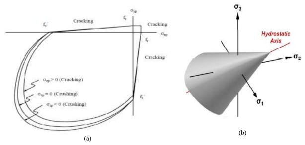
Figure 5-8 Failure surfaces of concrete under (a) biaxial and (b) triaxial loading states (Willam and Warnkle, 1975).
