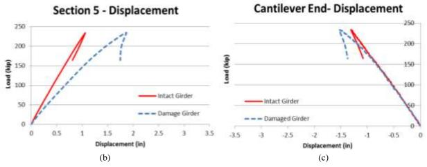
Figure 4-71 Test E: Load vs displacement curves at (a) mid-span, (b) Section 5 and (c) cantilever end.
