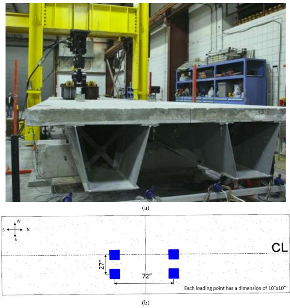
Figure 4-70 (a) Test setup for Test E and (b) schematic locations of loading foot prints.
