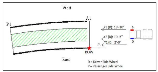
Figure 7-20 Test truck path locations.
