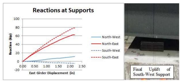
Figure 6-31 Prediction of uplift in finite element analysis.
