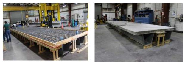
Figure 4-35 The reconstructed specimen before (left) and after casting (right).
