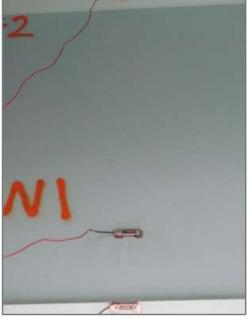
Figure 7-14 Strain transducers on box-girders (typical).
