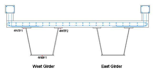
Figure 3-13 Strain gauges in the Section 4.
