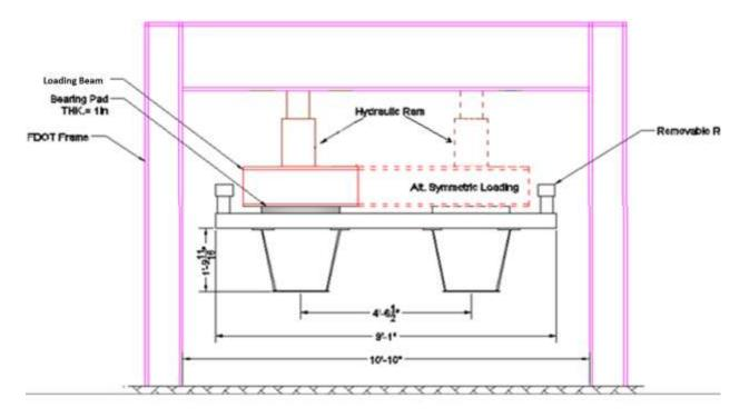
Figure 3-21 Schematic drawing of loading system.
