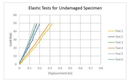
Figure 4-3 Results of elastic tests on undamaged specimen.
