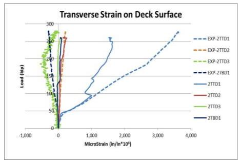
Figure 6-40 Transverse strain on the deck at mid-span.
