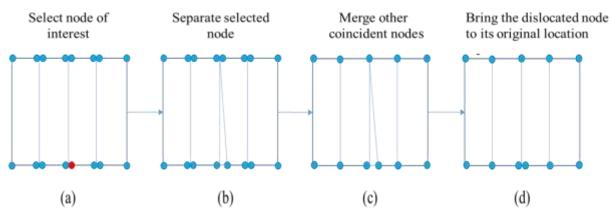
Figure 5-2 Process to simulate a fracture condition.
