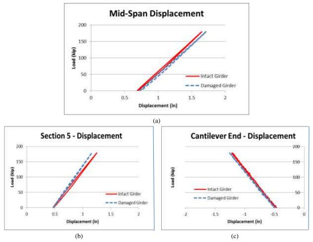
Figure 4-48 Test C: Load vs. displacement curves at (a) mid-span, (b) Section 5 and (c) cantilever end.
