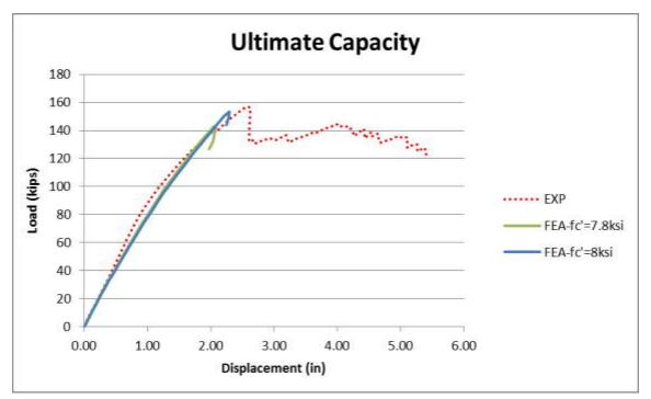
Figure 6-27 Comparison of load vs. vertical deflection curves using displacement-control analysis.
