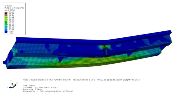
Figure 8-8 Von Mises stresses in single-span bridge under maximum moment, full-web cracked condition.
