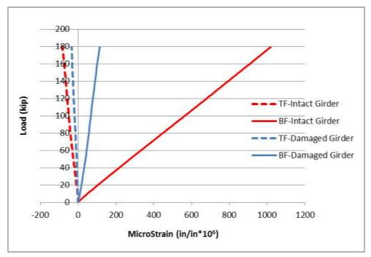
Figure 4-54 Comparison of longitudinal strains in the intact and damaged girders at Section 5.
