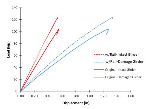
Figure 9-2 Effects of railing system.
