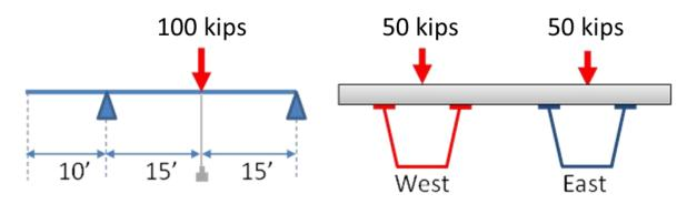
The first test had NNS characteristics. Figure 6-1 provides a schematic description of the test.
