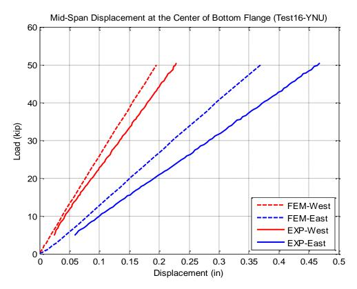
Figure 6-22 Comparison of vertical displacement at the bottom flange of each girder in Test 16.
