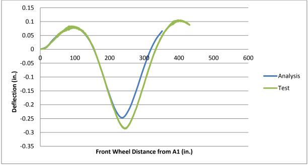
Figure 7-28 Vertical deflection of west edge of WG: 225.5 ft from north abutment, Truck-1 on path-3.
