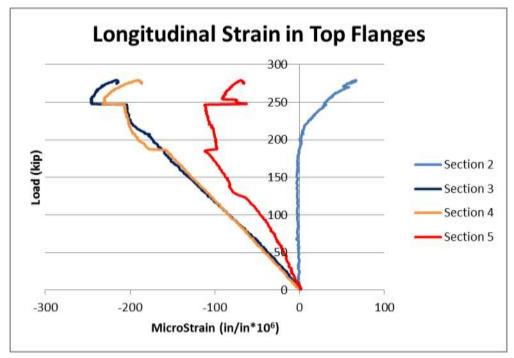
Figure 4-40 Average longitudinal strains at top flanges of the intact girder.
