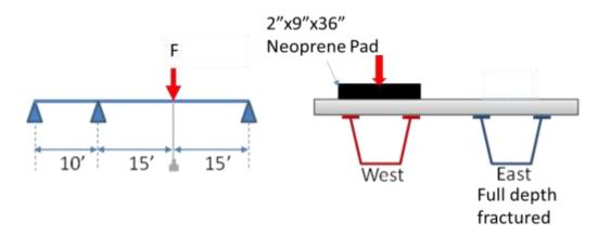
Figure 4-36 Schematic description of Test B.
