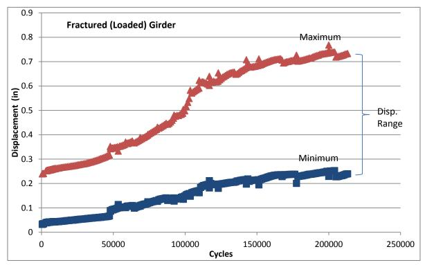
Figure 4-12 Mid-span displacement vs. number of loading cycles in the fractured girder.
