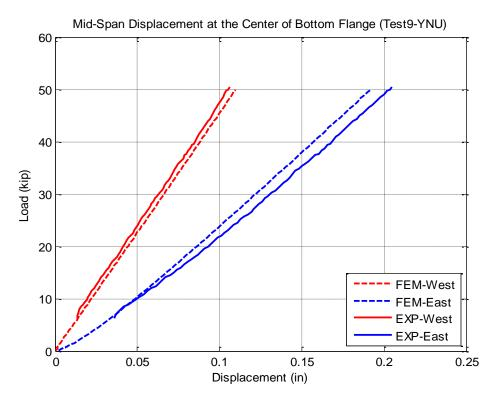
Figure 6-14 Comparison of vertical displacement at the bottom flange of each girder in Test 9.
