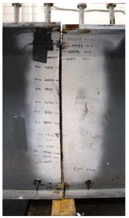
(a) Before aligned Figure 4-34 Alignment of two fractured segments.
