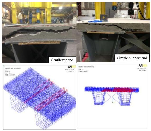
Figure 6-36 Shear cracking in south (left) and north (right) supports.
