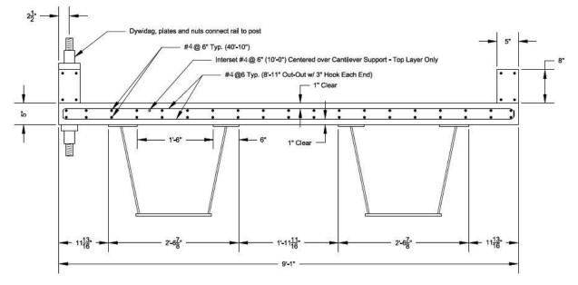
Figure 3-3 Cross-section of the testing specimen.
