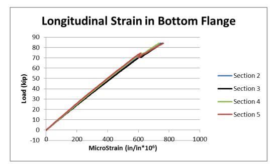
Figure 4-64 Longitudinal strains in bottom flange of the intact girder at Sections 2, 3, 4, and 5.
