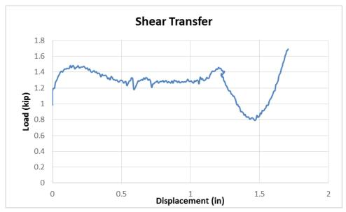
Figure 4-62 Shear transferred through a cross-frame in Test C.
