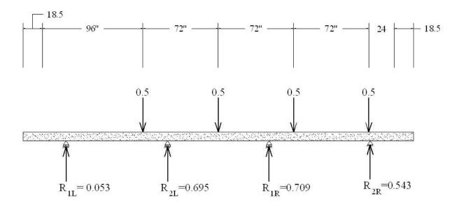
Figure 8-5 Web reactions due to application of two trucks with unit weight.
