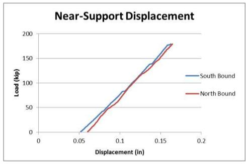
Figure 4-50 Near-support displacement.
