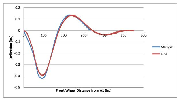
Figure 7-31 Vertical deflection of west edge of EG: 59 ft from north abutment, Truck-1 followed by Truck-2 on path-1.
