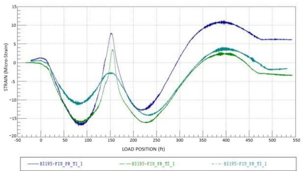
Figure 7-24 Example of variable thermal drift observed during testing.
