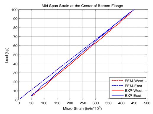
Figure 6-3 Comparison of longitudinal strain at the bottom flange of each girder in Test 1.
