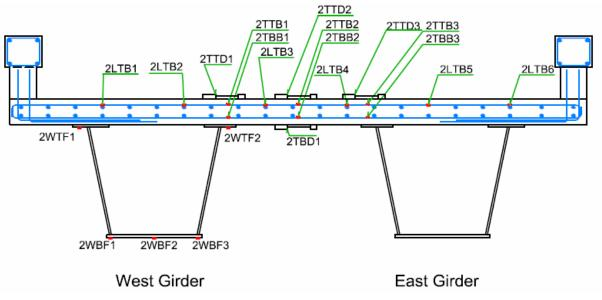
Figure 3-11 Strain gauges in the Section 2.
