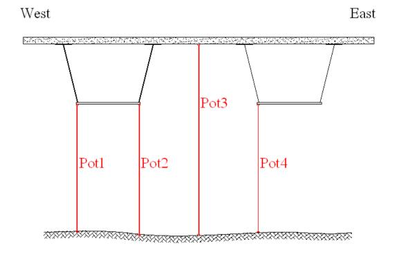
Figure 7-7 Arrangement of potentiometers at Location 1 in the first span.
