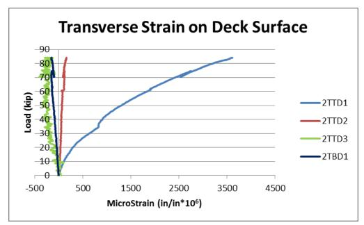
Figure 4-68 Transverse strain on the deck near mid-span.
