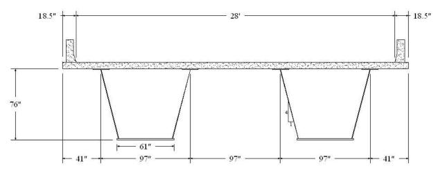
Figure 7-4 Cross-section of the Ft. Lauderdale bridge 860600.
