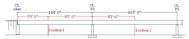
Figure 7-6 Locations of potentiometers in the first two spans.
