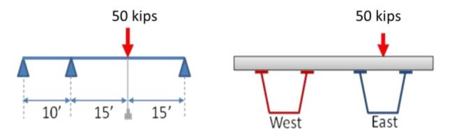
Figure 6-9 Schematic description of Test 3.
