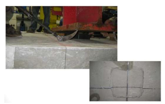
Figure 4-49 Punching damage in test C.
