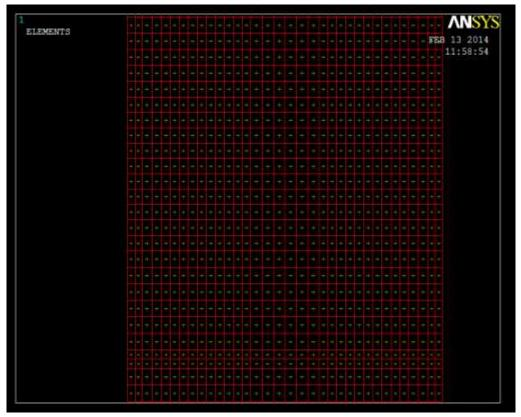
Figure 5-7 Smeared reinforcement bars.
