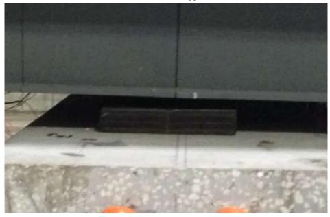
(b) South support Figure 4-25 Uplift at (a) north support and (b) south support.
