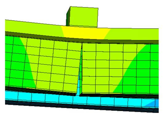
Figure 5-3 Finite element model with full-web fracture condition.
