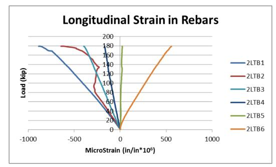
Figure 4-55 Longitudinal strain in rebars at mid-span.
