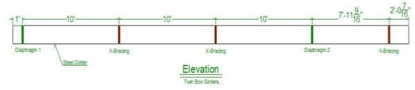
Figure 3-4 Internal bracing locations in each box girder.
