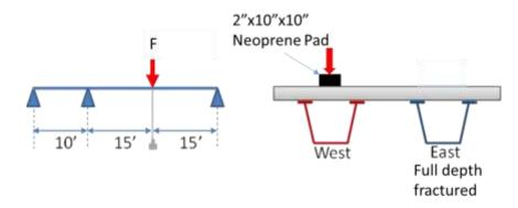
Figure 4-47 Schematic description of Test C.
