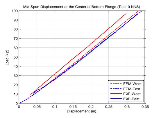
Figure 6-18 Comparison of vertical displacement at the bottom flange of each girder in Test 10.
