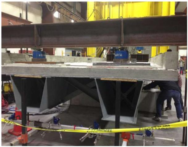
Figure 3-20 Setup for continuity effect.
