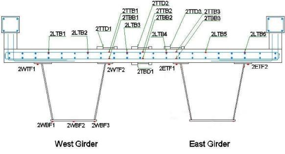
Figure 4-26 Strain gauges at the mid-span section.
