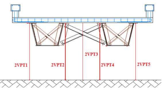
Figure 3-18 Potentiometers in Section 2.
