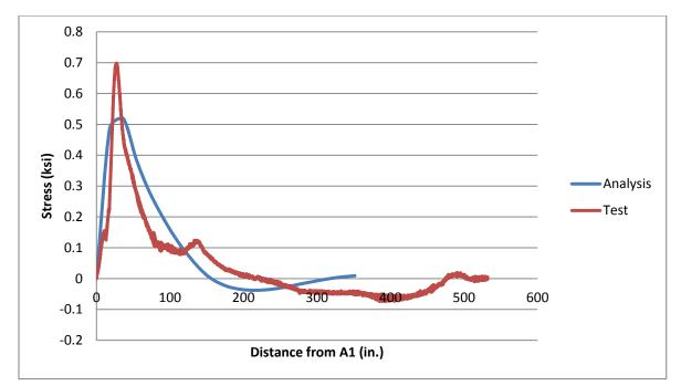
Figure 7-33 Longitudinal stress at 6 ft from north abutment in the west edge of bottom flange of WG: Truck-1 on Path-3.
