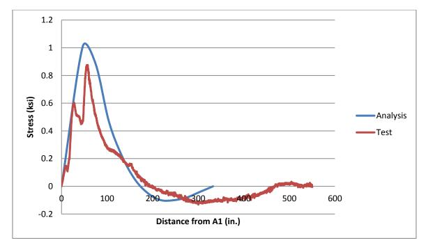
Figure 7-45 Longitudinal stress at 6 ft from north abutment in the west edge of bottom flange of EG - Truck-1 followed by Truck-2 on path-1.
