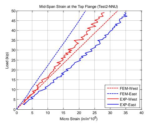
Figure 6-8 Comparison of longitudinal strain at the top flange of each girder in Test 2.
