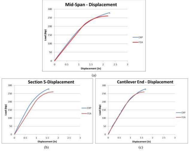
Figure 6-38 Load vs average vertical displacements at (a) mid-span, (b) Section 5, and (c) cantilever end.
