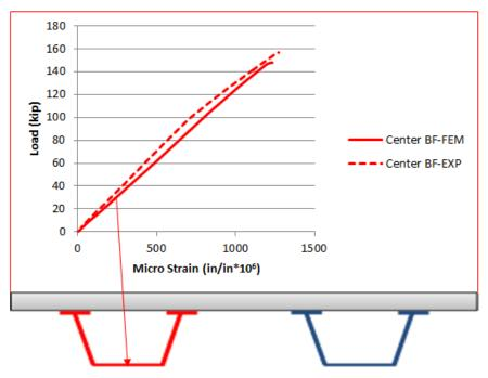
Figure 6-33 Comparison of longitudinal strain at bottom flange at mid-span.
