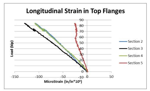
Figure 4-63 Average longitudinal strains at top flanges of the intact girder.
