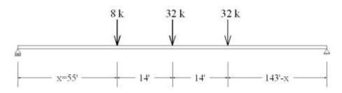
Figure 8-6 Position of the HS-20 truck for maximum moment in girders.
