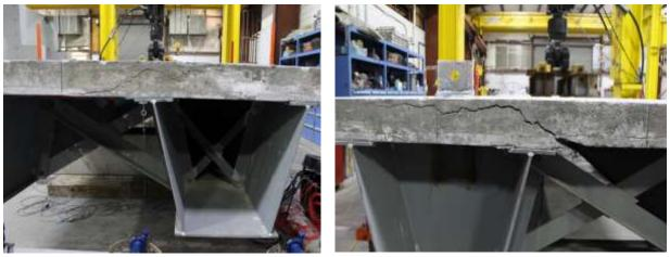
(a) Figure 4-73 Shear damage at ends in Test E.
