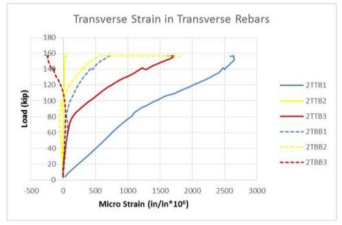
Figure 4-29 Strains of the transverse rebar at mid-span.
