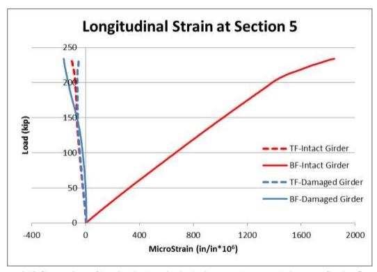
Figure 4-78 Comparison of longitudinal strains in the intact and damaged girders at Section 5.
