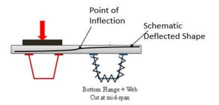
Figure 4-45 Schematic deflection shape of the deck.
