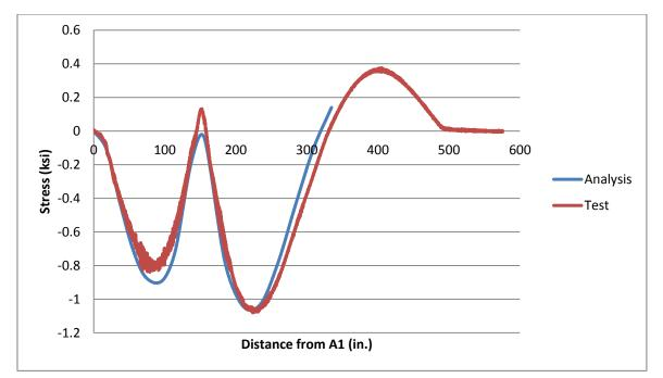
Figure 7-43 Longitudinal stress at 138 ft from north abutment in the west edge of bottom flange of WG: loading scenario-5.
