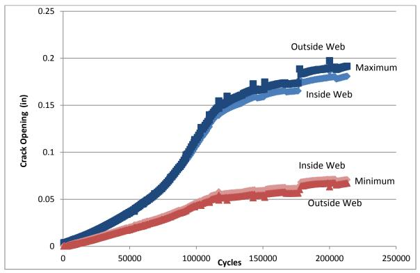
Figure 4-11 Crack base opening vs. number of loading cycles.
