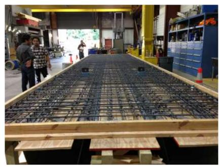
Figure 3-8 Complete specimen ready for casting.
