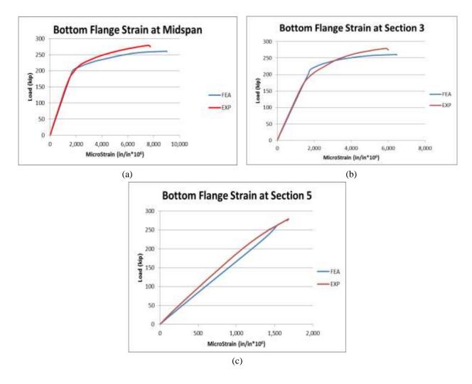
Figure 6-39 Comparison of longitudinal strains at the bottom flange of the intact girder at (a) mid-span, (b) Section 3, and (c) Section 5.
