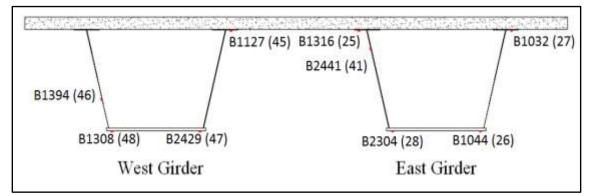
Figure 7-15 Gauge and channel ID's of strain gauges at Section 1.
