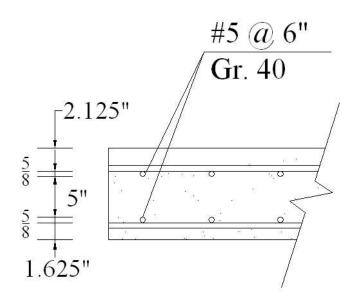
Figure 8-2 Rebar layout in concrete slab.  $f'_c = 4.5 \text{ ksi}$
