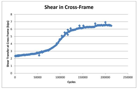
Figure 4-16 Maximum shear transfer in one cross-frame.
