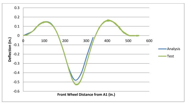
Figure 7-32 Vertical deflection of east edge of EG: 225.5 ft from north abutment, Truck-1 followed by Truck-2 on path-1.
