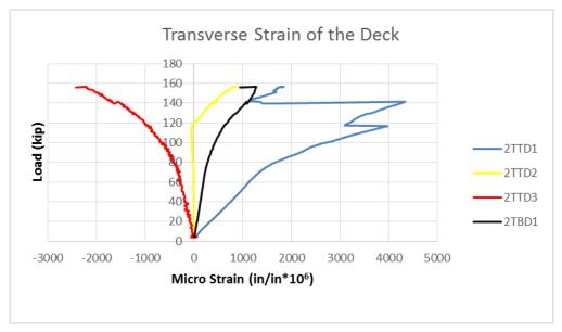
Figure 4-31 Transverse strain at the top and bottom of deck at mid-span.
