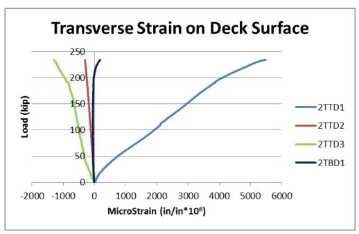
Figure 4-80 Transverse strain on the deck near mid-span.
