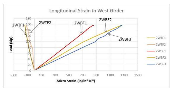
Figure 4-27 Longitudinal strain in the top and bottom flanges of west girder at mid-span.
