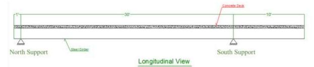
Figure 3-19 Longitudinal view of test specimen.
