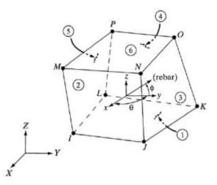
Figure 5-6 Solid65 concrete element in ANSYS.
