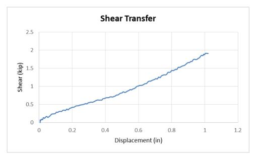
Figure 4-51 Shear transferred through a cross-frame in test C.
