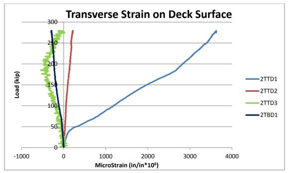
Figure 4-46 Transverse strain of the deck near mid-span.
