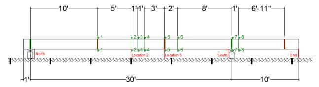
Figure 3-10 Locations of strain gauges and potentiometers along the length of the specimen.
