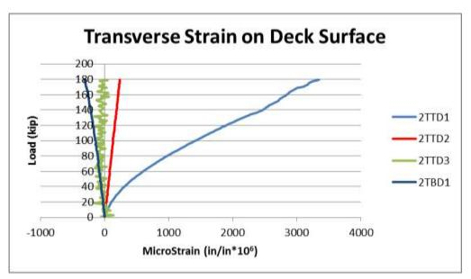
Figure 4-57 Transverse strain on the deck near mid-span.
