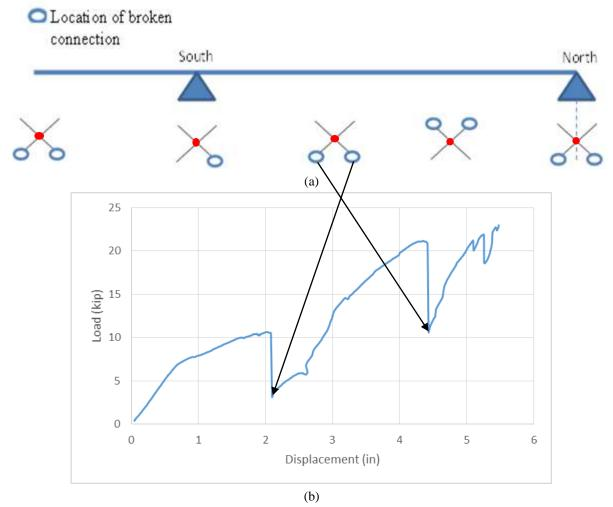
Figure 4-32 Shear transferred through one cross-frame in Test A.
