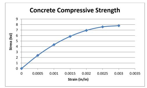
Figure 5-5 Stress-strain curve of concrete in compression.
