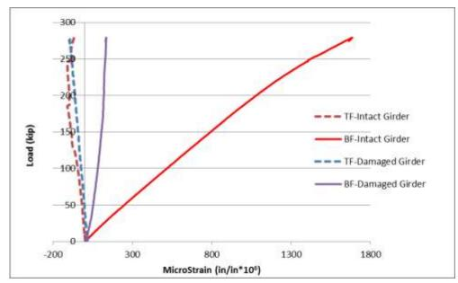
Figure 4-42 Comparison of longitudinal strains in the intact and damaged girders at Section 5.
