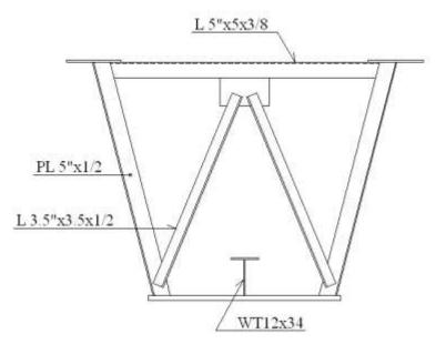
Figure 7-5 Internal bracing of superstructure girders.
