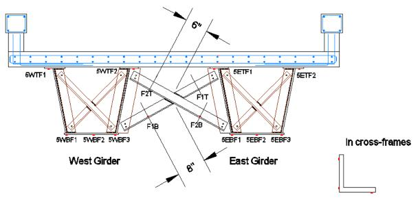
Figure 3-14 Strain gauges in the Section 5.
