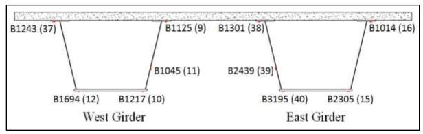
Figure 7-17 Gauge and channel ID's of strain gauges at Section 3.
