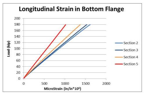
Figure 4-53 Longitudinal strains at the bottom flange of the intact girder.
