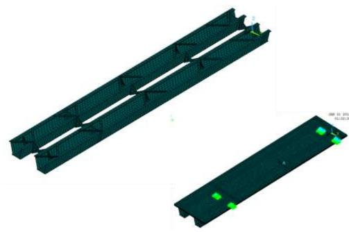
Figure 5-1 Finite element bridge model.
