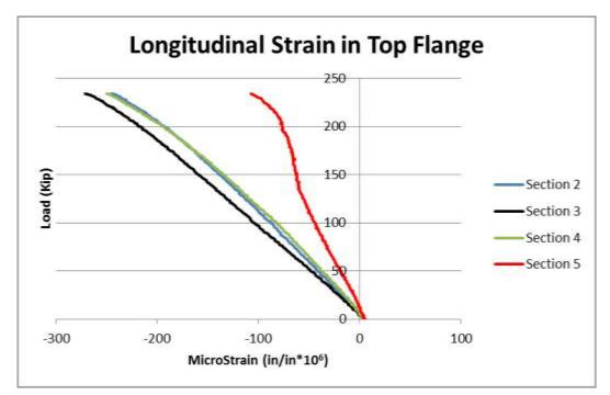
Figure 4-76 Average longitudinal strains at top flanges of the intact girder.
