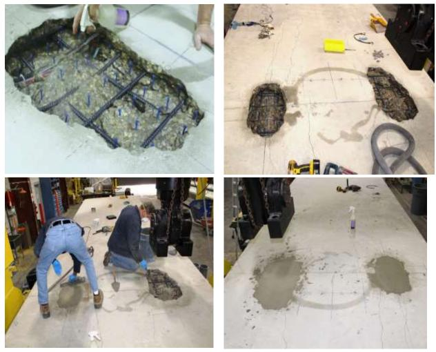
Figure 4-69 Repair of punching shear damage from Tests C and D.
