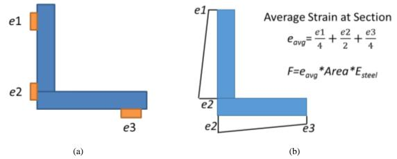
Figure 4-15 (a) Strain locations and (b) Strain profile in each cross-frame brace.
