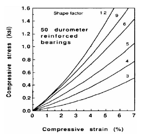
Figure 5-9 Typical stress-strain curve for steel-reinforced bearings (AASHTO-C14.7.6.3.3-1).
