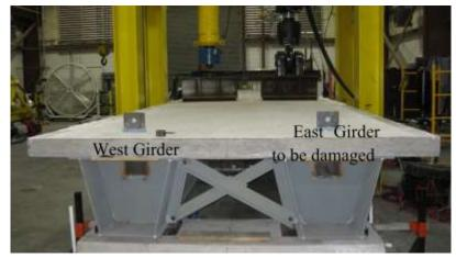
Figure 3-22 Specimen with complete loading setup.
