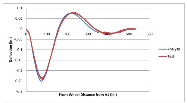
Figure 7-27 Vertical deflection of west edge of WG: 59 ft from north abutment, Truck-1 on path-3.
