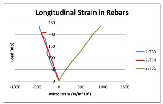
Figure 4-79 Longitudinal strain of rebars at mid-span.
