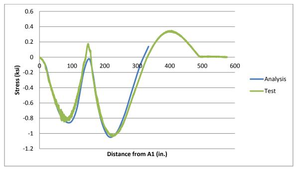
Figure 7-44 Longitudinal stress at 138 ft from north abutment in the east edge of bottom flange of WG: loading scenario-5.
