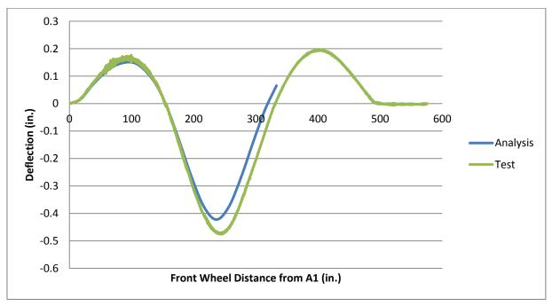
Figure 7-30 Vertical deflection of west edge of WG: 225.5 ft from north abutment, Truck-1 on path-3 and Truck-2 on path-1.
