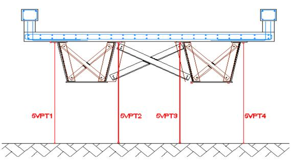
Figure 3-17 Potentiometers in Section 5.
