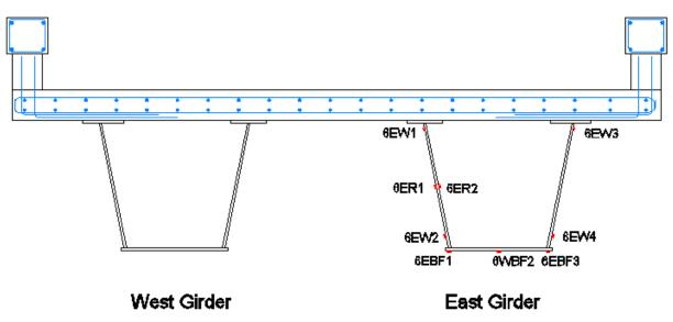
Figure 3-15 Strain gauges in the Section 6.
