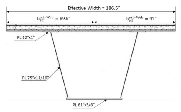
Figure 8-1 Box-girder composite section, Ft Lauderdale bridge.
