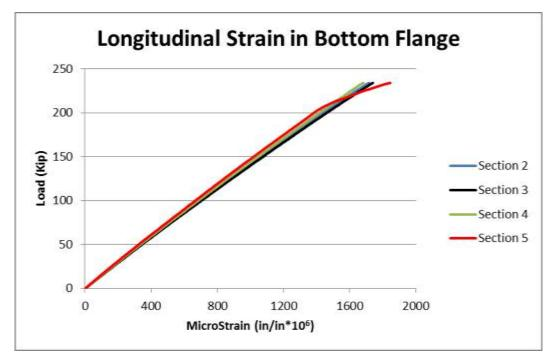
Figure 4-77 Longitudinal strains at the bottom flange of the intact girder.
