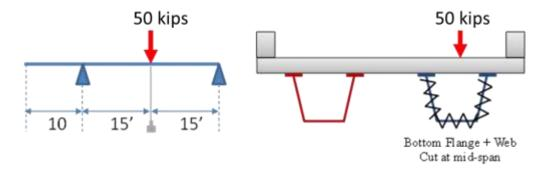
Figure 6-21 Schematic description of Test 16.
