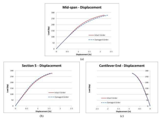
Figure 4-37 Test B: Load vs. displacement curves at (a) mid-span, (b) Section 5 and (c) cantilever end.
