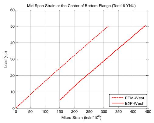
Figure 6-23 Comparison of longitudinal strain at the bottom flange of undamaged Girder in Test 16.
