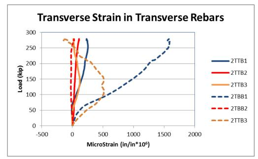
Figure 4-44 Transverse strain in rebars at mid-span.
