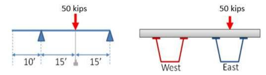
Figure 6-5 Schematic description of Test 2.
