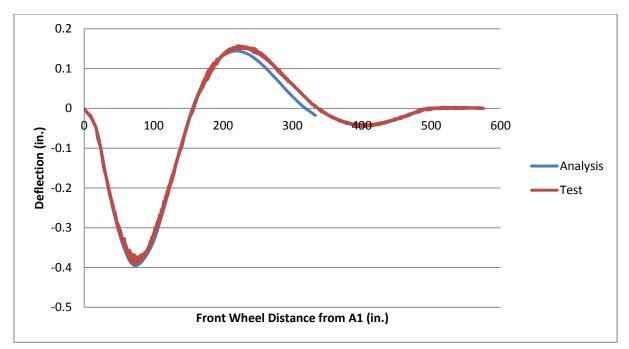
Figure 7-29 Vertical deflection of west edge of EG: 59 ft from north abutment, Truck-1 on path-3 and Truck-2 on path-1.
