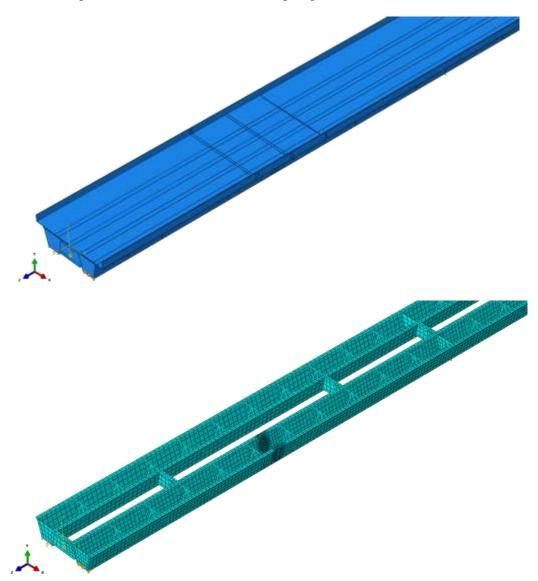
Figure 7-21 Finite element model of the first span of Ft. Lauderdale bridge 860600.
