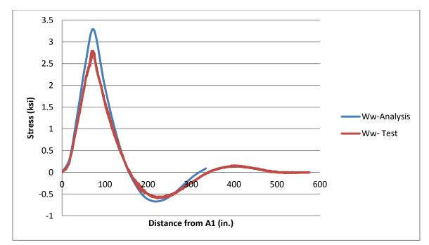
Figure 7-41 Longitudinal stress at 58 ft from north abutment in the west edge of bottom flange of WG: loading scenario-5.
