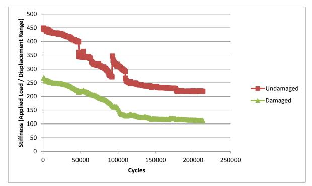
Figure 4-14 Stiffness of each girder during the cyclic test.
