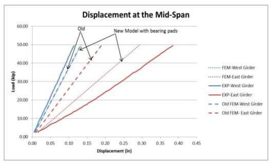
Figure 5-10 Mid-span displacement before and after modeling the bearing pads.
