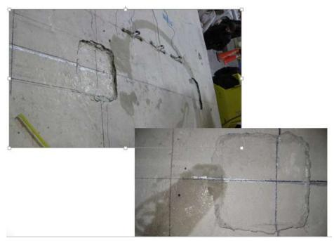
Figure 4-60 Punching damage in Test C.
