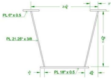
Figure 3-1 Dimension of one steel box girder.
