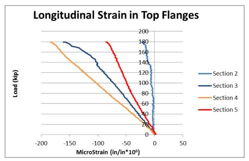
Figure 4-52 Average longitudinal strains at top flanges of the intact girder.
