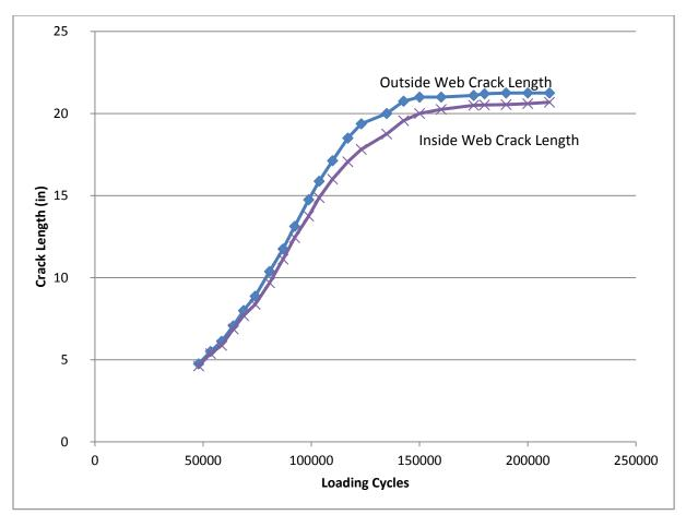
Figure 4-9 Crack growth in the damaged girder.
