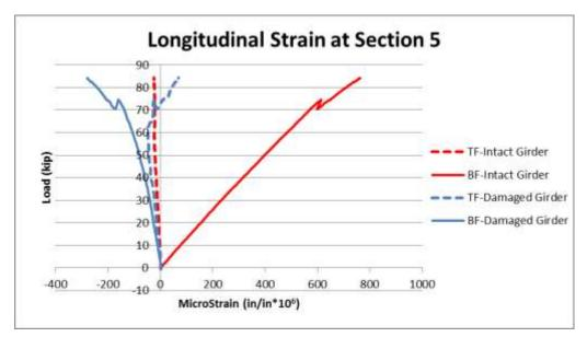
Figure 4-65 Comparison of longitudinal strains in the intact and damaged girders at Section 5.
