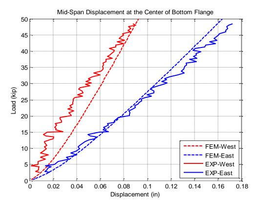
Figure 6-10 Comparison of vertical displacement at the bottom flange of each girder in Test 3.
