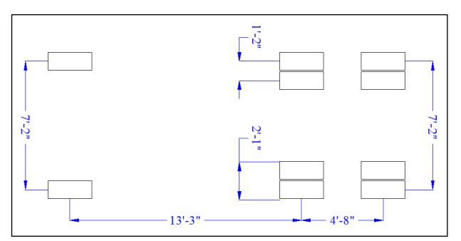
Figure 7-18 Test Truck-1 axle spacing.
