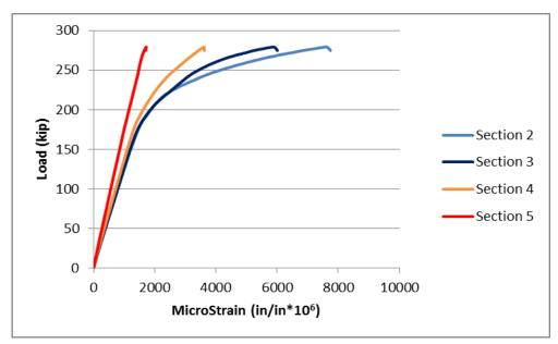
Figure 4-41 Longitudinal strains at the bottom flange of the intact girder.
