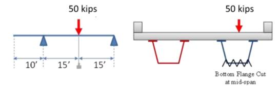
Figure 6-13 Schematic description of Test 9.
