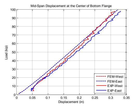
Figure 6-2 Comparison of vertical displacement at the bottom flange of each girder in Test 1.
