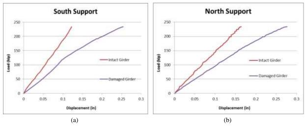
Figure 4-74 Near-support displacement.
