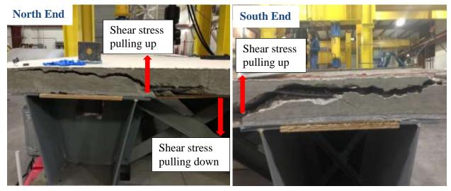
Figure 4-21 Damage at North end (left) and South end (right).
