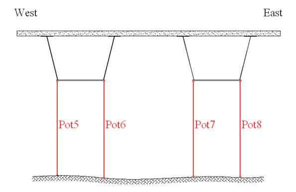
Figure 7-11 Arrangement of the potentiometers at Location 2 in the second span.
