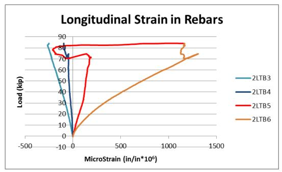
Figure 4-66 Longitudinal strain in rebars at mid-span.
