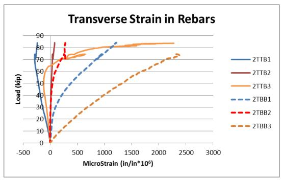
Figure 4-67 Transverse strain in rebars at mid-span.
