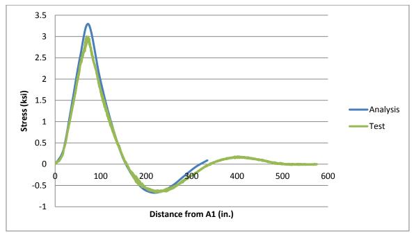
Figure 7-42 Longitudinal stress at 58 ft from north abutment in the east edge of bottom flange of WG: loading scenario-5.
