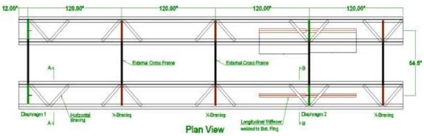
Figure 3-5 The top plan view of the testing specimen.
