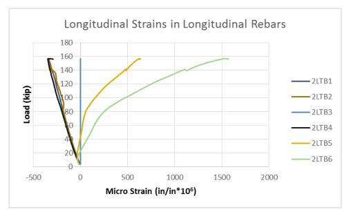
Figure 4-30 Longitudinal strain of rebars in longitudinal direction at mid-span.
