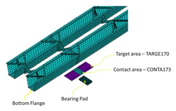
Figure 5-11 Contact surface between the bearing pad and bottom flange of girder.
