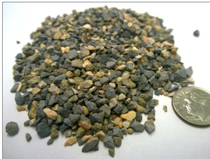
Figure 2.1 – Calcined bauxite, crushed and graded for HFST
