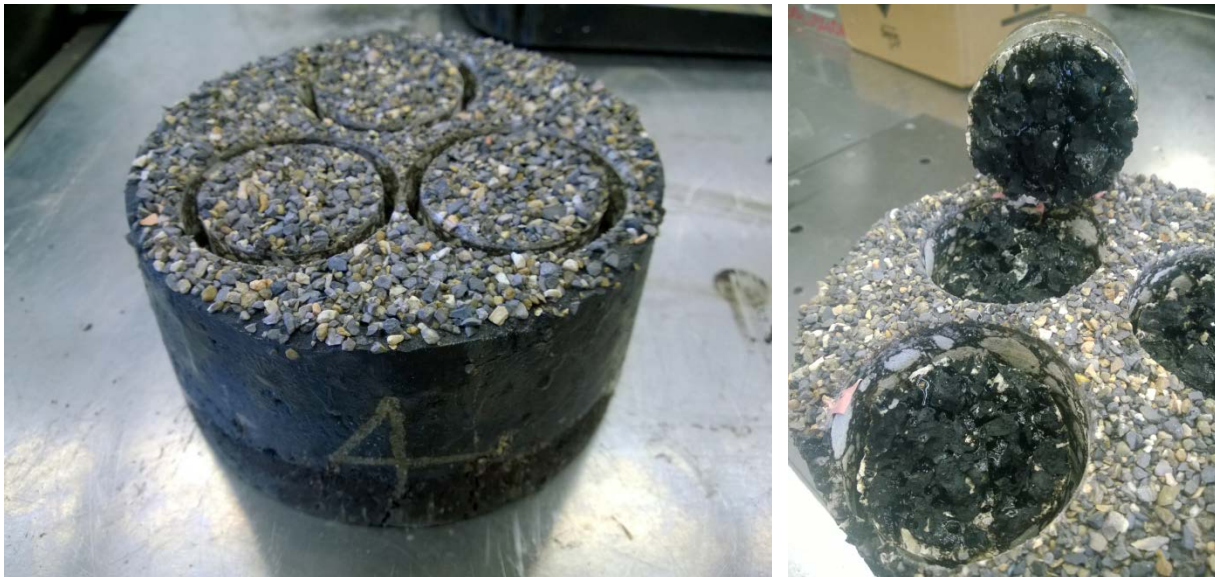
Figure 5.7 – Pull-off tensile strength test
