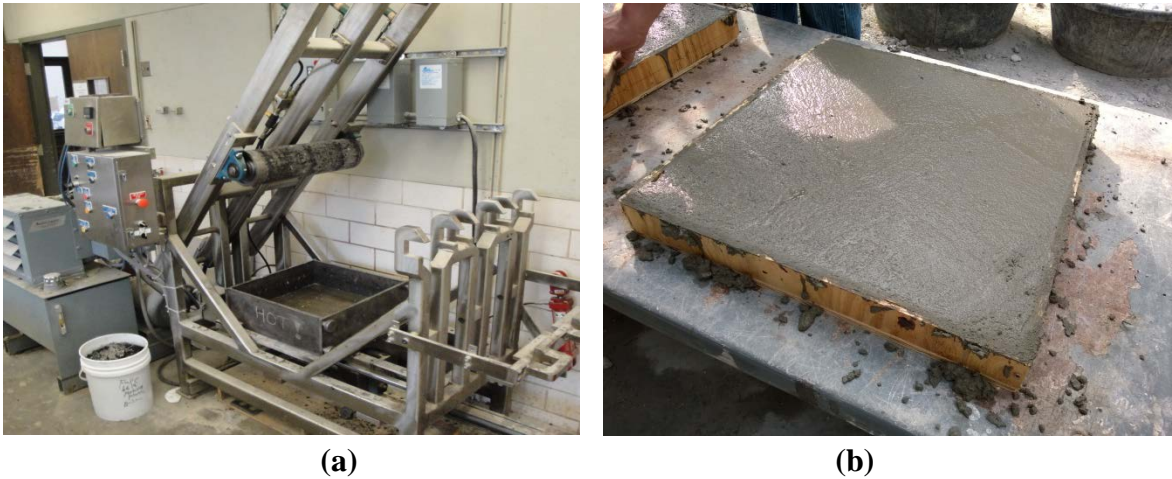
Figure 5.4 – Sample preparation: (a) HMA slab compactor and (b) concrete slab mold
