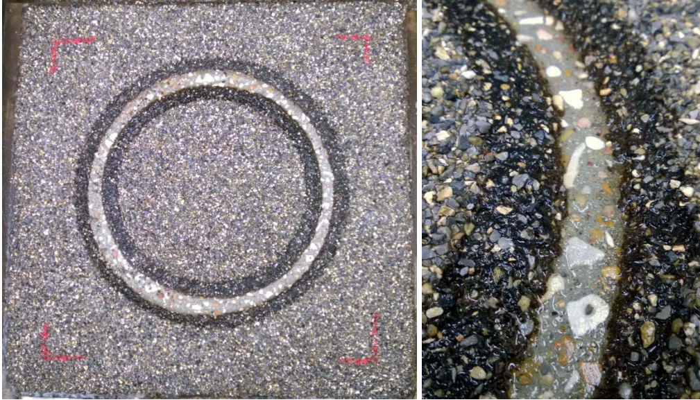
Figure 5.16 – Failure of Binder C sample at 140°F
