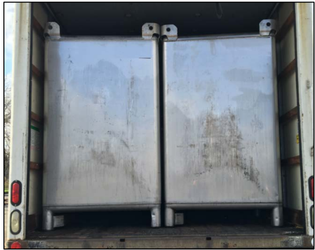
Figure 1. Two 550-gallon IBCs mounted at the rear of a truck. The strap that holds them in place is not shown.
