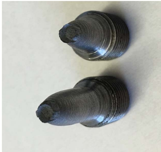
Figure 4: Typical rivet specimen after failure
