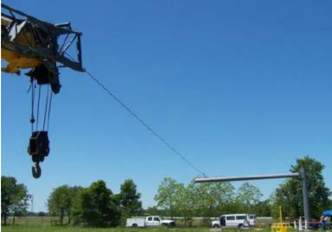
Figure 2.33: Combined torsion and lateral loading ( McVay et al. 2014 )
