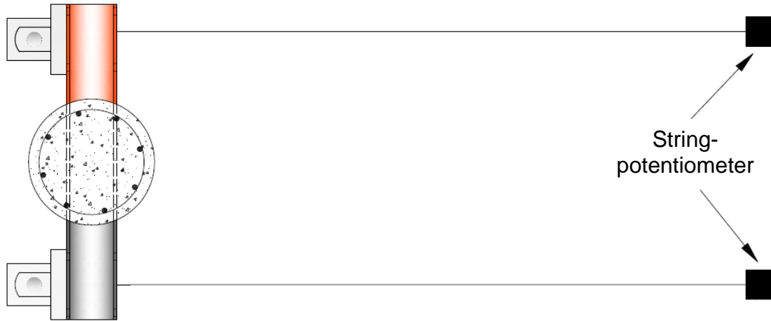
Figure 4.8: Schematic of string-potentiometers arrangement
