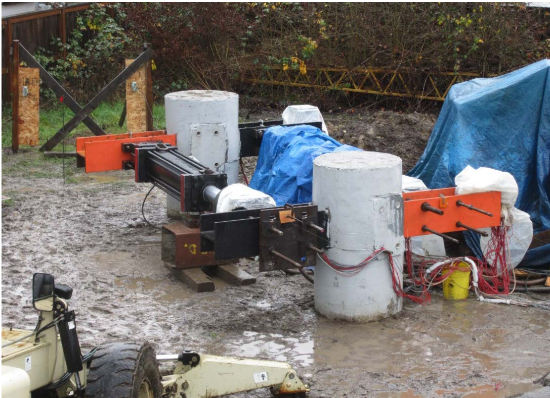
Figure 5.1: Torsional loading test in progress
