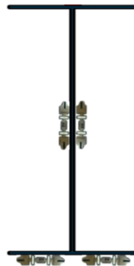
Figure 6.1 – Cross-Sectional View with FBG Sensors on the Web and Bottom Flange
