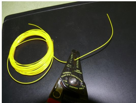
Figure 1.3: Stripping outer coating of optical fiber.
