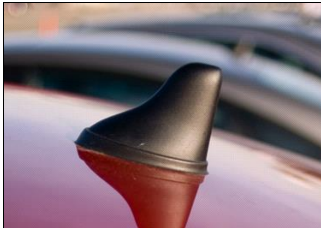
Figure 10. Hirschman shark fin combined DSRC/GPS antenna.
