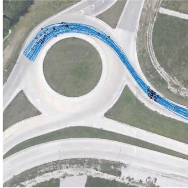
Figure 5.4 Path of center of mass and locations of minimum \Delta v_a and \Delta v_c for sample of drivers on high-speed road (Google Maps).
