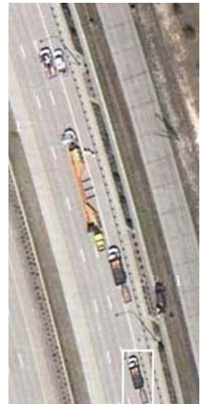
Illustration of In-Lane Barrier Vehicle used with MBT-1
