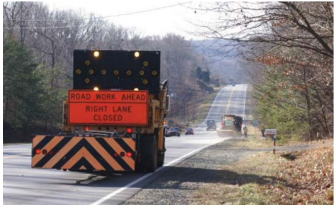
Protective Vehicles with TMAs Provide Rear (Longitudinal) Protection
