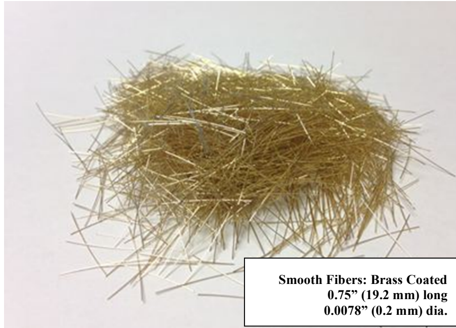
Figure 3-2: Example of the Steel Fibers Used in this Study
