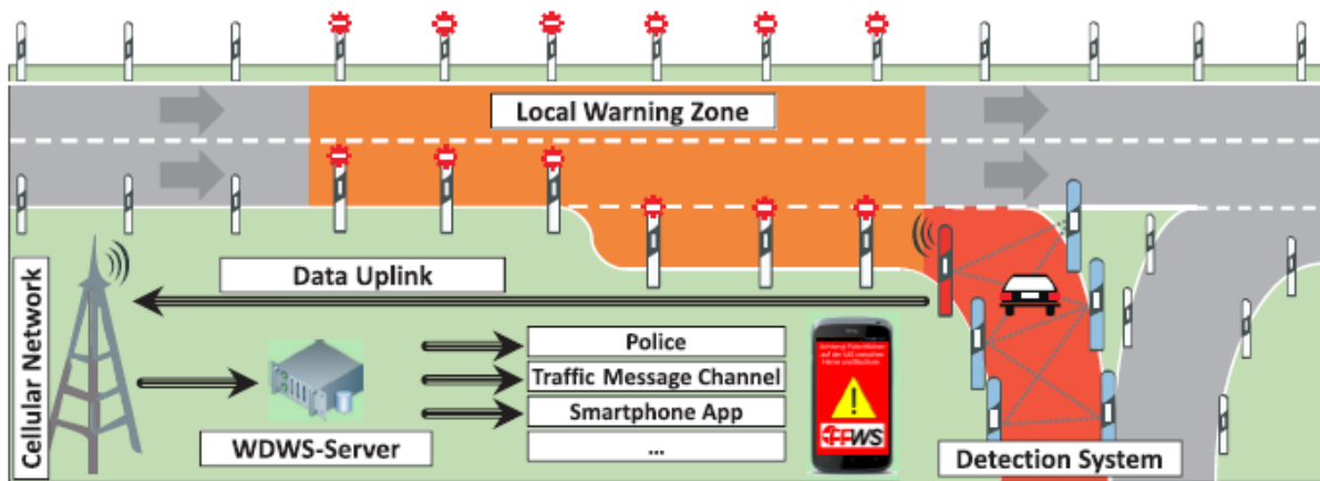
Figure 27. System Architecture of the New Wireless Detection and Warning System for Wrong-Way Drivers (28).
