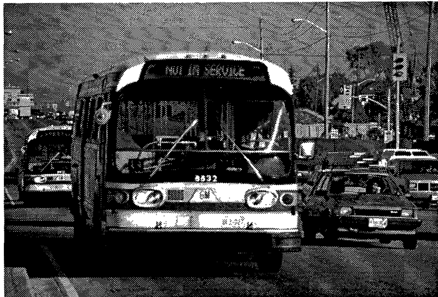
“Dead Heading” buses via HOV lanes can improve fleet utilization during peak periods ( Dufferin St., North York )
