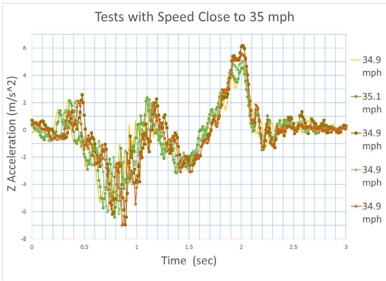
FIGURE 5. Accelerations Measured at Speeds Close to 35 mph.
