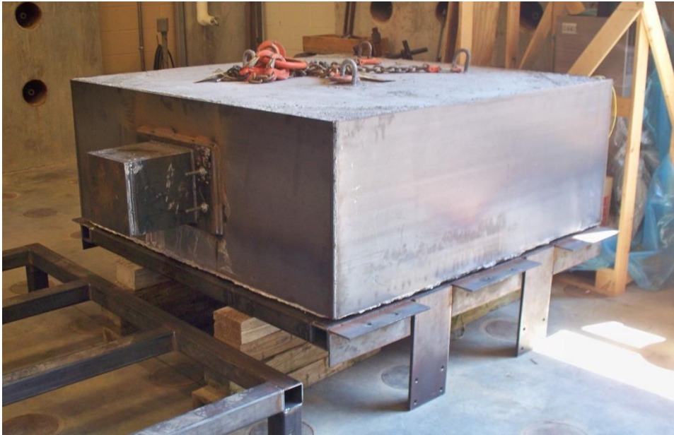
Figure 7. Finished concrete block with impactor.
