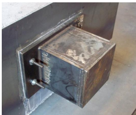
Figure 9. Impactor attached to the imbed plate.
