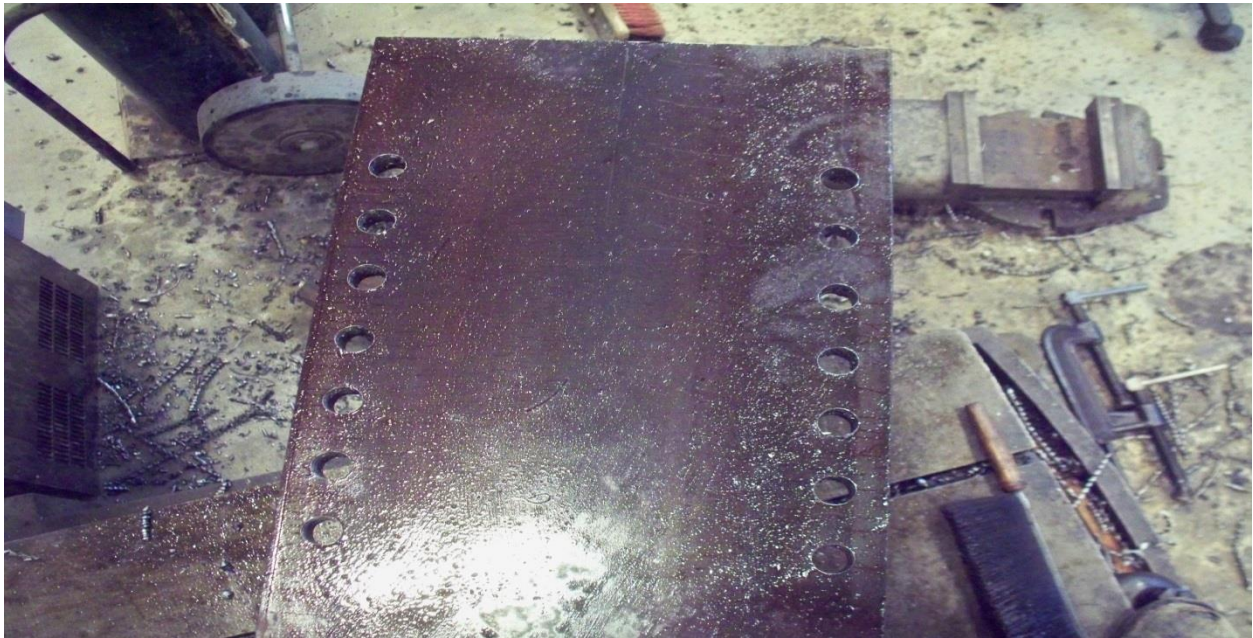
Figure 27. Vertical beams with predrilled holes at 2" spacing.
