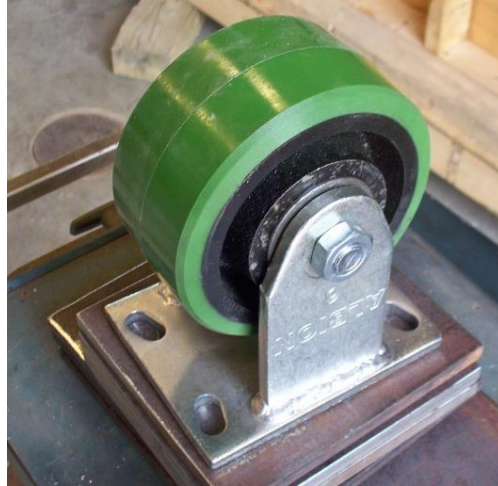
Figure 5. Example of main bearing caster.
