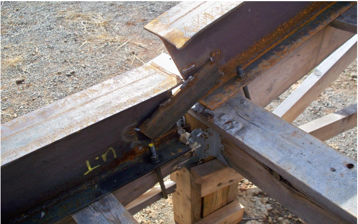
Figure 34. Damage to rails after testing.
