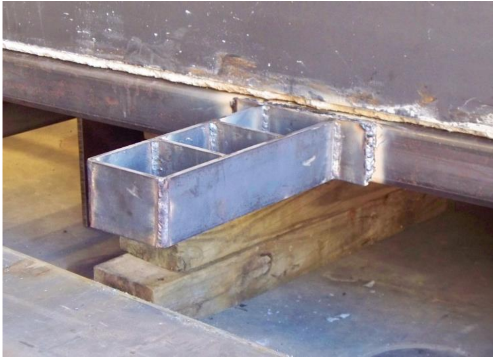
Figure 4. Pull hitch attached to cart frame.
