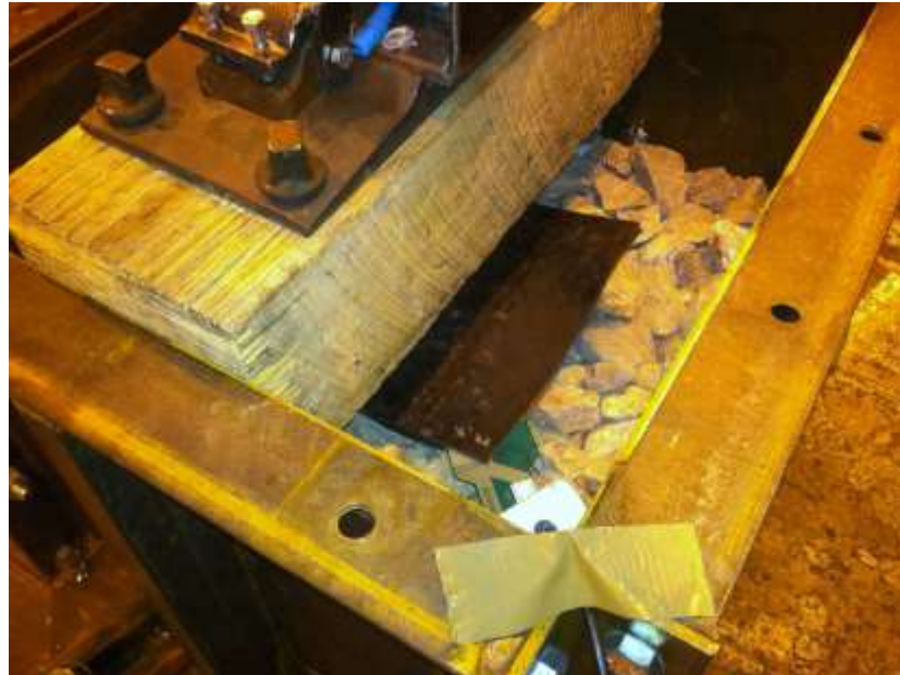
Figure 5.5 Detail of MBTSS sensor/protection location
