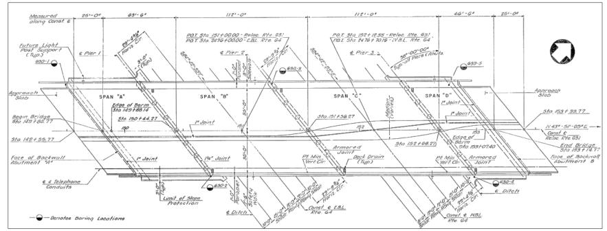
Figure 3. Plan View of 5th Street Extended Bridge
