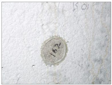
Figure 29. Metallized Reinforced Concrete Surface of I-95 Bridge Substructure Where Test Dolly Was Removed. The removal of the dolly was part of an adhesion test to evaluate the bond between the metallized layer and the concrete substrate.
