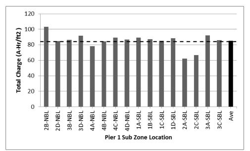
Figure 40. Total Charge Passed During ECE Treatment on Pier 1 Under I-95 Bridge Over Overbrook Road. Sub-zones that did not meet the criteria for charge did meet the chloride level requirement. ECE = electrochemical chloride extraction.
