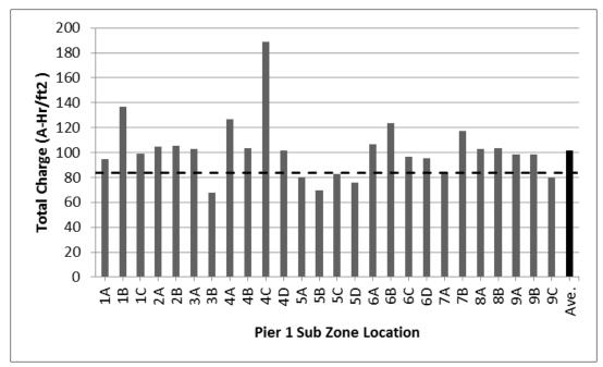
Figure 23. Total Charge Passed During ECE Treatment on Pier 1 of I-95 Bridge Over Hermitage Road. Sub-zones that did not meet the criteria for charge did meet the chloride level requirement. ECE = electrochemical chloride extraction.
