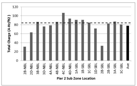
Figure 41. Total Charge Passed During ECE Treatment on Pier 2 Under I-95 Bridge Over Overbrook Road. Sub-zones that did not meet the criteria for charge did meet the chloride level requirement. ECE = electrochemical chloride extraction.
