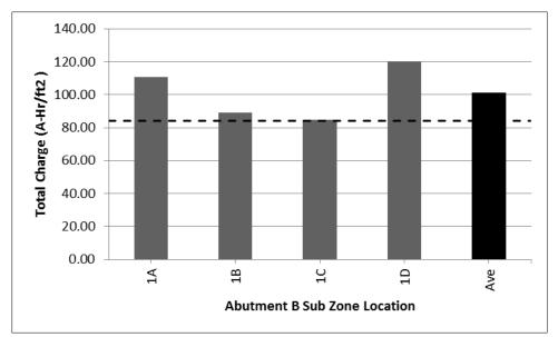
Figure 42. Total Charge Passed During ECE Treatment on Abutment B Under I-95 Bridge Over Overbrook Road. ECE = electrochemical chloride extraction.
