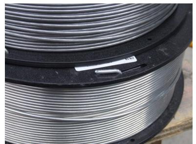
Figure 27. Al-Zn-In Anode Wire on Spool. This wire will be fed through a specially designed gun that will result in the molten metal striking and adhering to the surface being coated.
