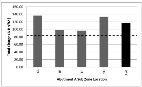
Figure 39. Total Charge Passed During ECE Treatment on Abutment A Under I-95 Bridge Over Overbrook Road. ECE = electrochemical chloride extraction.
