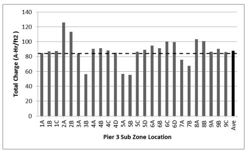
Figure 25. Total Charge Passed During ECE Treatment in Selected Sub-zone Areas on Pier 3 of I-95 Bridge Over Hermitage Road. A partial data set was made available by the contractor. Sub-zones that did not meet the criteria for charge did meet the chloride level requirement. ECE = electrochemical chloride extraction.
