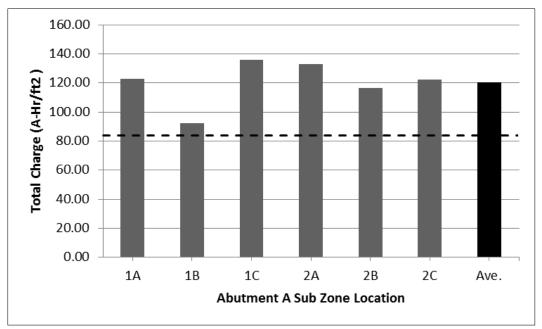
Figure 22. Total Charge Passed During ECE Treatment on Abutment A of I-95 Bridge Over Hermitage Road. ECE = electrochemical chloride extraction.
