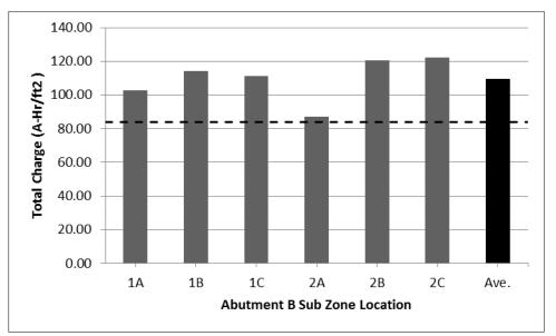
Figure 26. Total Charge Passed During ECE Treatment on Abutment B of I-95 Bridge Over Hermitage Road. ECE = electrochemical chloride extraction.
