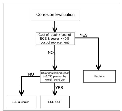
Figure 19. Repair Method Proposed by Corrosion Services Consultant for the Eleven I-95 Bridges in Richmond, Virginia
