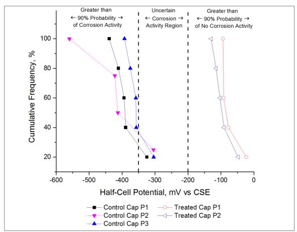
Figure 17. Half-cell Potential Measurements for Treated and Untreated Pier Cap Ends of 5th Street Extended Bridge
