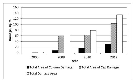
Figure 8. Column and Cap Reported Concrete Damage With Time for 5th Street Extended Bridge
