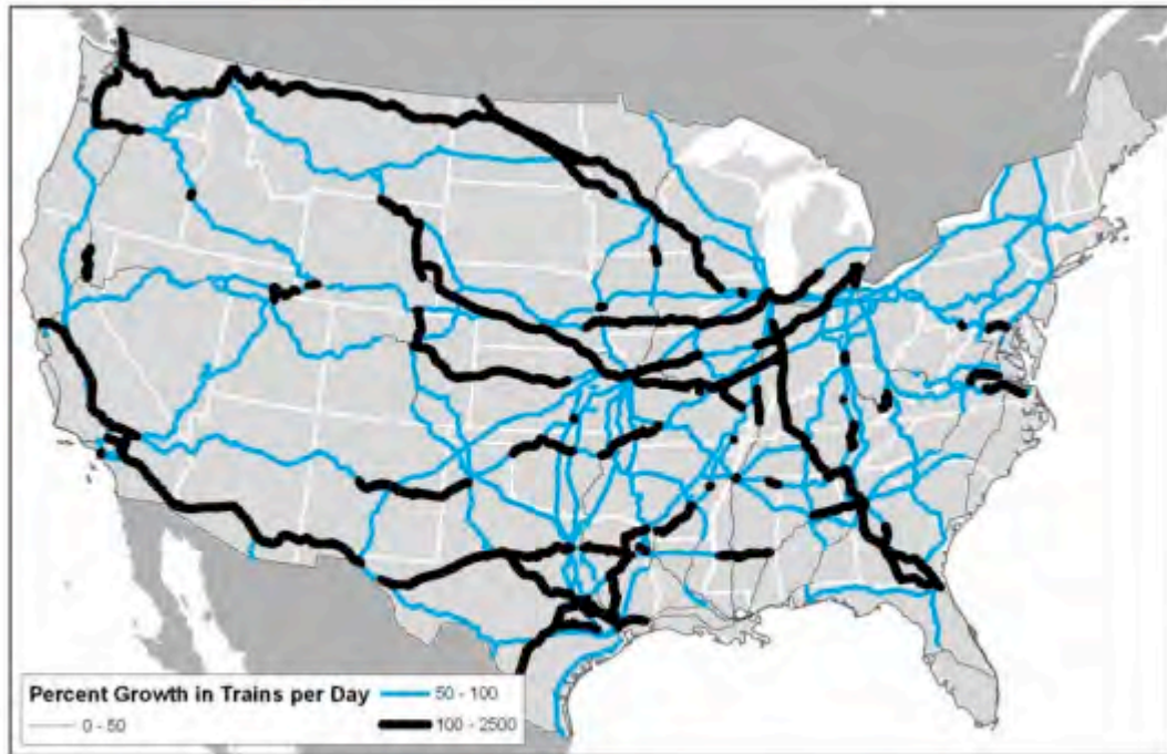
Figure 1-2: Percentage growth in trains per day from 2005 to 2035 by Primary Rail Corridor Source: Cambridge Systematics
